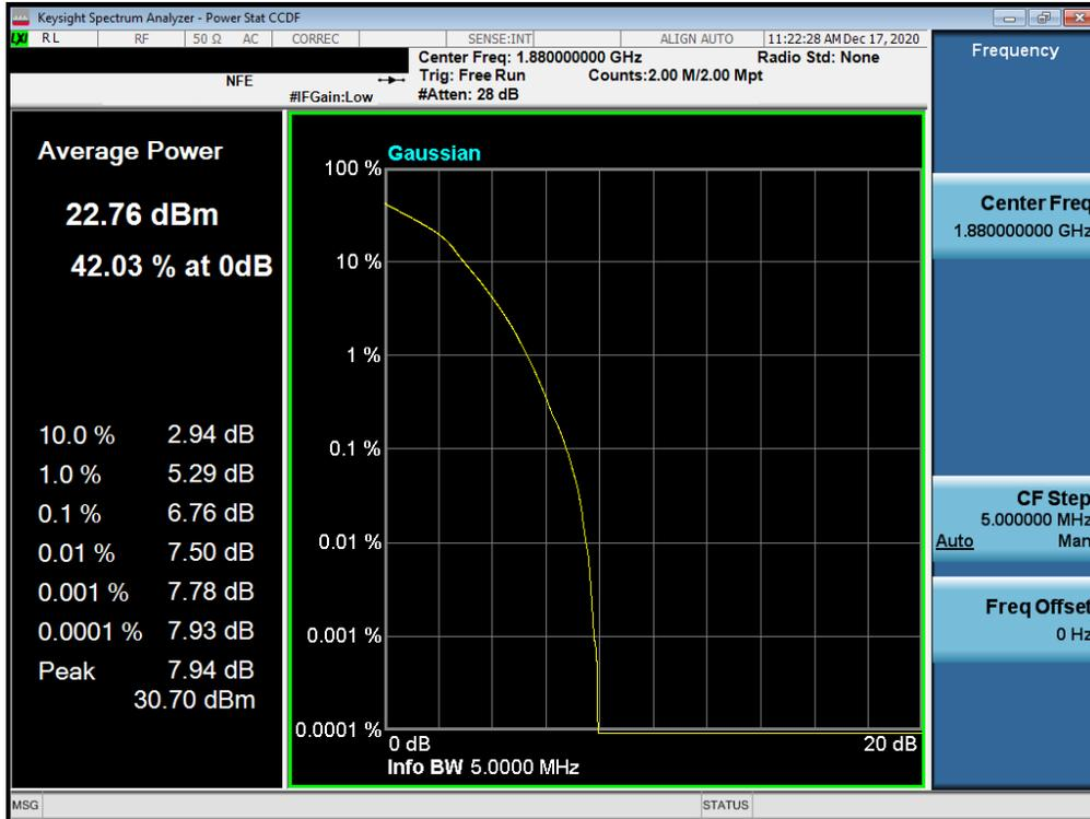
Plot 7-115. PAR Plot (LTE Band 25/2 - 5MHz 16-QAM - Full RB Configuration)
