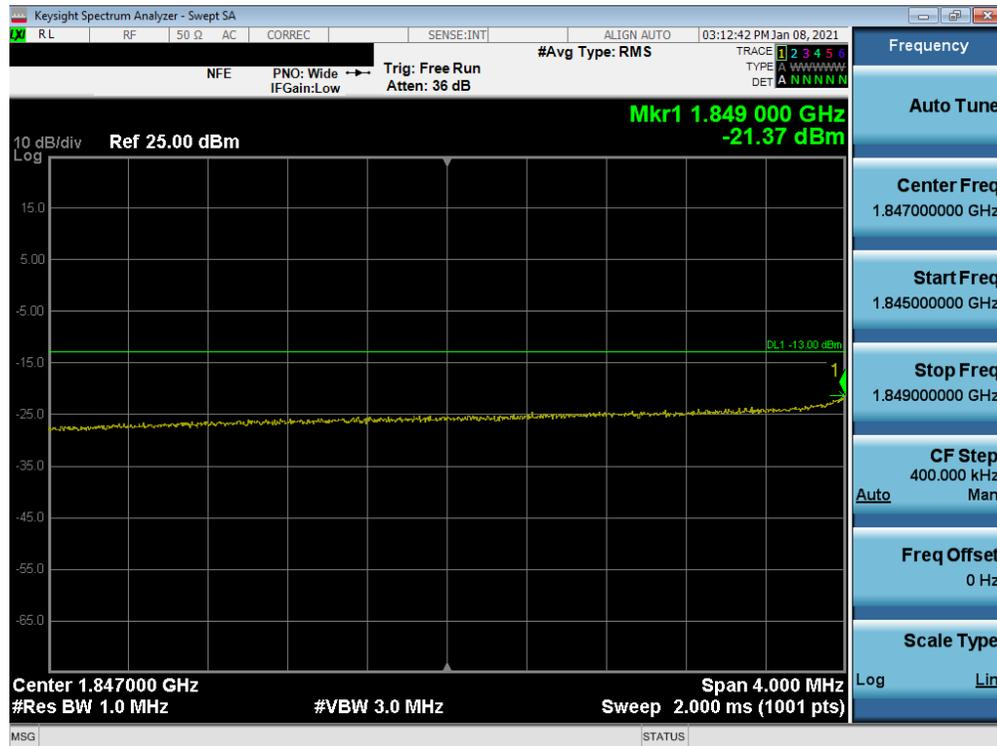
Plot 7-72. Extended Lower Band Edge Plot (LTE Band 25/2 - 10MHz QPSK – Full RB Configuration)
