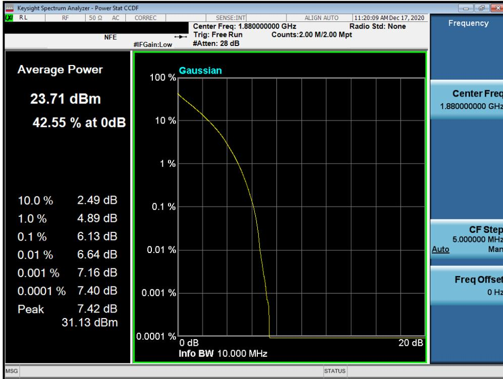
Plot 7-111. PAR Plot (LTE Band 25/2 - 10MHz QPSK - Full RB Configuration)
