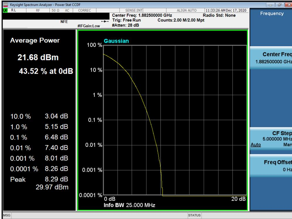
Plot 7-107. PAR Plot (LTE Band 25/2 - 20MHz 64-QAM - Full RB Configuration)
