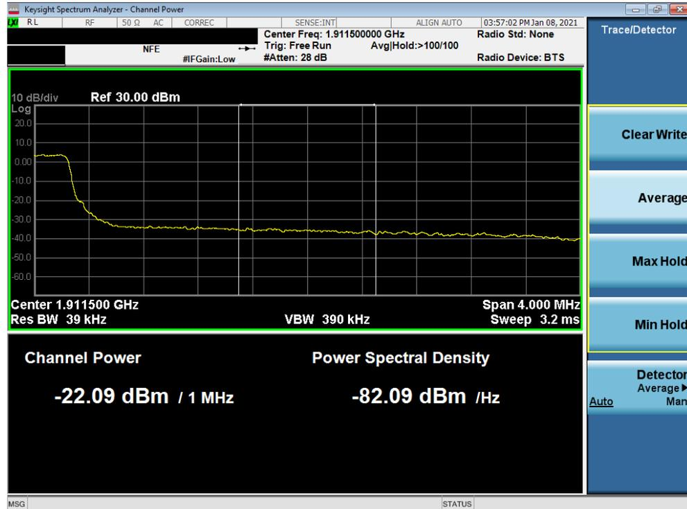
Plot 7-80. Extended Upper Band Edge Plot (LTE Band 2 - 5MHz QPSK – Full RB Configuration)
