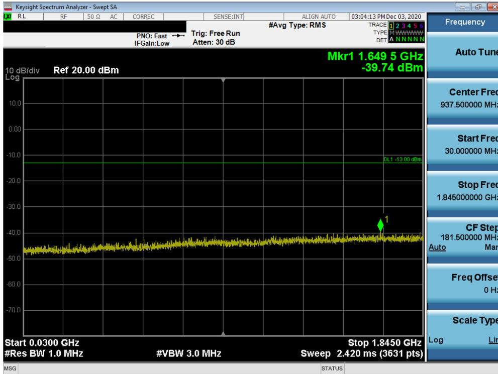
**Plot 7-32. Conducted Spurious Plot (GPRS Ch. 512)**
