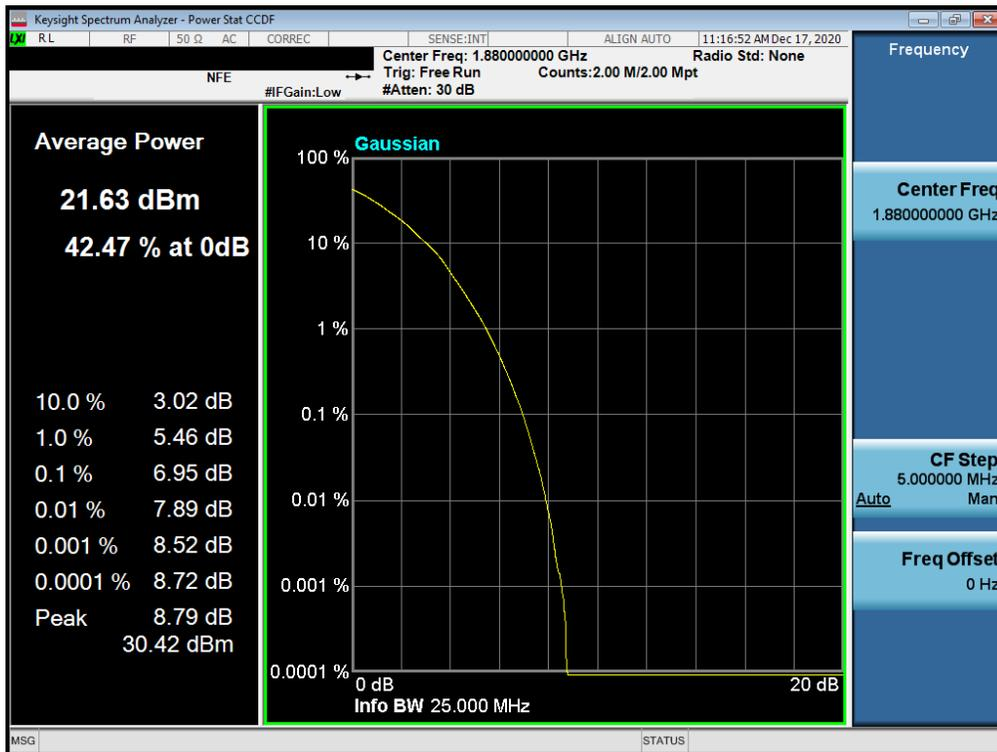
Plot 7-110. PAR Plot (LTE Band 25/2 - 15MHz 64-QAM - Full RB Configuration)
