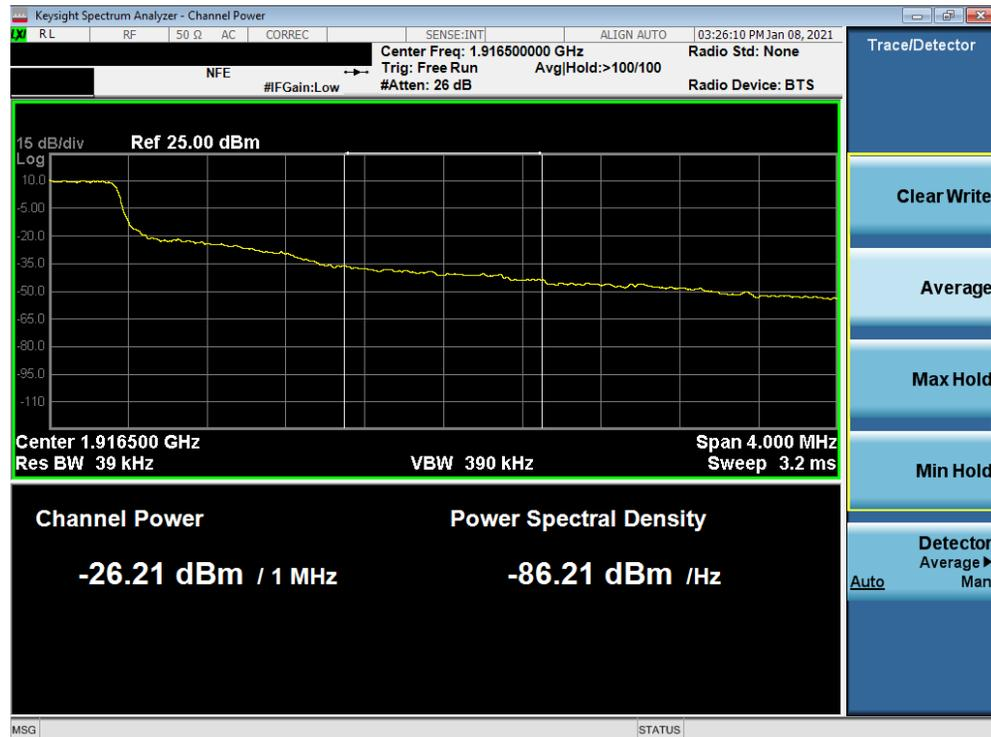
Plot 7-94. Extended Upper Band Edge Plot (LTE Band 25 – 1.4MHz QPSK – Full RB Configuration)
