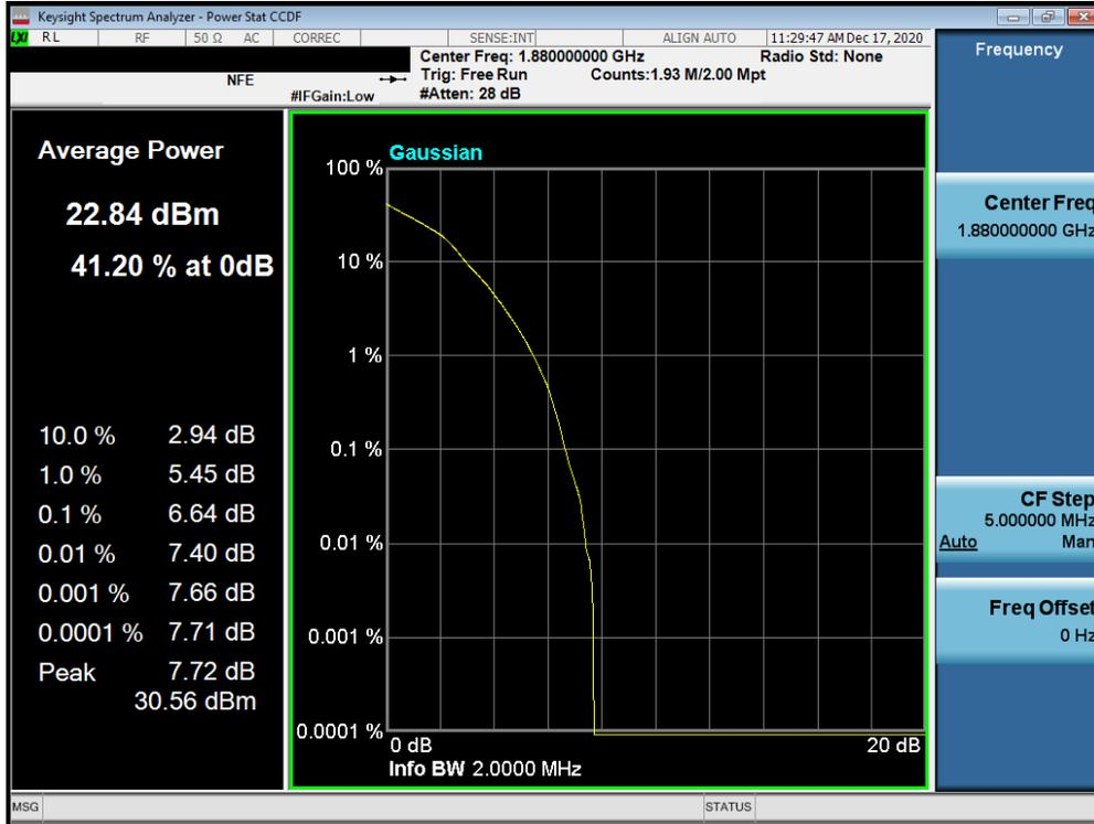
Plot 7-121. PAR Plot (LTE Band 25/2 - 1.4MHz 16-QAM - Full RB Configuration)
