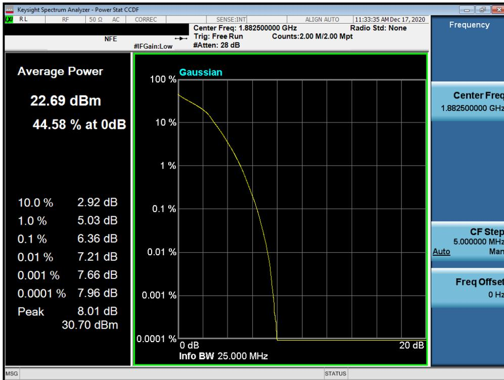
**Plot 7-106. PAR Plot (LTE Band 25/2 - 20MHz 16-QAM - Full RB Configuration)**
