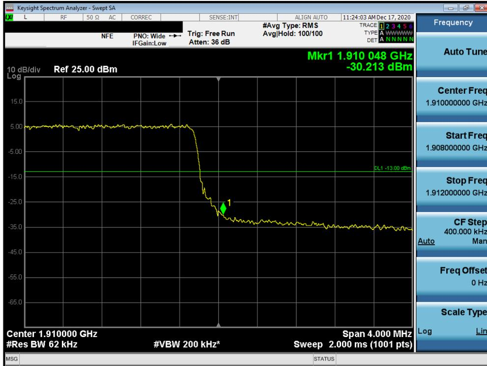
Plot 7-79. Upper Band Edge Plot (LTE Band 2 - 5MHz QPSK – Full RB Configuration)
