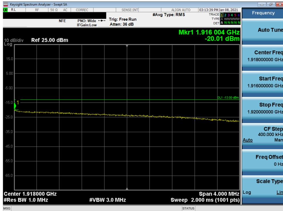
Plot 7-76. Extended Upper Band Edge Plot (LTE Band 25 - 10MHz QPSK – Full RB Configuration)
