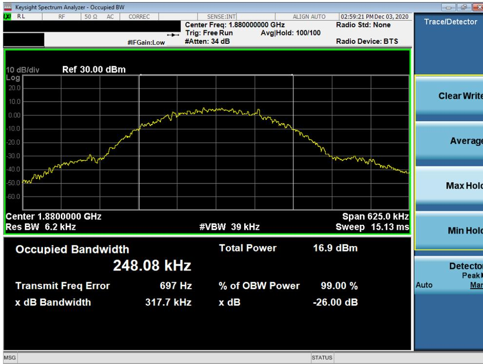
Plot 7-19. Occupied Bandwidth Plot (GPRS, Ch. 661)
