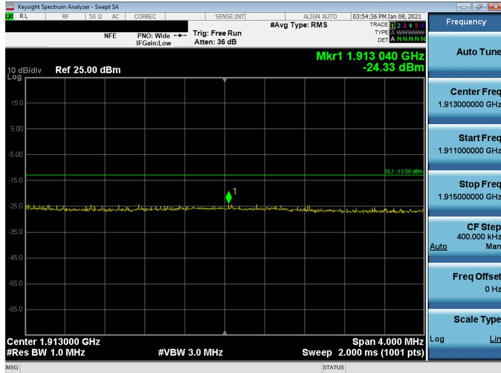
Plot 7-68. Extended Upper Band Edge Plot (LTE Band 2 - 15MHz QPSK – Full RB Configuration)
