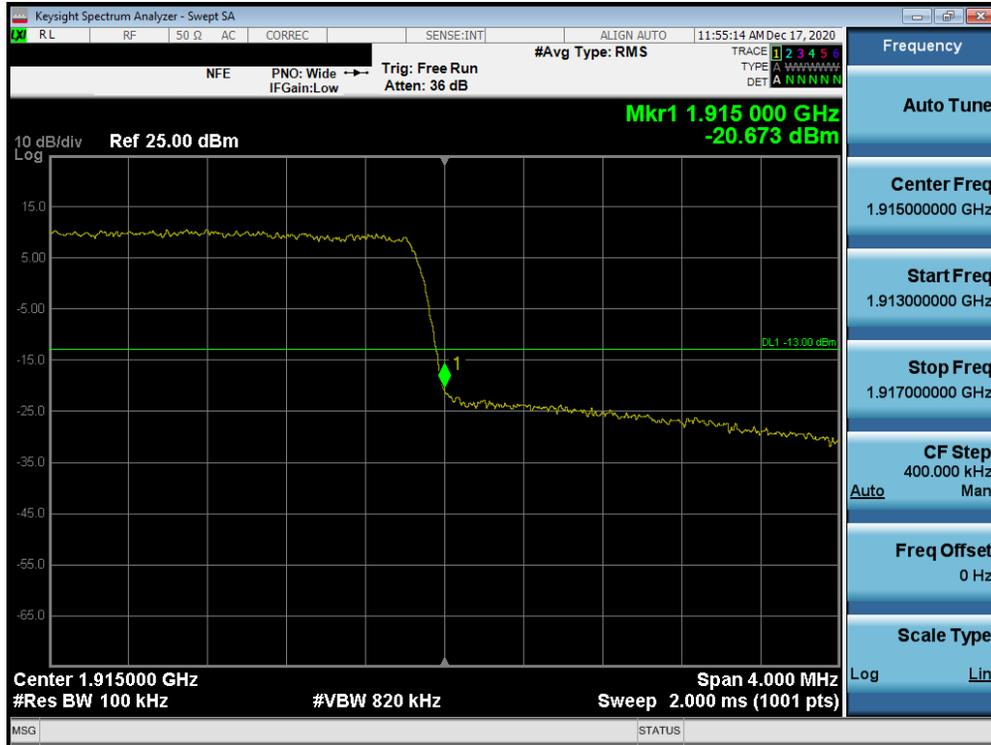
Plot 7-87. Upper Band Edge Plot (LTE Band 25 - 3MHz QPSK – Full RB Configuration)
