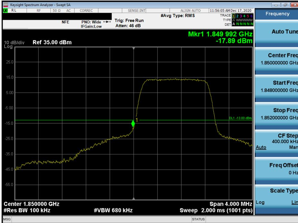
Plot 7-89. Lower Band Edge Plot (LTE Band 25/2 – 1.4MHz QPSK – Full RB Configuration)
