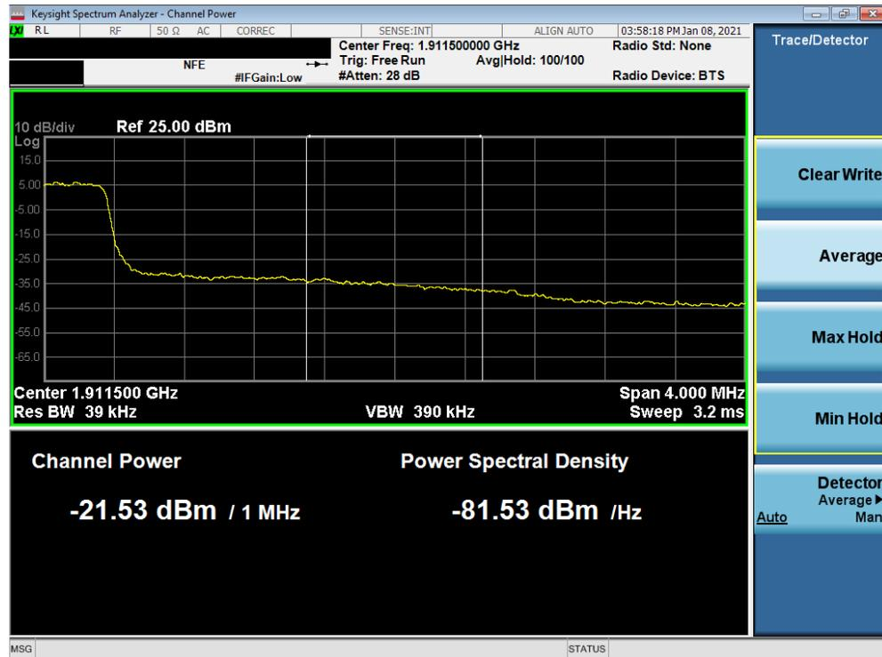
Plot 7-86. Extended Upper Band Edge Plot (LTE Band 2 - 3MHz QPSK – Full RB Configuration)
