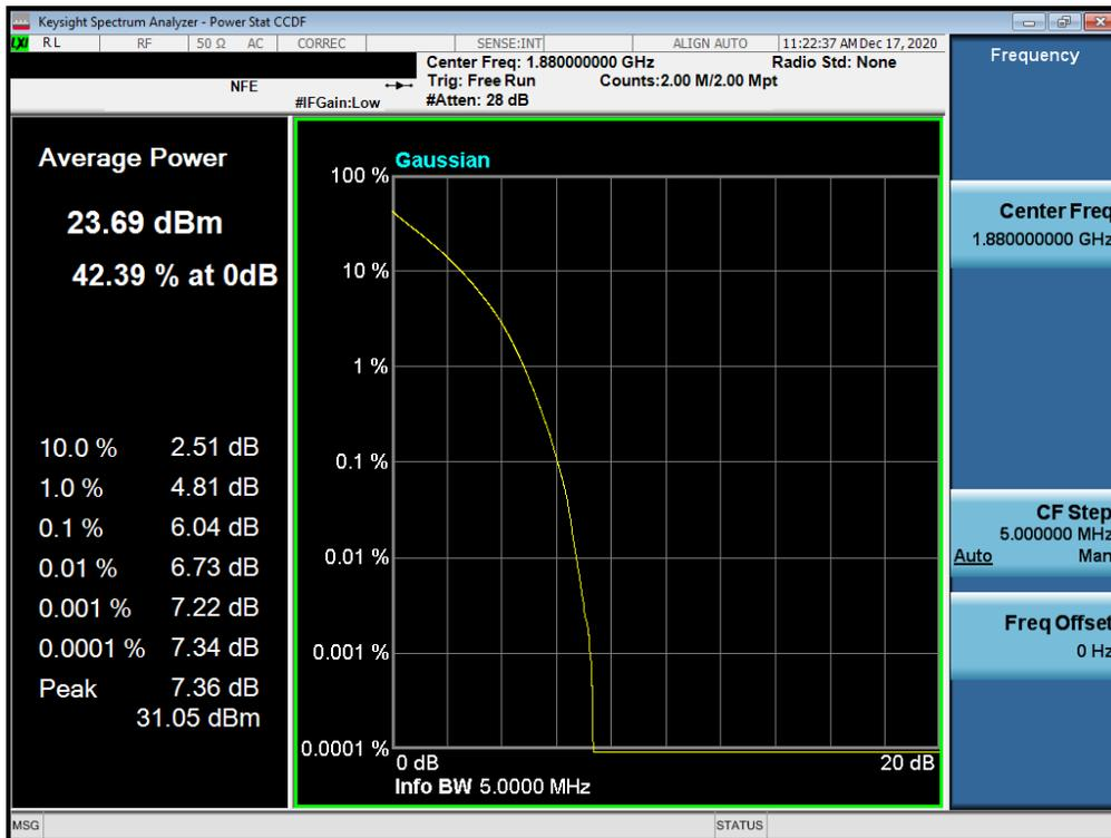
Plot 7-114. PAR Plot (LTE Band 25/2 - 5MHz QPSK - Full RB Configuration)
