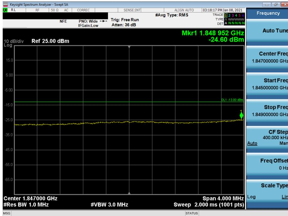
Plot 7-66. Extended Lower Band Edge Plot (LTE Band 25/2 - 15MHz QPSK – Full RB Configuration)
