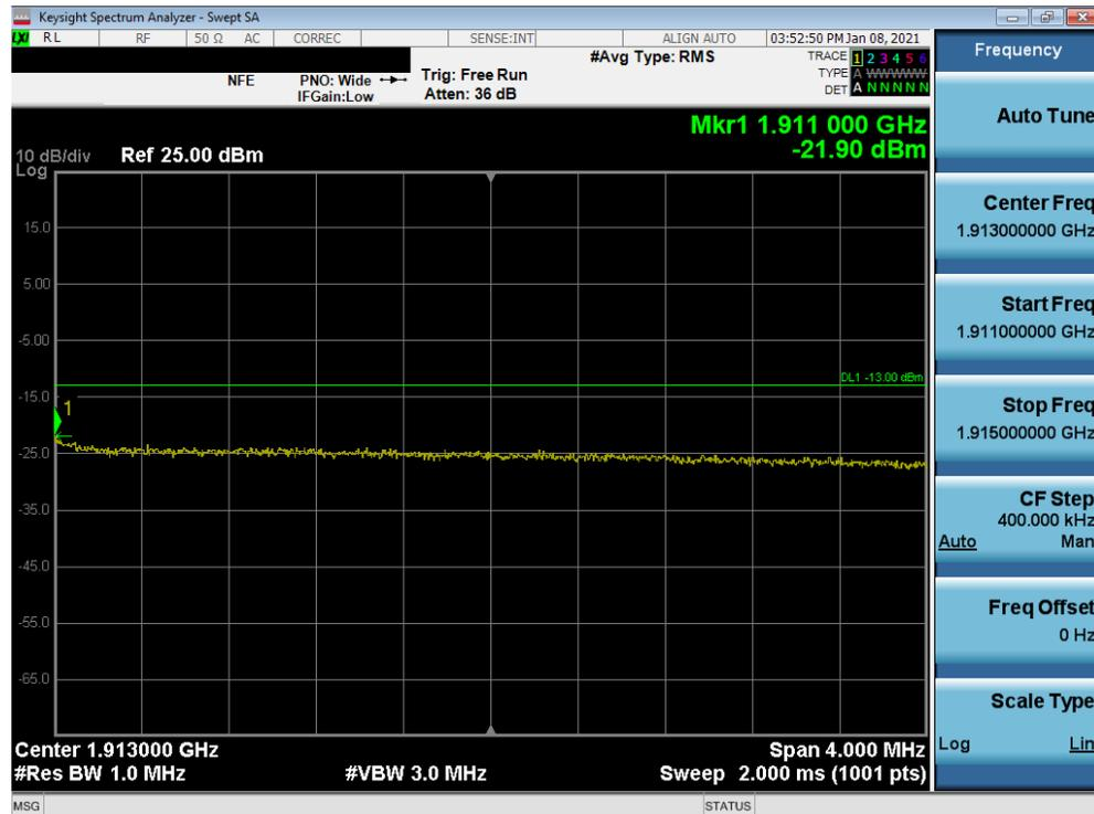
Plot 7-74. Extended Upper Band Edge Plot (LTE Band 2 - 10MHz QPSK – Full RB Configuration)
