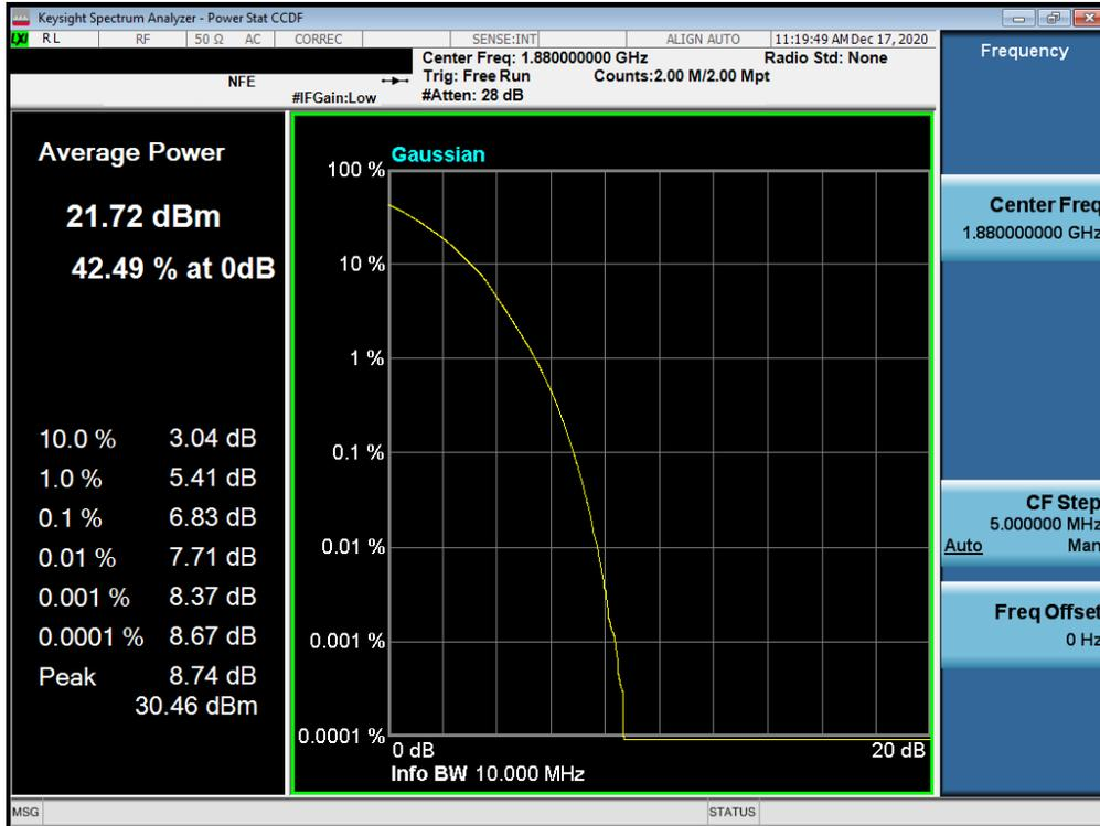
Plot 7-113. PAR Plot (LTE Band 25/2 - 10MHz 64-QAM - Full RB Configuration)
