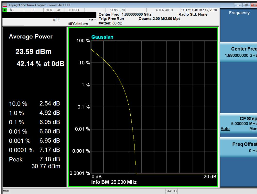
Plot 7-108. PAR Plot (LTE Band 25/2 - 15MHz QPSK - Full RB Configuration)
