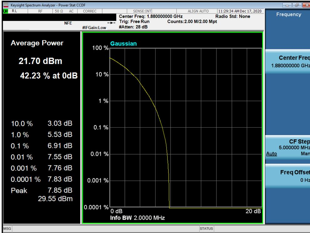
Plot 7-122. PAR Plot (LTE Band 25/2 - 1.4MHz 64-QAM - Full RB Configuration)
