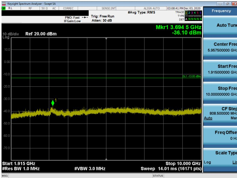
Plot 7-39. Conducted Spurious Plot (GPRS Ch. 810)
