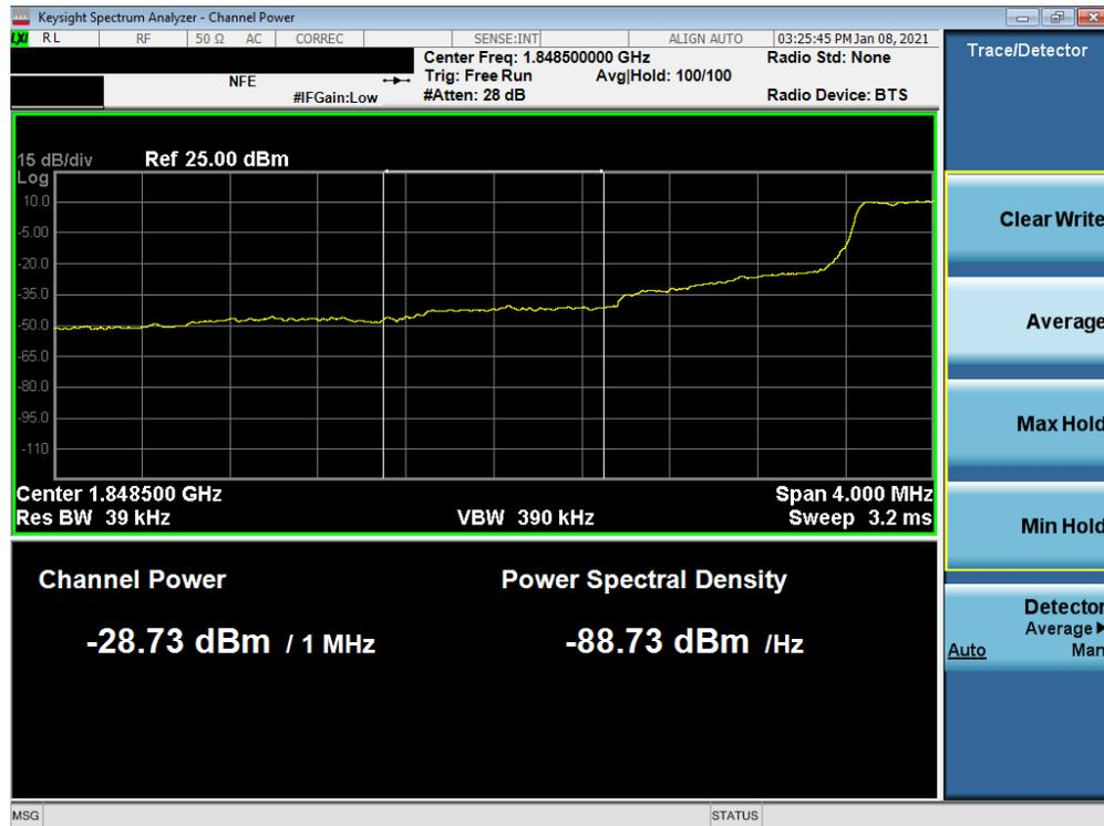
Plot 7-90. Extended Lower Band Edge Plot (LTE Band 25/2 – 1.4MHz QPSK – Full RB Configuration)
