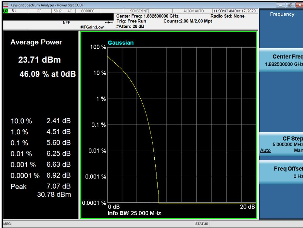
**Plot 7-105. PAR Plot (LTE Band 25/2 - 20MHz QPSK - Full RB Configuration)**
