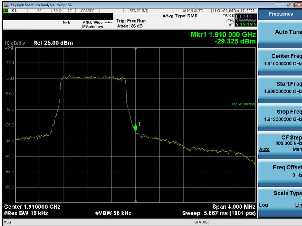
Plot 7-91. Upper Band Edge Plot (LTE Band 2 – 1.4MHz QPSK – Full RB Configuration)
