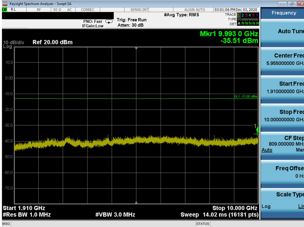
Plot 7-36. Conducted Spurious Plot (GPRS Ch. 661)
