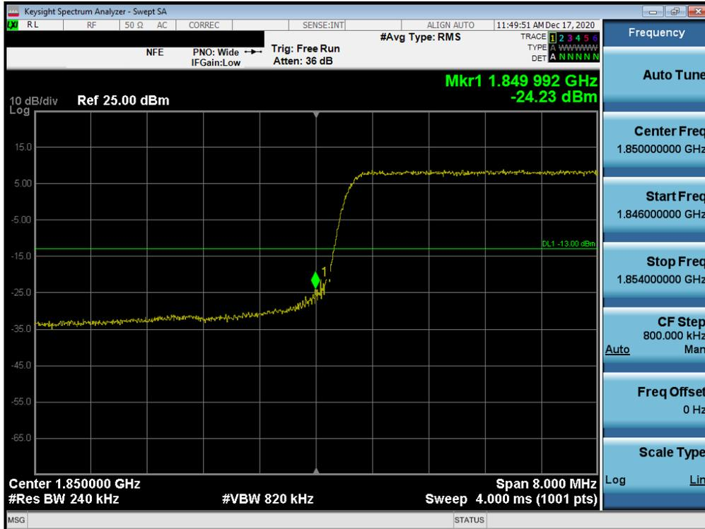
Plot 7-71. Lower Band Edge Plot (LTE Band 25/2 - 10MHz QPSK – Full RB Configuration)
