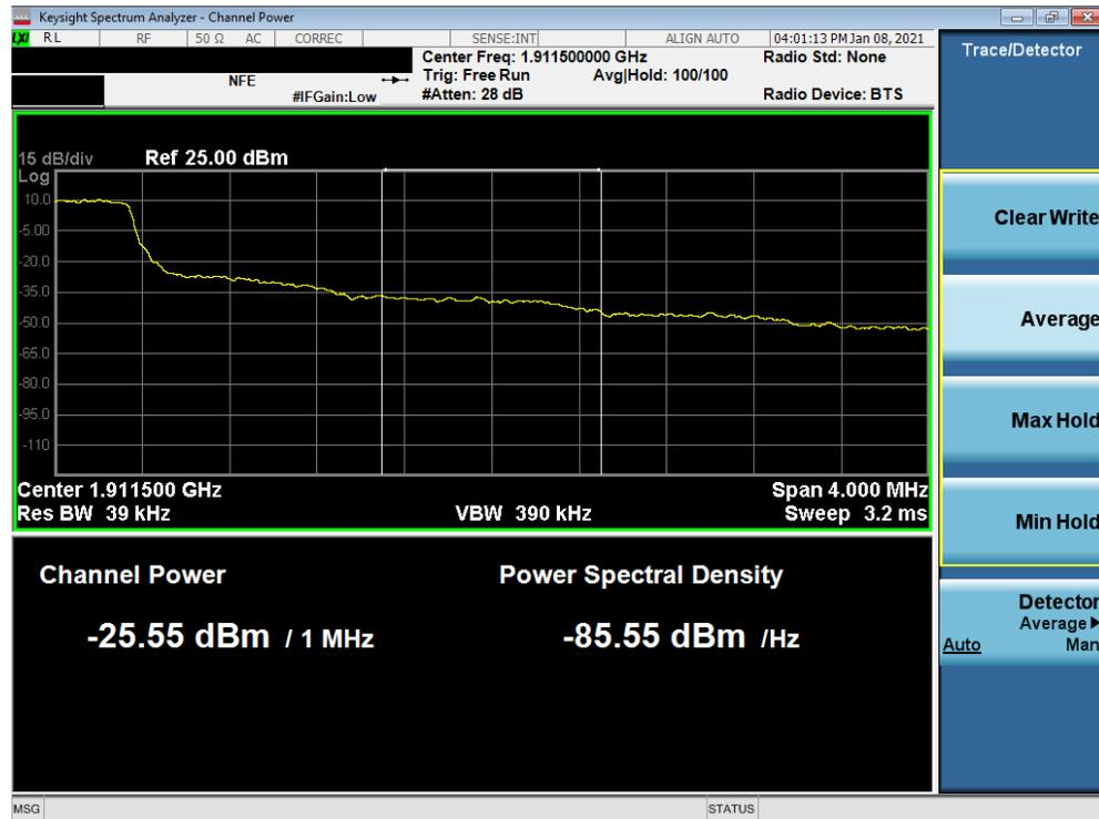
Plot 7-92. Extended Upper Band Edge Plot (LTE Band 2 – 1.4MHz QPSK – Full RB Configuration)
