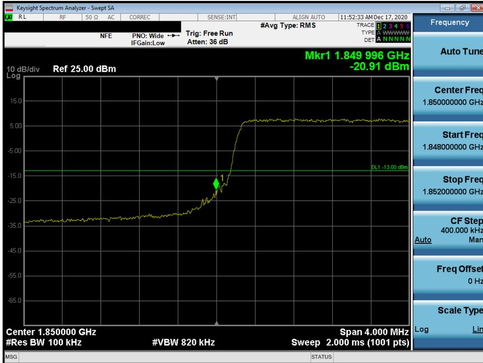
Plot 7-77. Lower Band Edge Plot (LTE Band 25/2 - 5MHz QPSK – Full RB Configuration)
