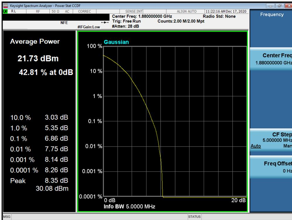
Plot 7-116. PAR Plot (LTE Band 25/2 - 5MHz 64-QAM - Full RB Configuration)
