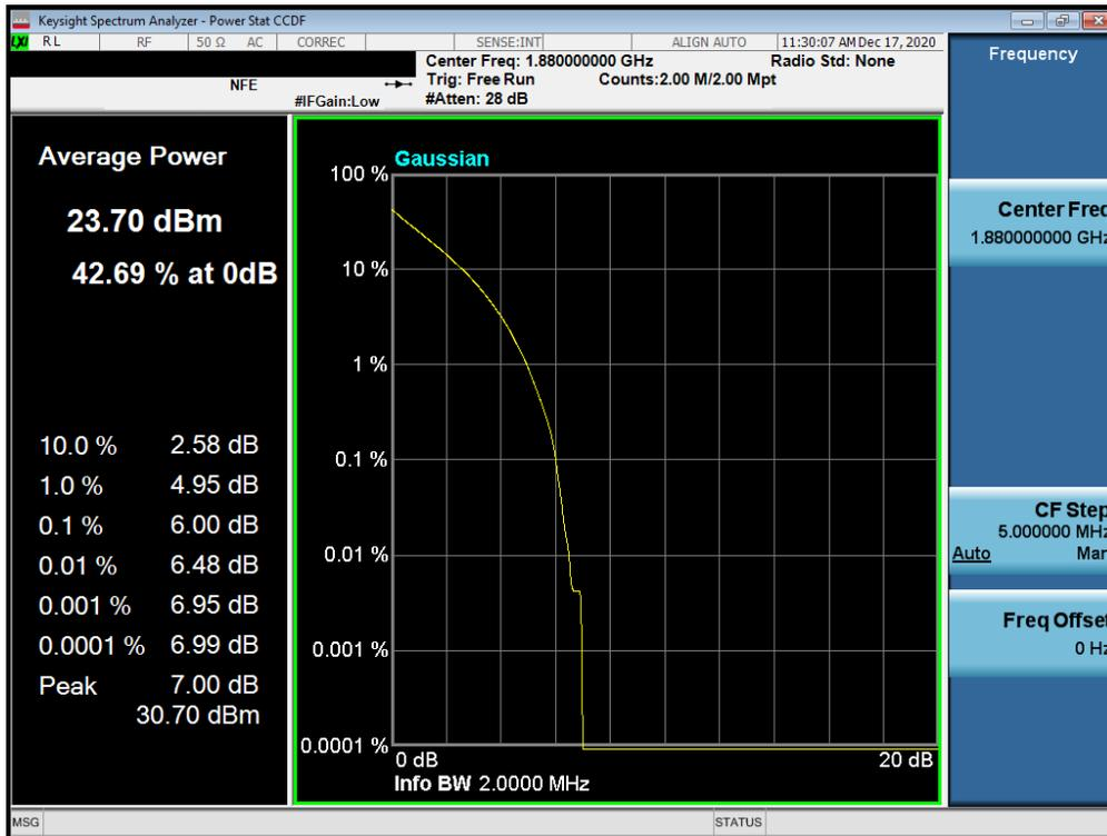
Plot 7-120. PAR Plot (LTE Band 25/2 - 1.4MHz QPSK - Full RB Configuration)
