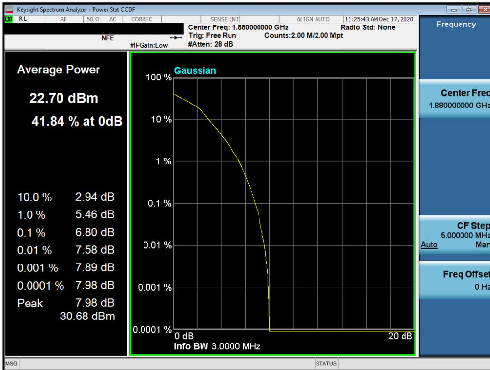
Plot 7-118. PAR Plot (LTE Band 25/2 - 3MHz 16-QAM - Full RB Configuration)
