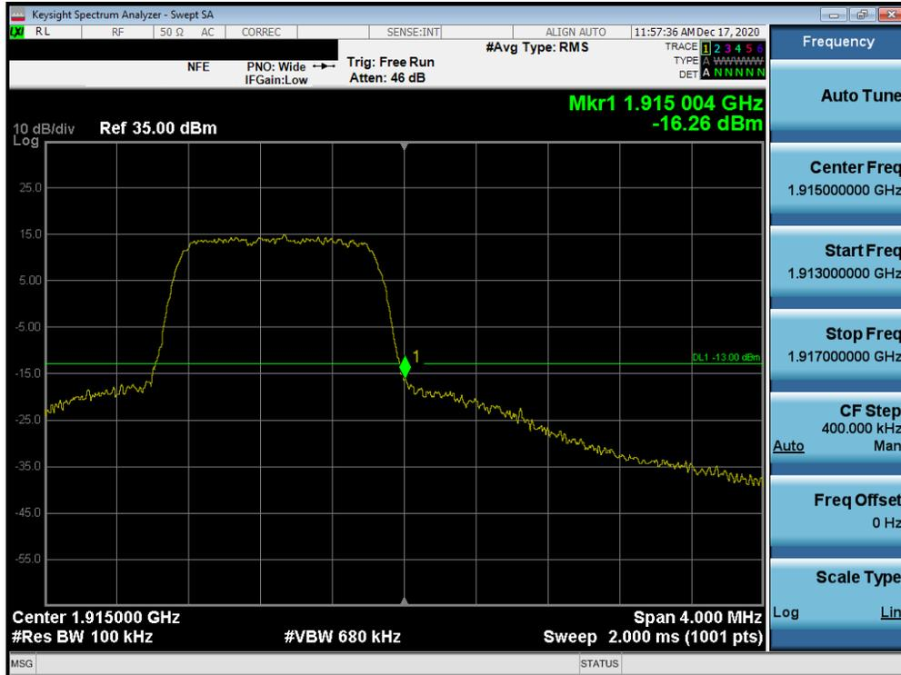
Plot 7-93. Upper Band Edge Plot (LTE Band 25 – 1.4MHz QPSK – Full RB Configuration)
