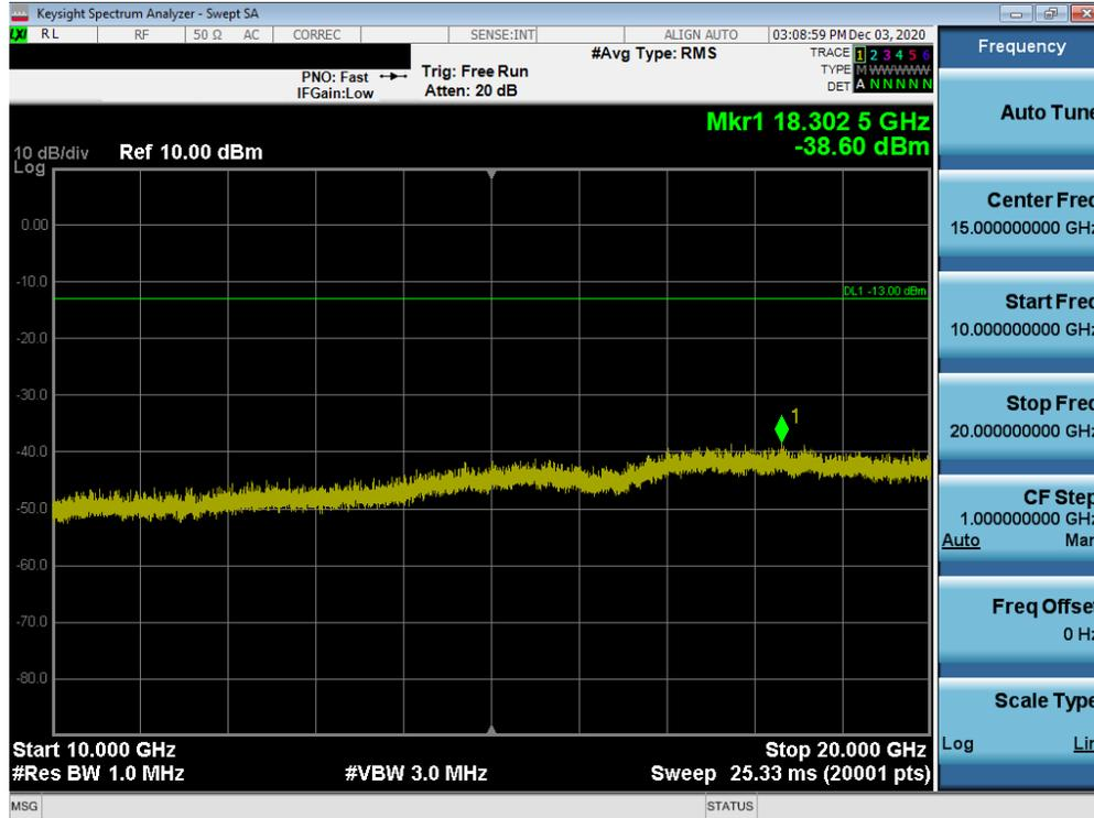
Plot 7-40. Conducted Spurious Plot (GPRS Ch. 810)
