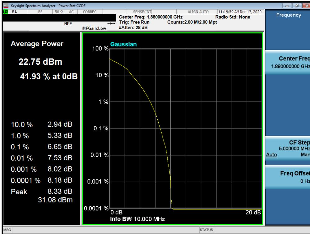
Plot 7-112. PAR Plot (LTE Band 25/2 - 10MHz 16-QAM - Full RB Configuration)
