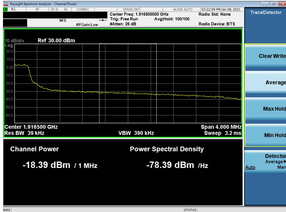
Plot 7-82. Extended Upper Band Edge Plot (LTE Band 25 - 5MHz QPSK – Full RB Configuration)
