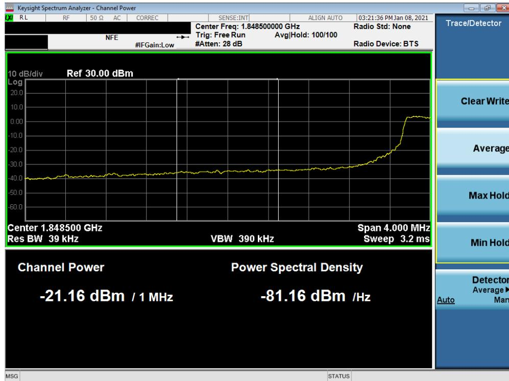
Plot 7-78. Extended Lower Band Edge Plot (LTE Band 25/2 - 5MHz QPSK – Full RB Configuration)
