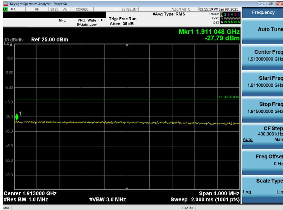
Plot 7-62. Extended Upper Band Edge Plot (LTE Band 2 - 20MHz QPSK – Full RB Configuration)
