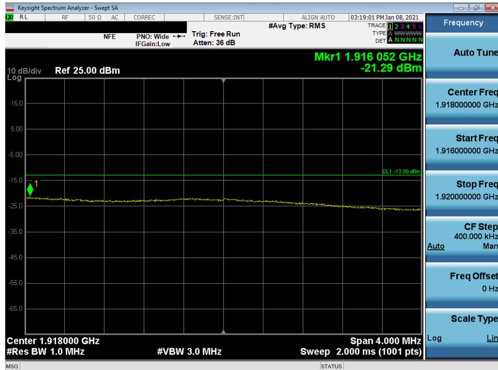
Plot 7-70. Extended Upper Band Edge Plot (LTE Band 25 - 15MHz QPSK – Full RB Configuration)
