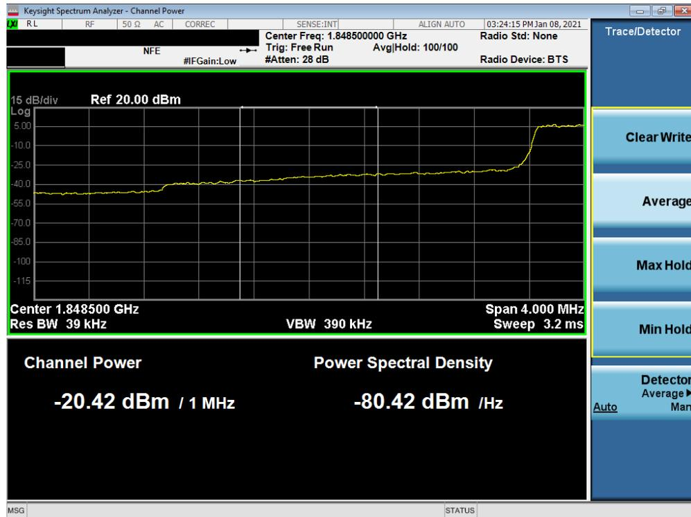
Plot 7-84. Extended Lower Band Edge Plot (LTE Band 25/2 - 3MHz QPSK – Full RB Configuration)
