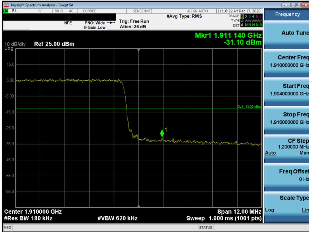
Plot 7-67. Upper Band Edge Plot (LTE Band 2 - 15MHz QPSK – Full RB Configuration)
