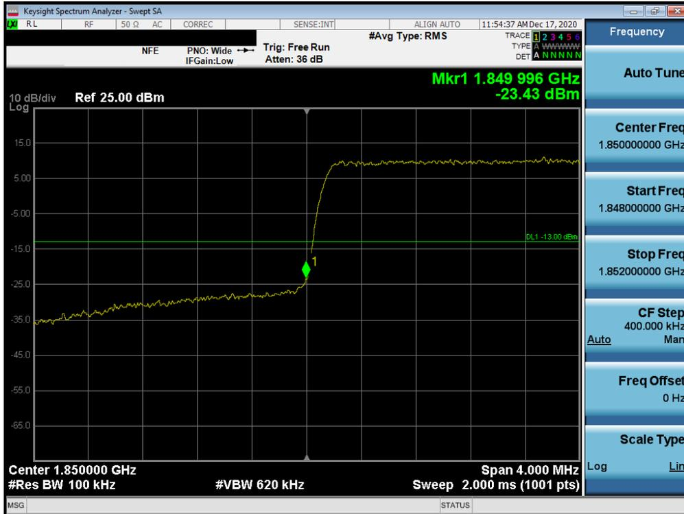
Plot 7-83. Lower Band Edge Plot (LTE Band 25/2 - 3MHz QPSK – Full RB Configuration)
