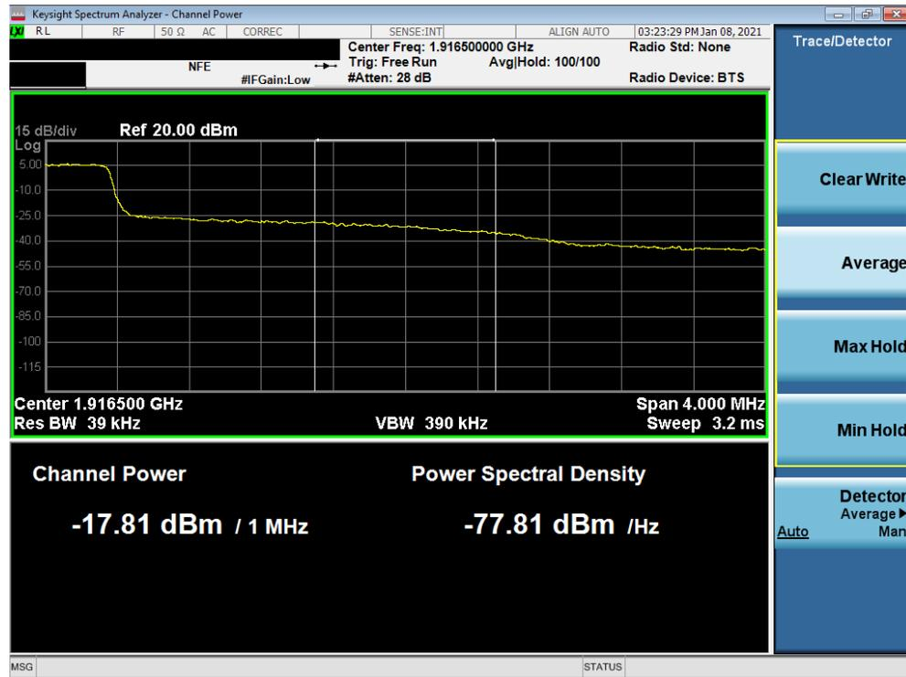
Plot 7-88. Extended Upper Band Edge Plot (LTE Band 25 - 3MHz QPSK – Full RB Configuration)
