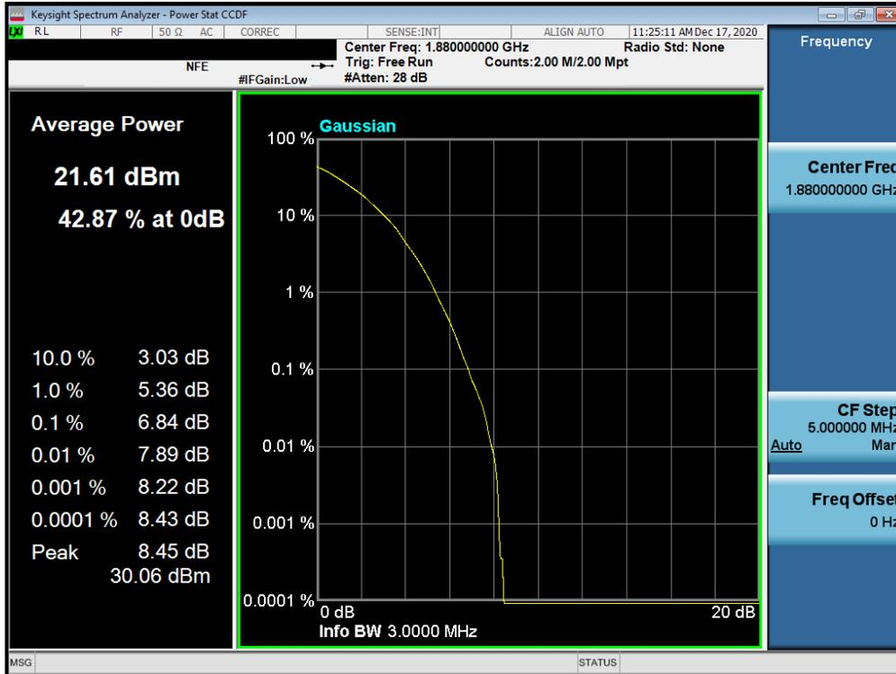
Plot 7-119. PAR Plot (LTE Band 25/2 - 3MHz 64-QAM - Full RB Configuration)
