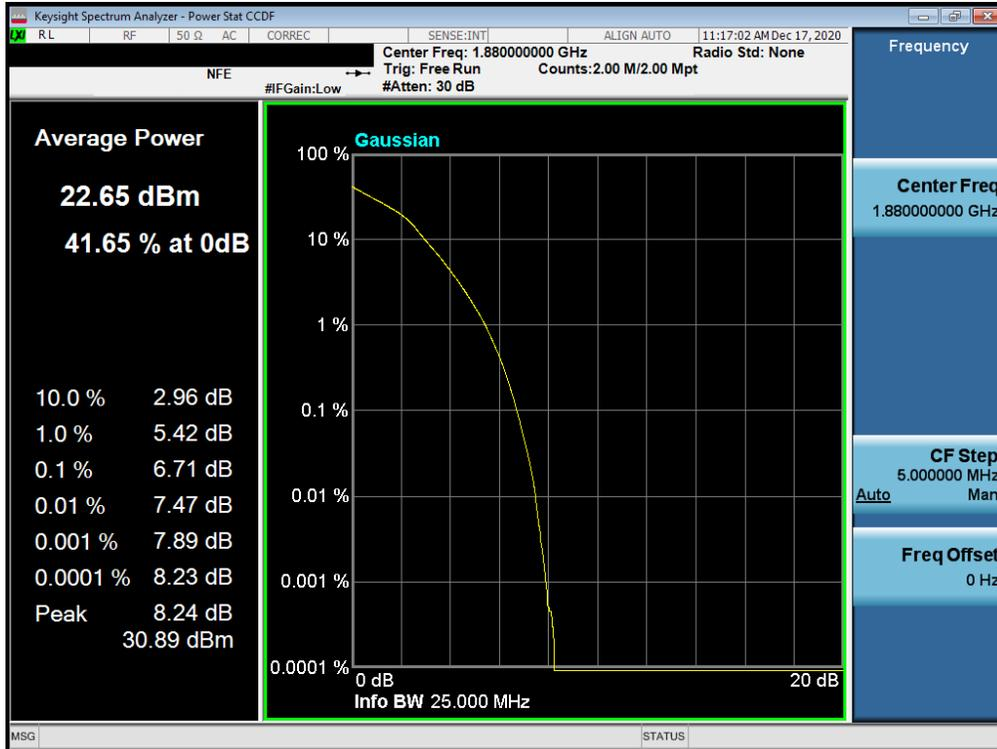
Plot 7-109. PAR Plot (LTE Band 25/2 - 15MHz 16-QAM - Full RB Configuration)
