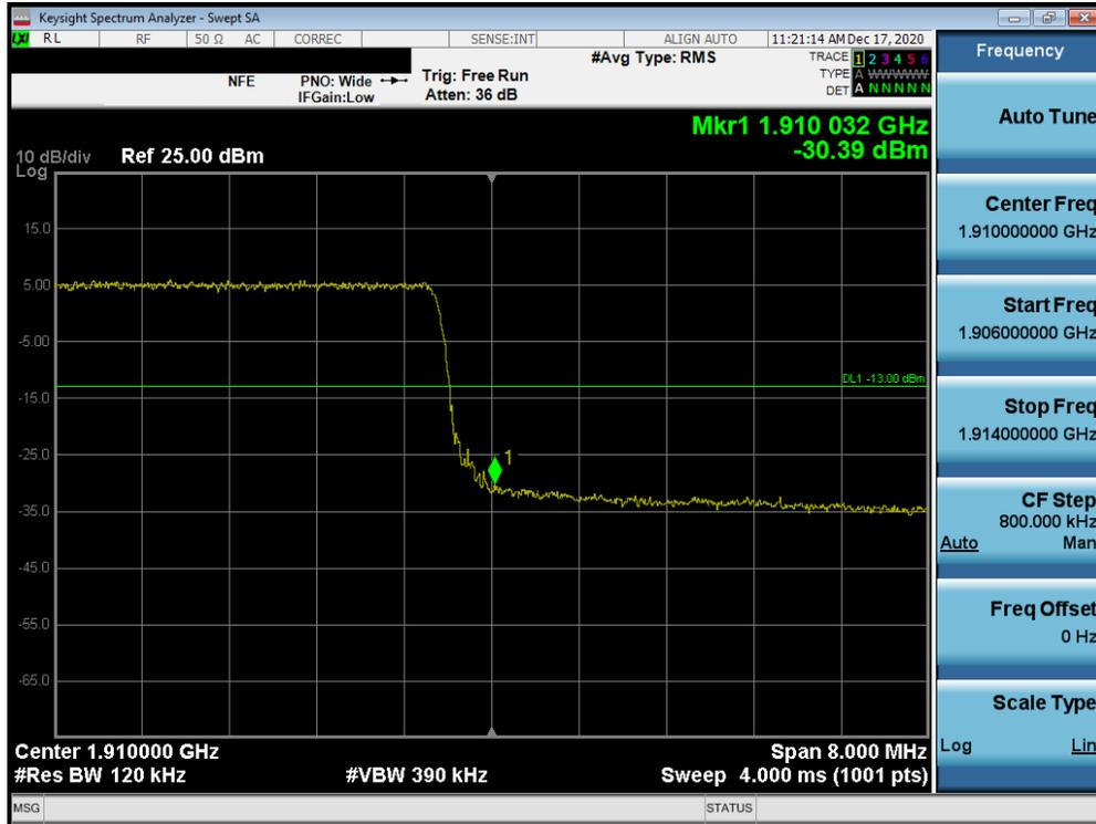
Plot 7-73. Upper Band Edge Plot (LTE Band 2 - 10MHz QPSK – Full RB Configuration)
