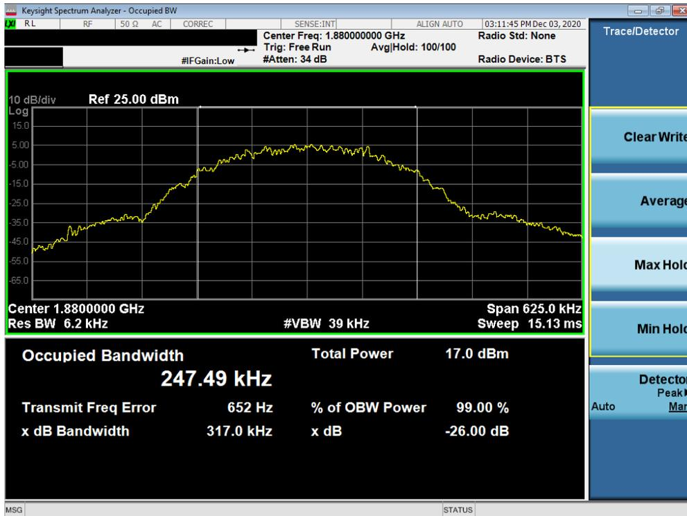
Plot 7-20. Occupied Bandwidth Plot (EDGE, Ch. 661)
