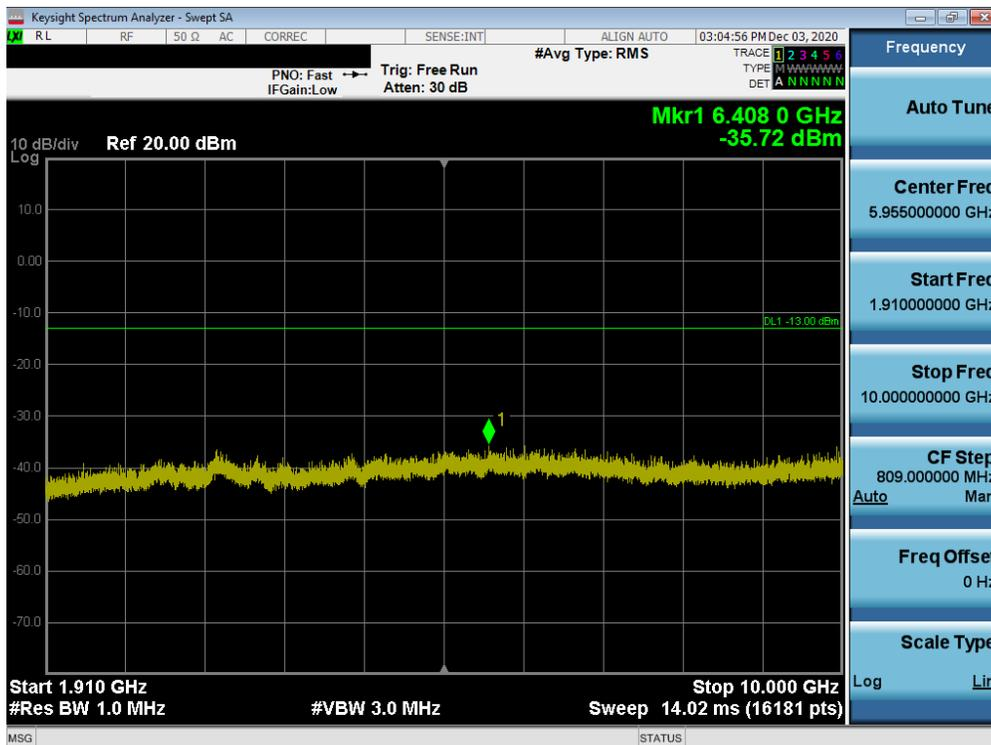
**Plot 7-33. Conducted Spurious Plot (GPRS Ch. 512)**
