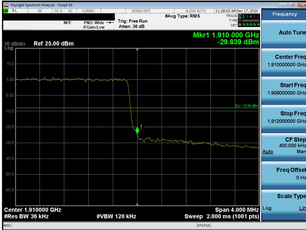
Plot 7-85. Upper Band Edge Plot (LTE Band 2 - 3MHz QPSK – Full RB Configuration)
