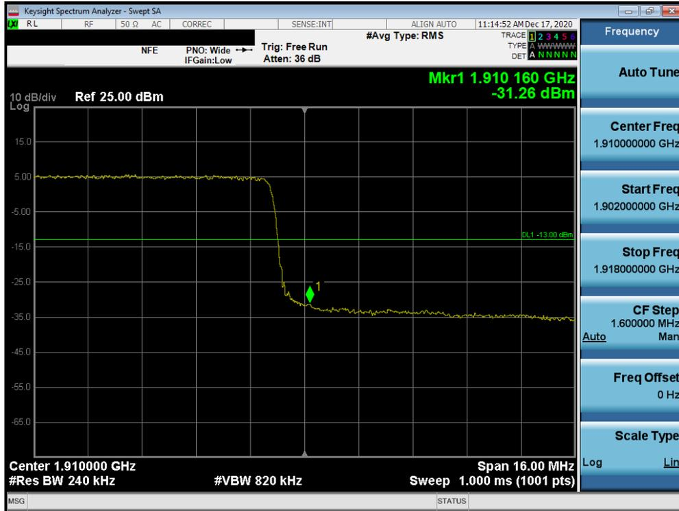
Plot 7-61. Upper Band Edge Plot (LTE Band 2 - 20MHz QPSK – Full RB Configuration)
