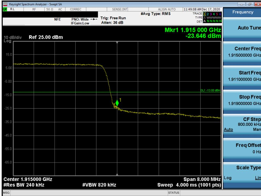
Plot 7-75. Upper Band Edge Plot (LTE Band 25 - 10MHz QPSK – Full RB Configuration)
