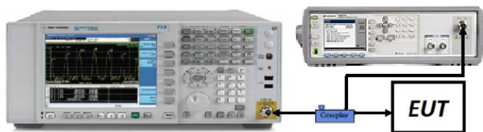
Figure 7-6. Test Instrument & Measurement Setup
