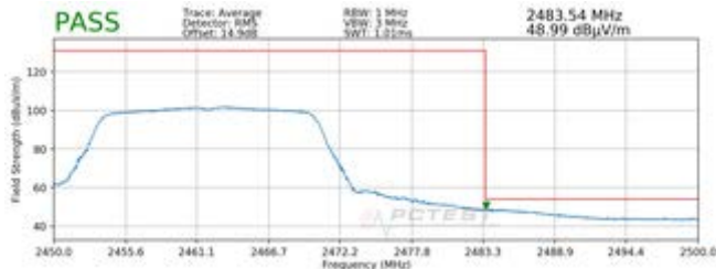
Plot 7-41. Radiated Restricted Upper Band Edge Measurement (Average)
