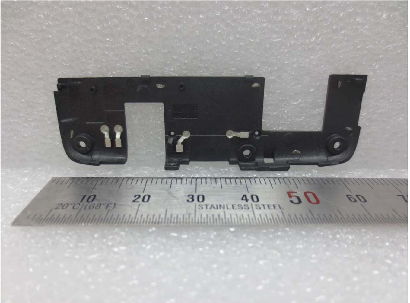
■ BT & WLAN Antenna INTERNAL PHOTO
