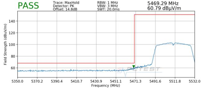
**Plot 7-19. Radiated Lower Band Edge Plot SISO ANT1 (Peak – UNII Band 2C)**
