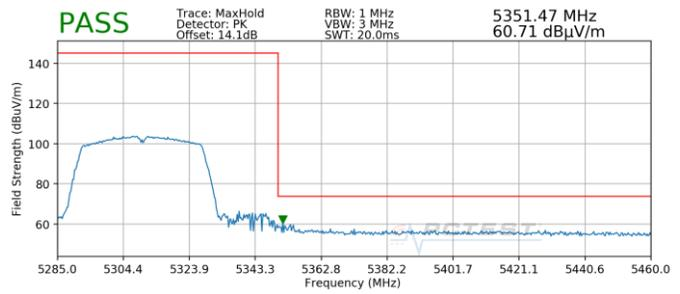
**Plot 7-17. Radiated Upper Band Edge Plot SISO ANT1 (Peak – UNII Band 2A)**
