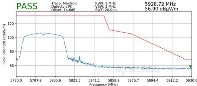
**Plot 7-20. Radiated Upper Band Edge Plot SISO ANT1 (Peak – UNII Band 3)**
