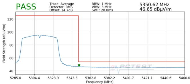
**Plot 7-16. Radiated Upper Band Edge Plot SISO ANT1 (Average – UNII Band 2A)**
