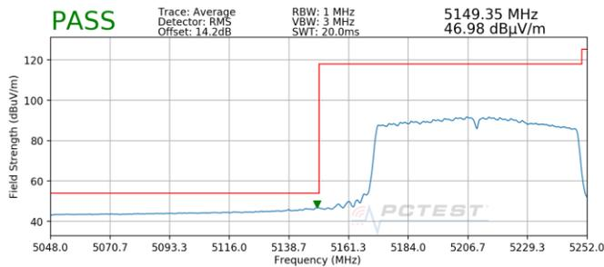
**Plot 7-21. Radiated Lower Band Edge Plot SISO ANT1 (Average – UNII Band 1)**
