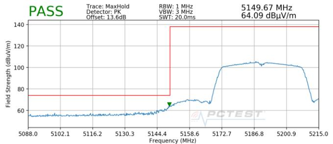
**Plot 7-15. Radiated Lower Band Edge Plot SISO ANT1 (Peak – UNII Band 1)**
