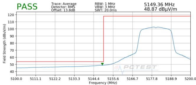
**Plot 7-7. Radiated Lower Band Edge Plot SISO ANT1 (Average – UNII Band 1)**
