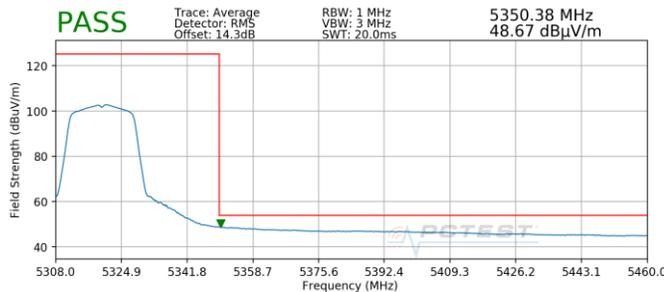
**Plot 7-9. Radiated Upper Band Edge Plot SISO ANT1 (Average – UNII Band 2A)**
