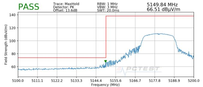
**Plot 7-8. Radiated Lower Band Edge Plot SISO ANT1 (Peak – UNII Band 1)**
