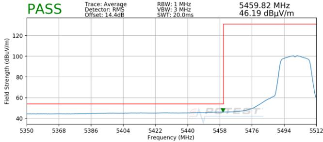
**Plot 7-11. Radiated Lower Band Edge Plot SISO ANT1 (Average – UNII Band 2C)**
