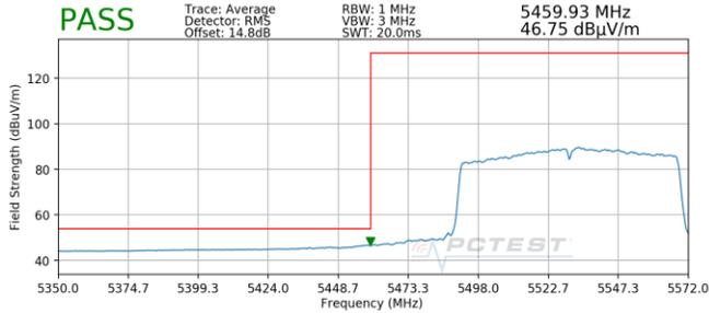
**Plot 7-25. Radiated Lower Band Edge Plot SISO ANT1 (Average – UNII Band 2C)**
