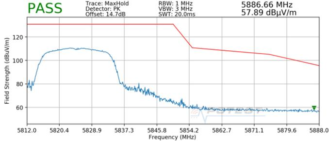
**Plot 7-13. Radiated Upper Band Edge Plot SISO ANT1 (Peak – UNII Band 3)**
