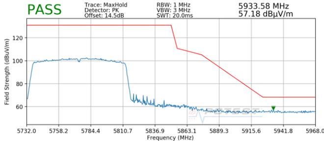
**Plot 7-27. Radiated Upper Band Edge Plot SISO ANT1 (Peak – UNII Band 3)**
