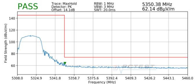
**Plot 7-10. Radiated Upper Band Edge Plot SISO ANT1 (Peak – UNII Band 2A)**
