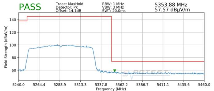
**Plot 7-24. Radiated Upper Band Edge Plot SISO ANT1 (Peak – UNII Band 2A)**
