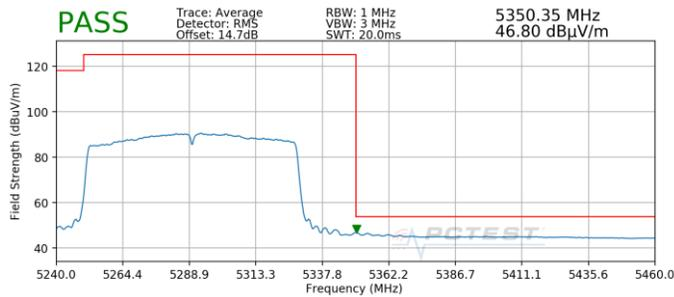
**Plot 7-23. Radiated Upper Band Edge Plot SISO ANT1 (Average – UNII Band 2A)**
