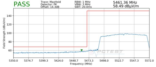
**Plot 7-26. Radiated Lower Band Edge Plot SISO ANT1 (Peak – UNII Band 2C)**
