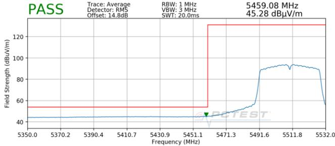
**Plot 7-18. Radiated Lower Band Edge Plot SISO ANT1 (Average – UNII Band 2C)**
