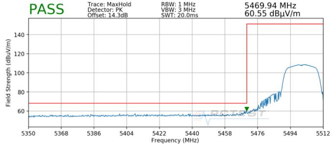
**Plot 7-12. Radiated Lower Band Edge Plot SISO ANT1 (Peak – UNII Band 2C)**
