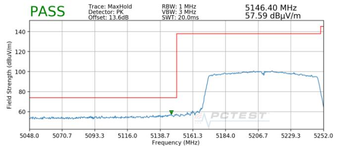
**Plot 7-22. Radiated Lower Band Edge Plot SISO ANT1 (Peak – UNII Band 1)**
