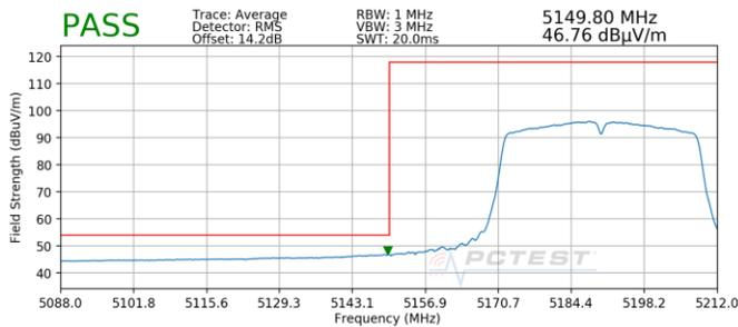
**Plot 7-14. Radiated Lower Band Edge Plot SISO ANT1 (Average – UNII Band 1)**
