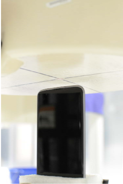
SAR Test Setup Photo 7: Top Edge at 1.0 cm
