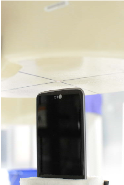
SAR Test Setup Photo 8: Bottom Edge at 1.0 cm
