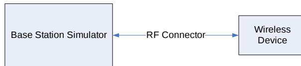
Figure 9-2 Power Measurement Setup
