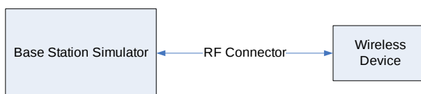
Figure 9-1 Power Measurement Setup
