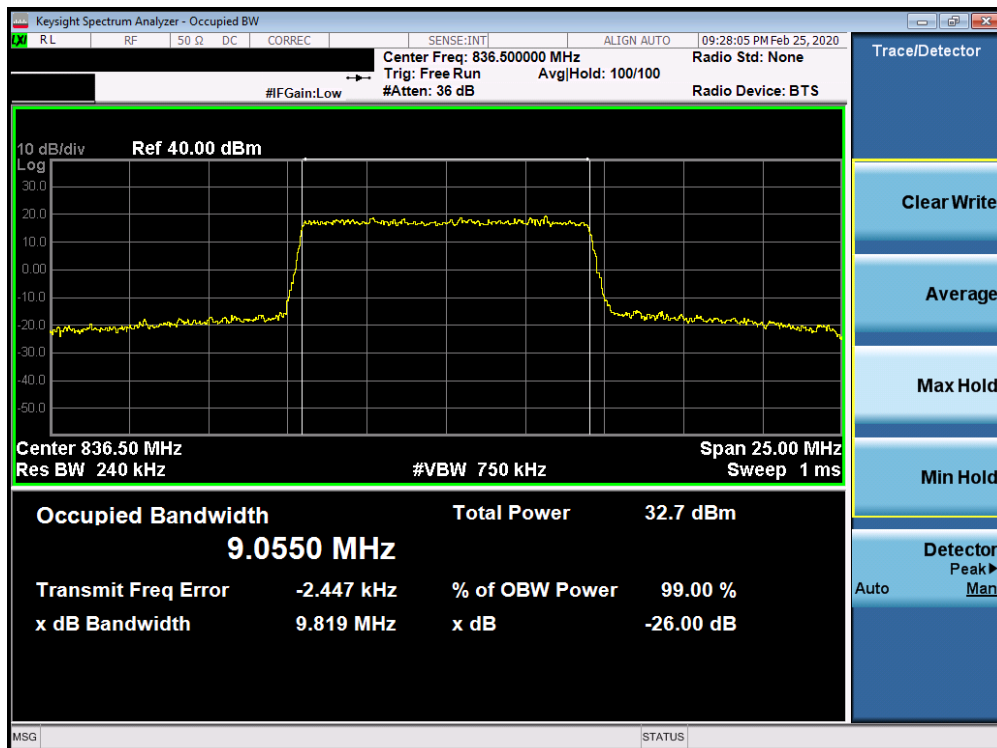
Plot 7-40. Occupied Bandwidth Plot (Band 26/5 - 10.0MHz QPSK - Full RB Configuration)
