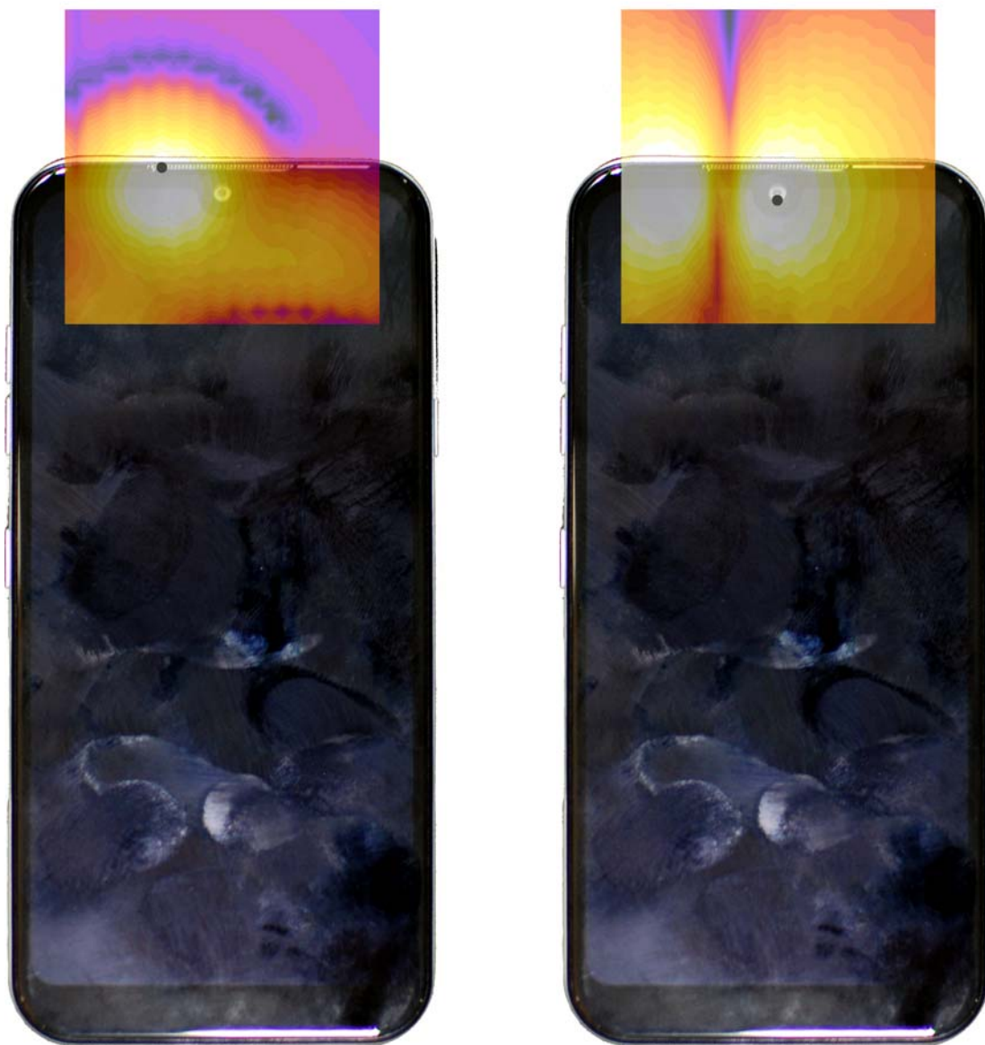
Figure 16-3 T-Coil Scan Overlay Magnetic Field Distributions
