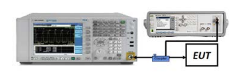
Figure 7-1. Test Instrument & Measurement Setup
