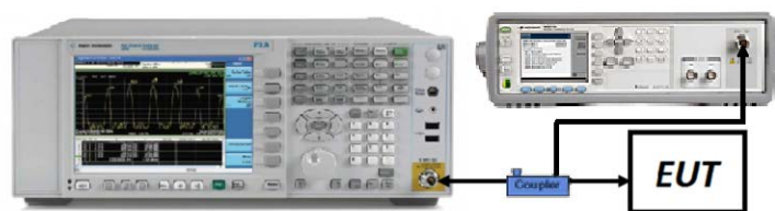
Figure 7-5. Test Instrument & Measurement Setup
