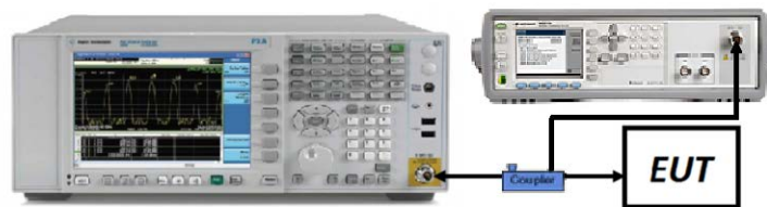
Figure 7-4. Test Instrument & Measurement Setup
