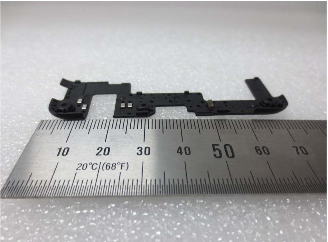
■ BT&WLAN Antenna INTERNAL PHOTO
