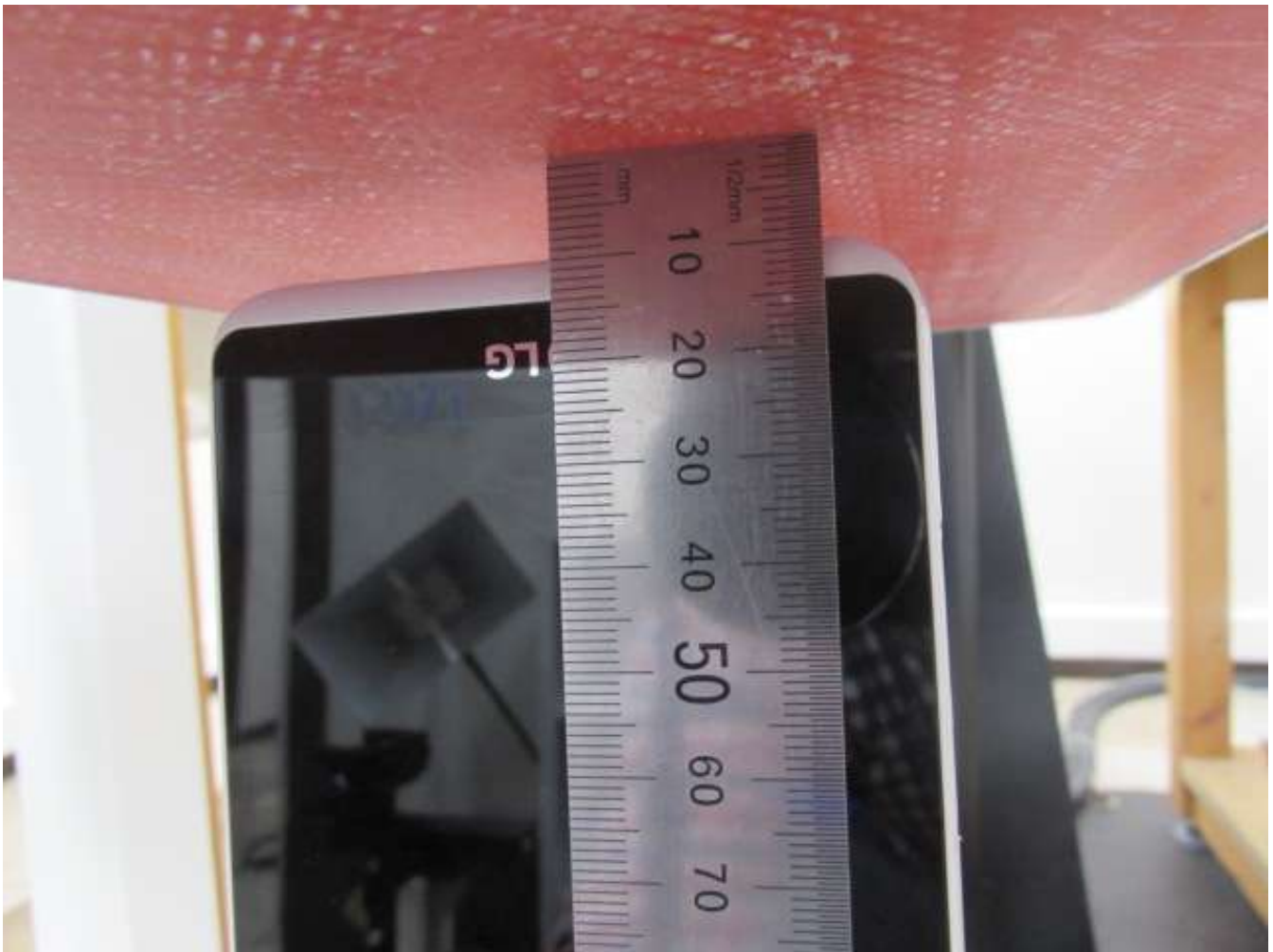
[Distance of 1.0 cm from the EUT]
