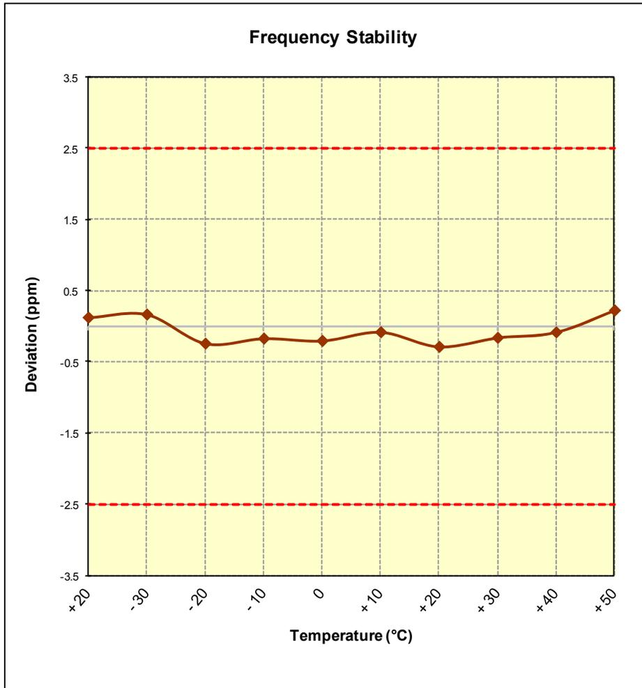
Figure 7-9. Frequency Stability Graph (Cellular WCDMA Mode – Ch. 4183)
