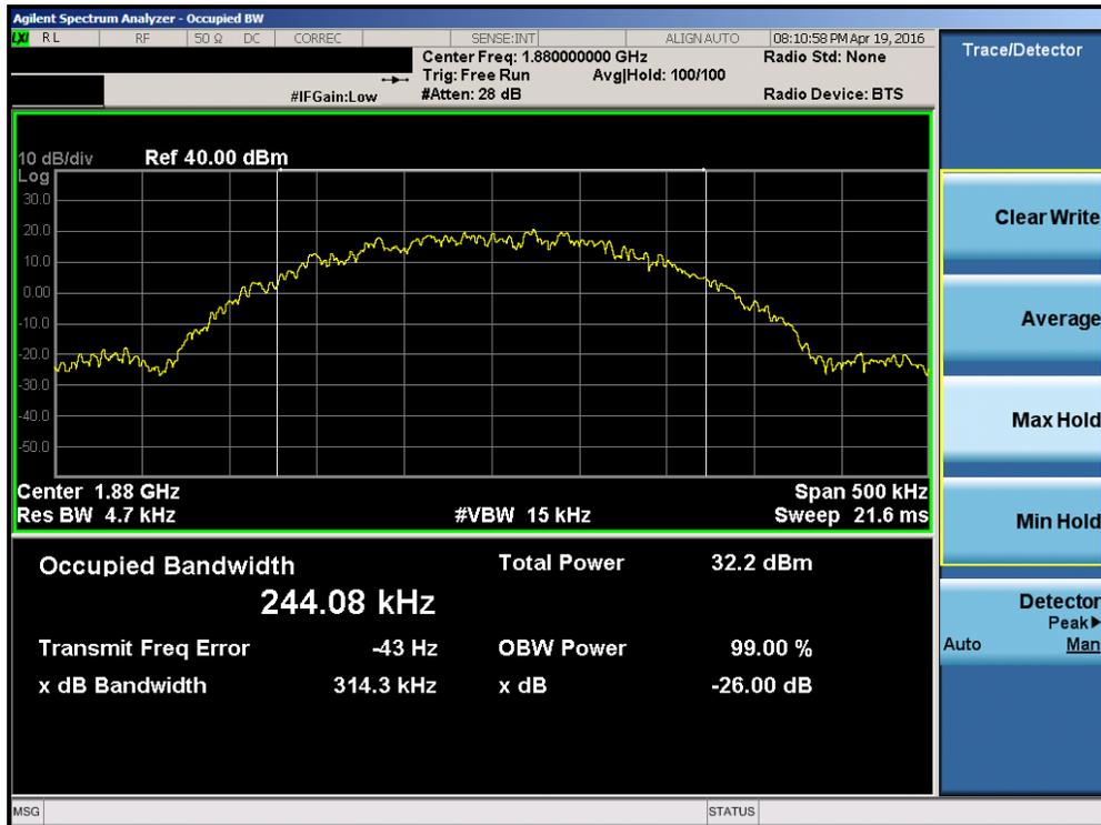
Plot 7-4. Occupied Bandwidth Plot (EDGE1900 Mode – Ch. 661)
