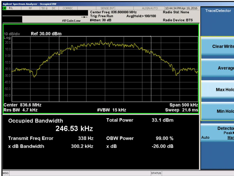
Plot 7-2. Occupied Bandwidth Plot (EDGE850 Mode – Ch. 190)
