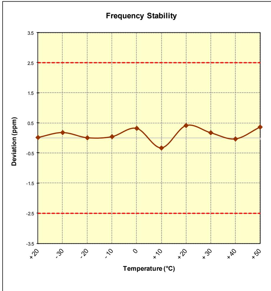
**Figure 7-8. Frequency Stability Graph (Cellular GSM Mode – Ch. 190)**
