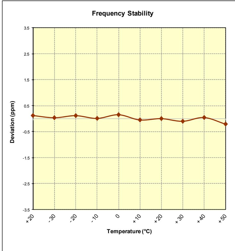
**Figure 7-11. Frequency Stability Graph (PCS GSM Mode – Ch. 661)**
