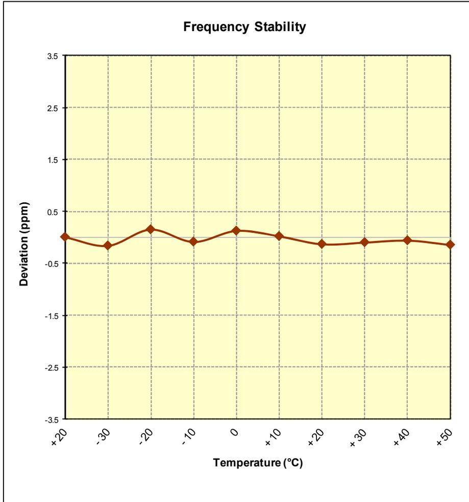
**Figure 7-10. Frequency Stability Graph (AWS WCDMA Mode – Ch. 1412)**
