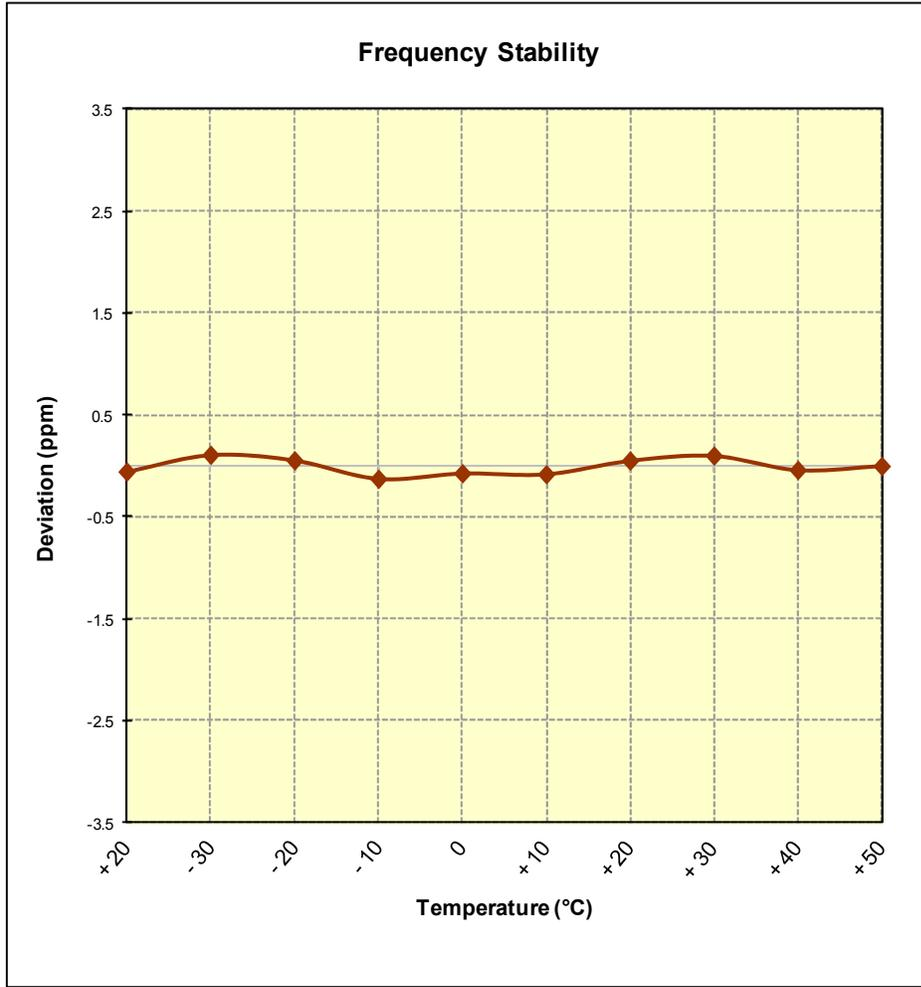
**Figure 7-12. Frequency Stability Graph (PCS WCDMA Mode – Ch. 9400)**
