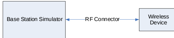
Figure 9-3 Power Measurement Setup
