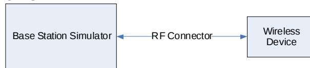
Figure 9-2 Power Measurement Setup
