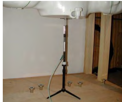
Figure 10-2 System Verification Setup Photo
