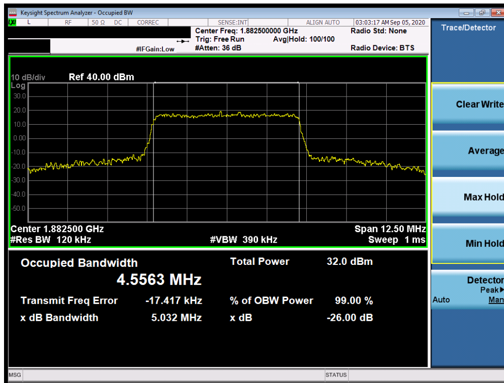
Plot 7-12. Occupied Bandwidth Plot (LTE Band 25/2 - 5MHz 64-QAM - Full RB Configuration)
