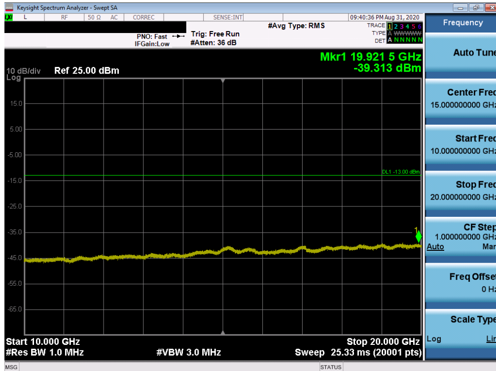
Plot 7-25. Conducted Spurious Plot (LTE Band 25/2 - 20MHz QPSK - RB Size 1, RB Offset 0 - Low Channel)
