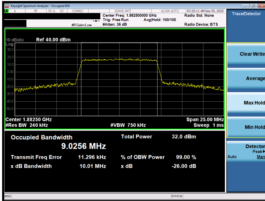
Plot 7-9. Occupied Bandwidth Plot (LTE Band 25/2 - 10MHz 64-QAM - Full RB Configuration)
