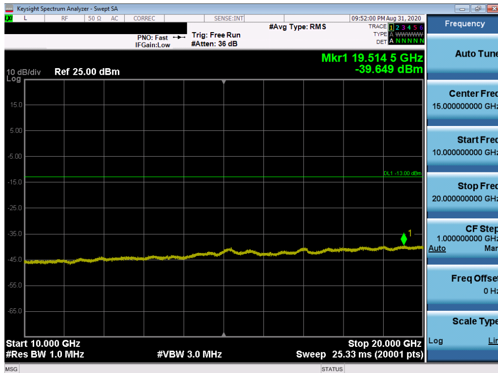
Plot 7-31. Conducted Spurious Plot (LTE Band 25/2 - 20MHz QPSK - RB Size 1, RB Offset 0 - High Channel)
