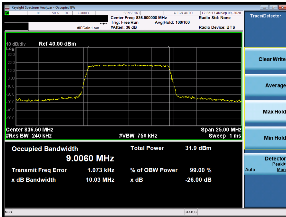
Plot 7-2. Occupied Bandwidth Plot (LTE Band 5 - 10MHz 16-QAM - Full RB Configuration)
