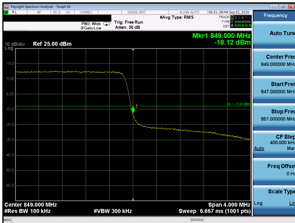
Plot 7-58. Upper Band Edge Plot (LTE Band 5 - 3MHz QPSK – Full RB Configuration)
