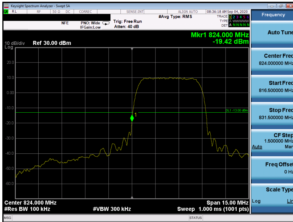
Plot 7-63. Lower Band Edge Plot (WCDMA Cell – Ch. 4132)
