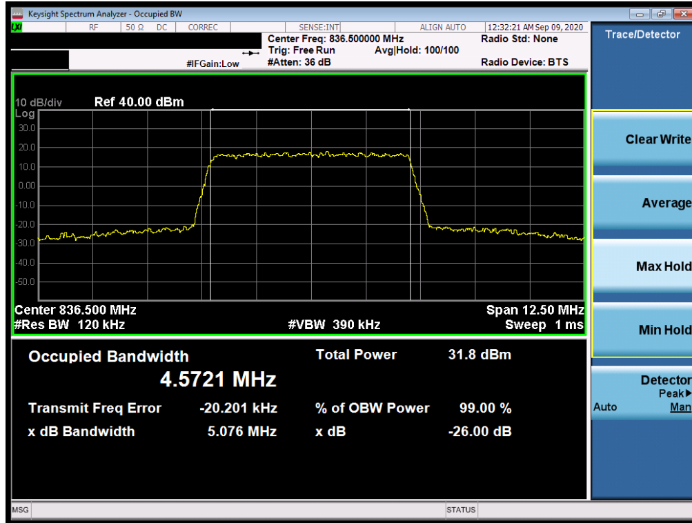
Plot 7-5. Occupied Bandwidth Plot (LTE Band 5 - 5MHz 16-QAM - Full RB Configuration)
