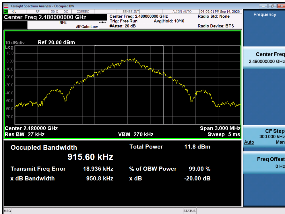
Plot 7-3. 20dB Bandwidth Plot (Bluetooth, 1Mbps – Ch. 78)
