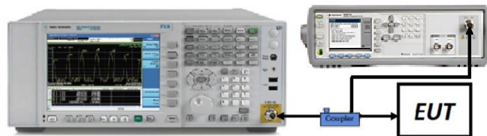
Figure 7-6. Test Instrument & Measurement Setup
