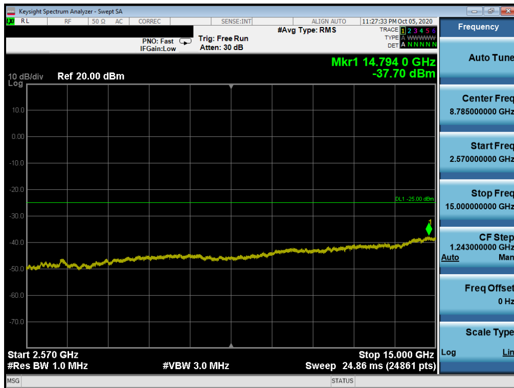
Plot 7-14. Conducted Spurious Plot (LTE Band 7 - 20MHz QPSK - RB Size 1, RB Offset 0 - Low Channel)
