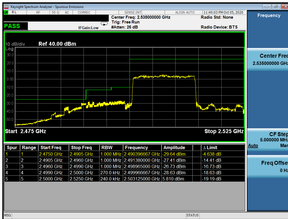
Plot 7-24. Lower ACP Plot (LTE Band 7 - 15MHz QPSK – Full RB Configuration)
