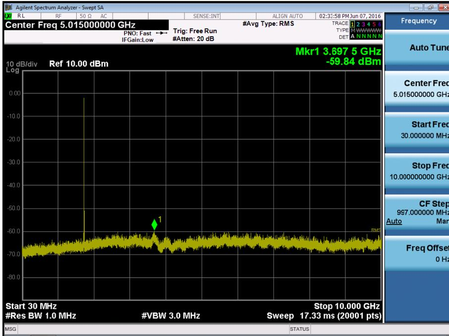
BAND 4. Conducted Spurious Plot\_2 (20350ch\_10MHz\_QPSK\_RB 1\_0)
