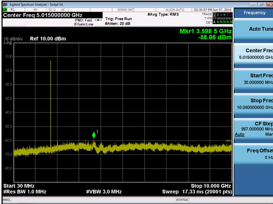
BAND 4. Conducted Spurious Plot\_2 (20175ch\_15MHz\_QPSK\_RB 1\_0)
