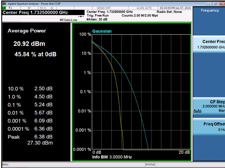
BAND 4. PAR Plot (3M BW\_Ch.20175\_16QAM\_RB15\_0)
