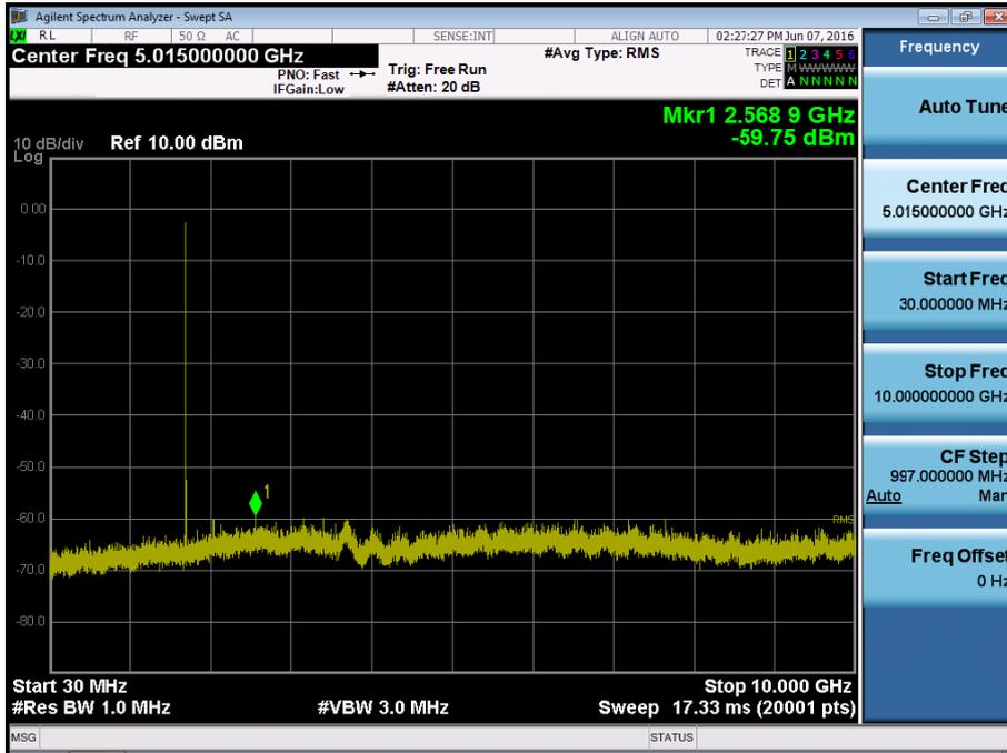
BAND 4. Conducted Spurious Plot\_2 (19975ch\_5MHz\_QPSK\_RB 1\_0)
