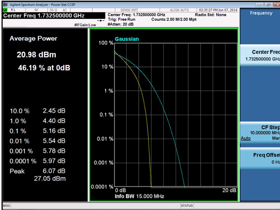
BAND 4. PAR Plot (15M BW\_Ch.20175\_16QAM\_RB75\_0)
