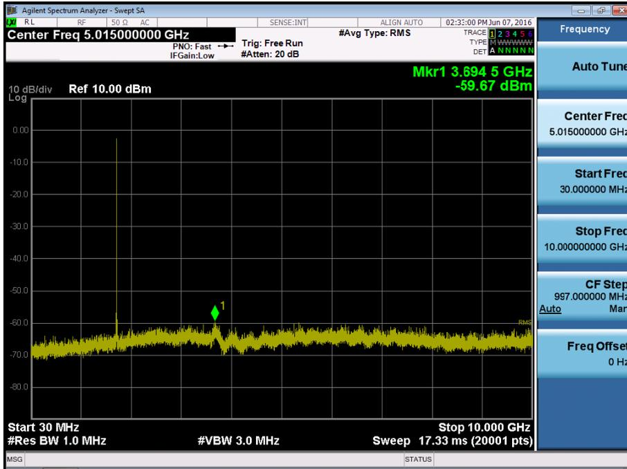
BAND 4. Conducted Spurious Plot\_2 (20175ch\_10MHz\_QPSK\_RB 1\_0)
