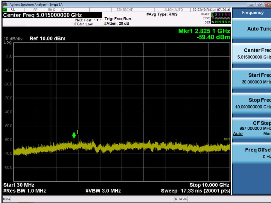
BAND 4. Conducted Spurious Plot\_2 (20393ch\_1.4MHz\_QPSK\_RB 1\_0)
