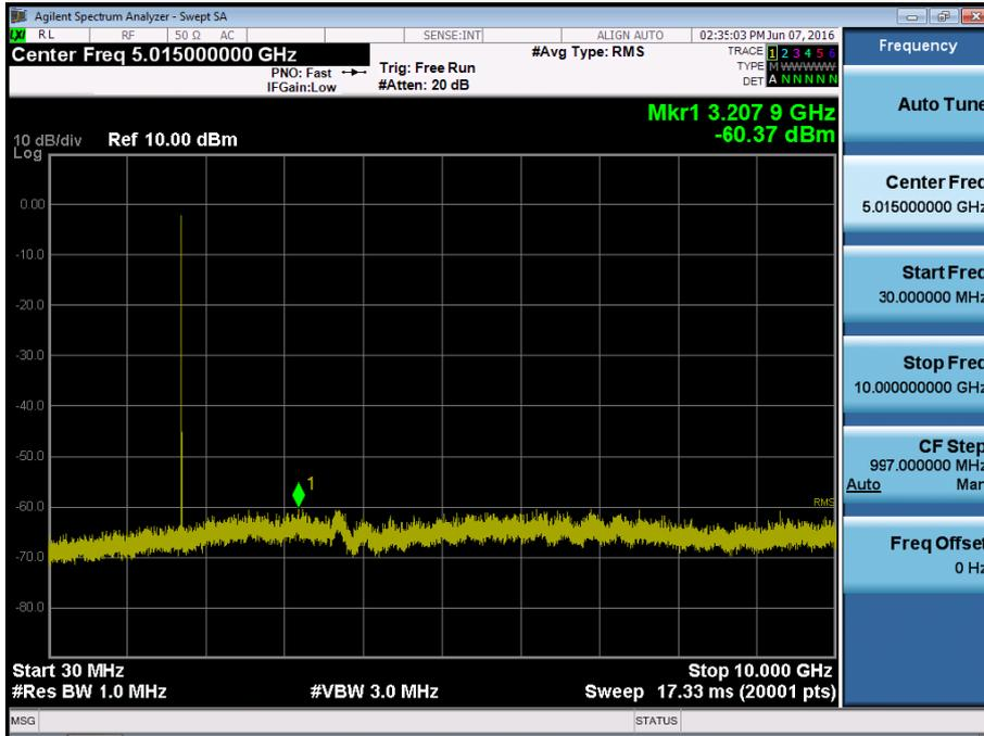
BAND 4. Conducted Spurious Plot\_2 (20025ch\_15MHz\_QPSK\_RB 1\_0)
