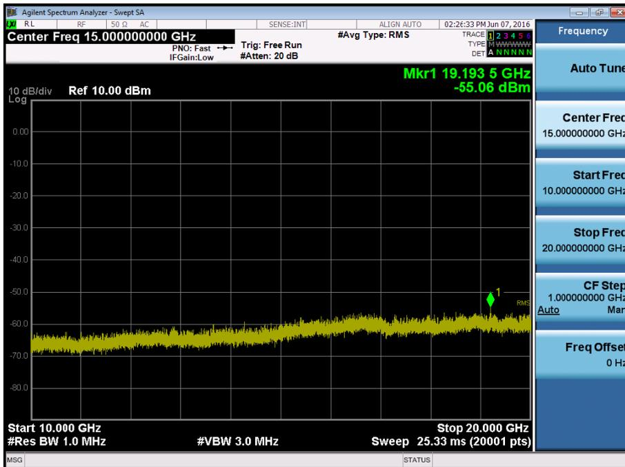
BAND 4. Conducted Spurious Plot\_1 (19975ch\_5MHz\_QPSK\_RB 1\_0)
