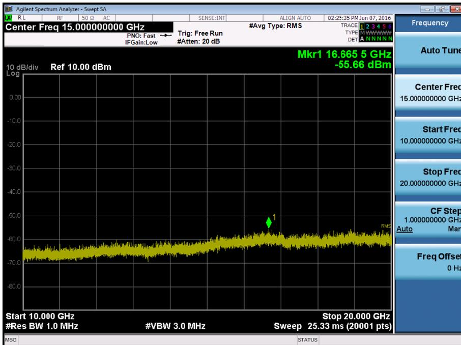
BAND 4. Conducted Spurious Plot\_1 (20385ch\_3MHz\_QPSK\_RB 1\_0)
