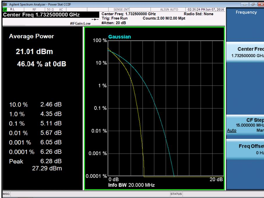
BAND 4. PAR Plot (20M BW\_Ch.20175\_16QAM\_RB100\_0)
