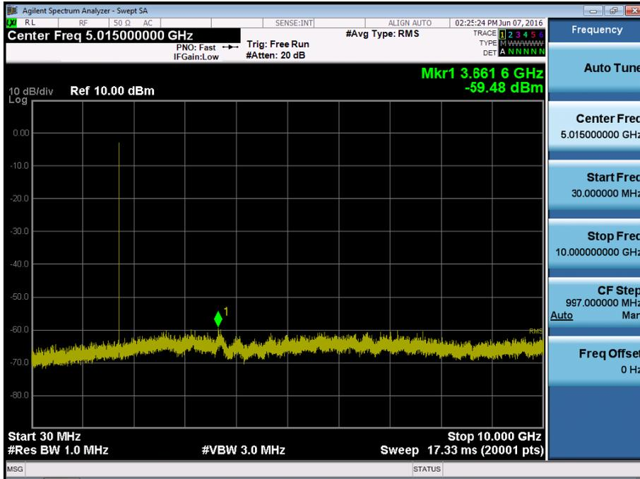
BAND 4. Conducted Spurious Plot\_2 (20175ch\_3MHz\_QPSK\_RB 1\_0)
