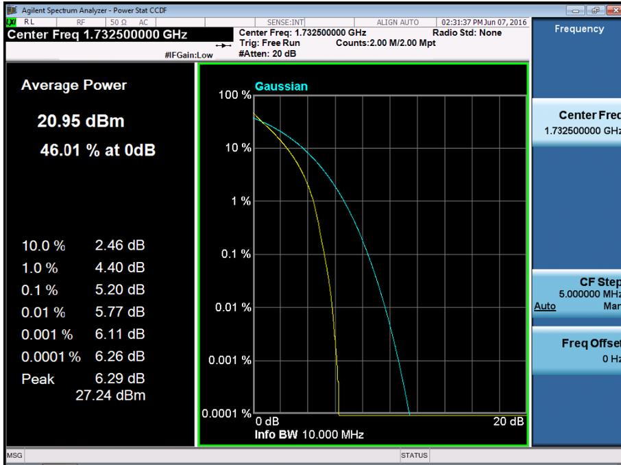
BAND 4. PAR Plot (10M BW\_Ch.20175\_16QAM\_RB50\_0)
