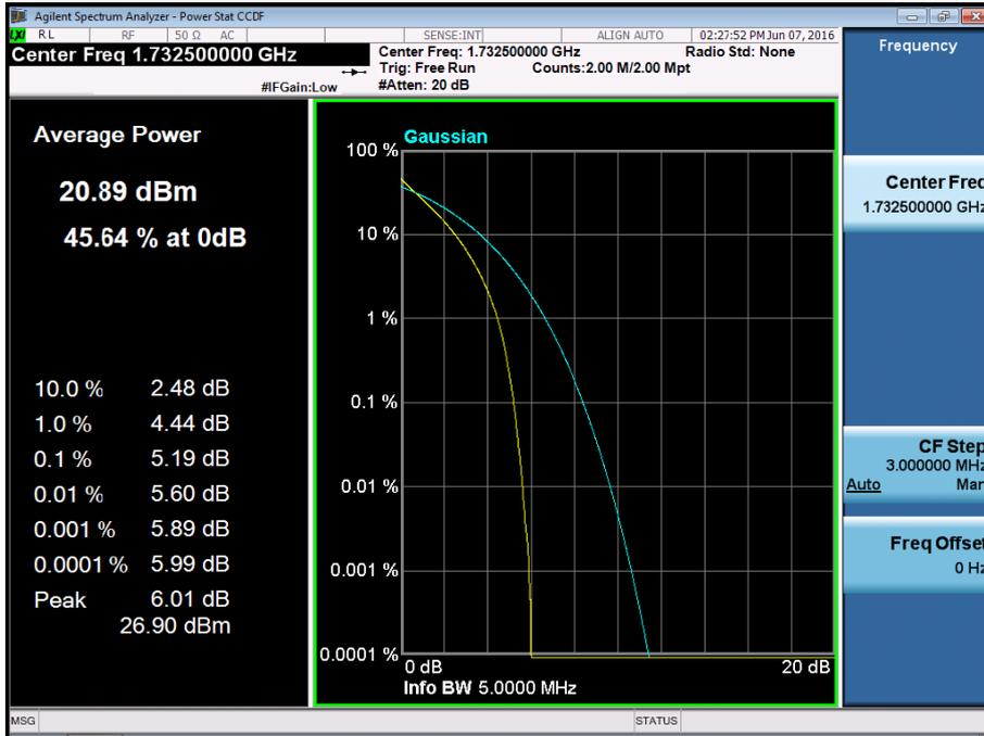
BAND 4. PAR Plot (5M BW\_Ch.20175\_16QAM\_RB25\_0)
