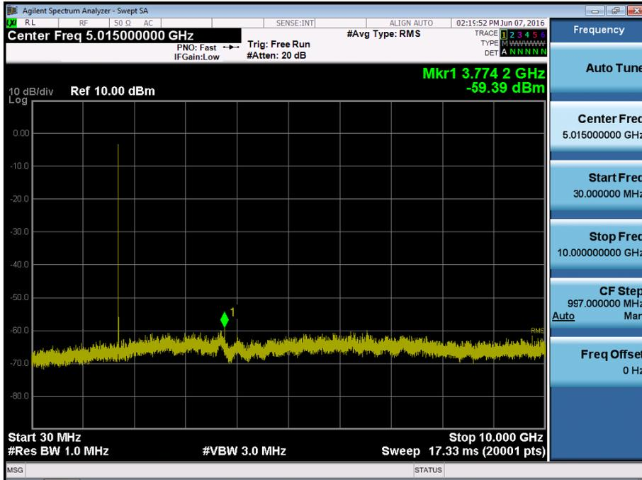
BAND 4. Conducted Spurious Plot\_2 (19957ch\_1.4MHz\_QPSK\_RB 1\_0)
