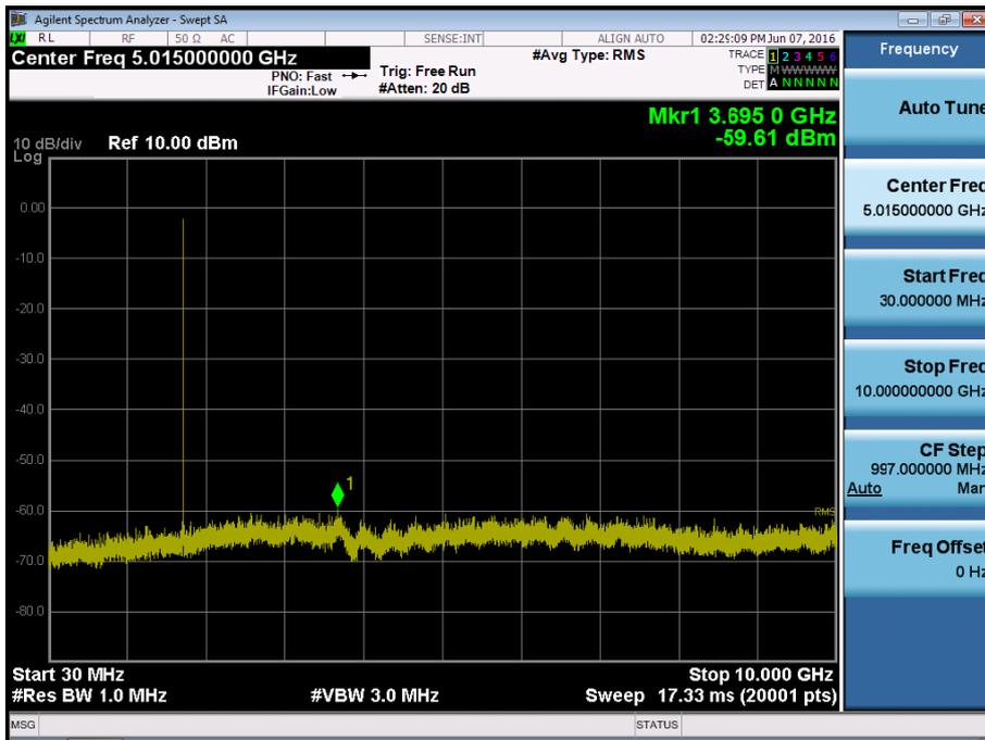
BAND 4. Conducted Spurious Plot\_2 (20175ch\_5MHz\_QPSK\_RB 1\_0)
