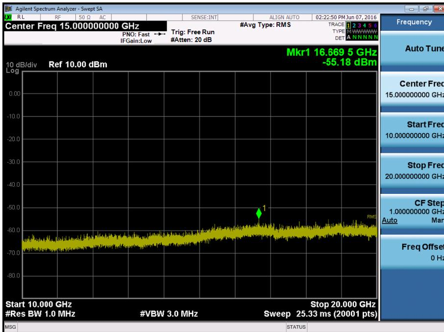
BAND 4. Conducted Spurious Plot\_1 (19965ch\_3MHz\_QPSK\_RB 1\_0)
