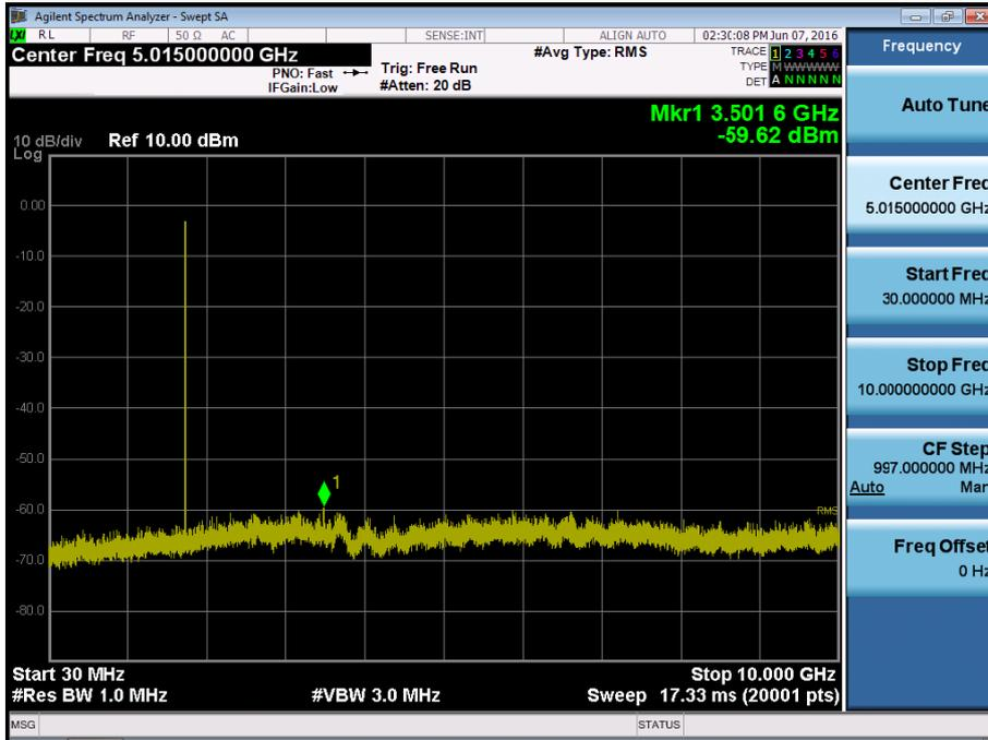
BAND 4. Conducted Spurious Plot\_2 (20375ch\_5MHz\_QPSK\_RB 1\_0)
