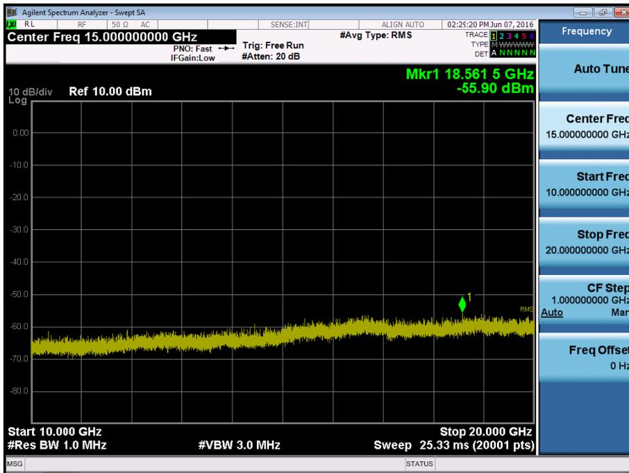
BAND 4. Conducted Spurious Plot\_1 (20375ch\_5MHz\_QPSK\_RB 1\_0)
