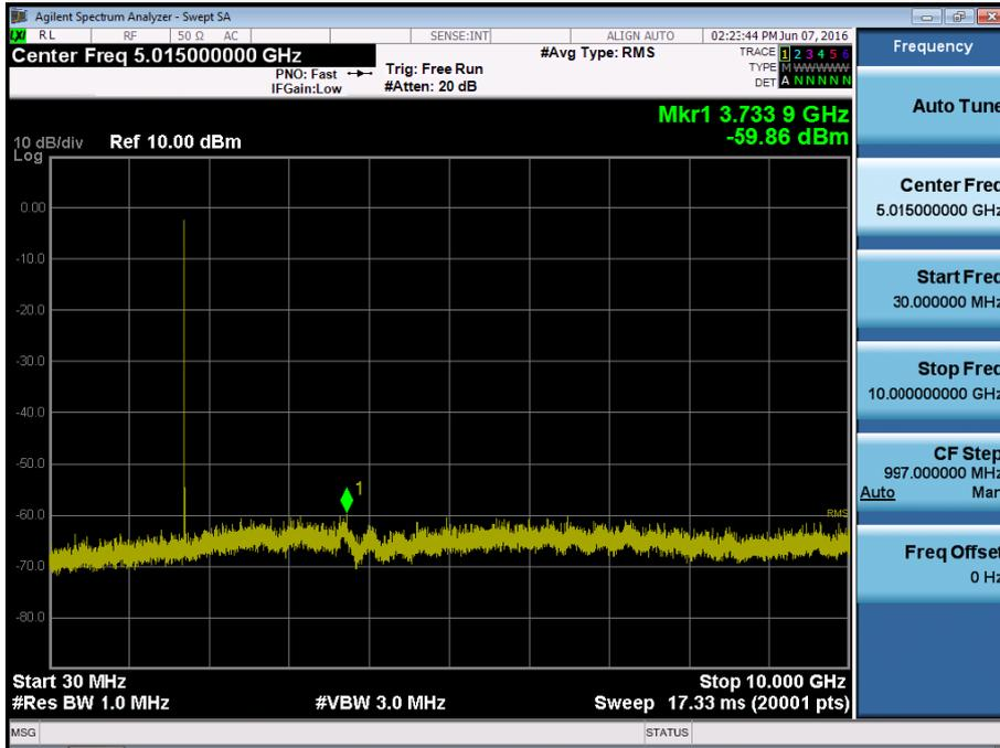
BAND 4. Conducted Spurious Plot\_2 (19965ch\_3MHz\_QPSK\_RB 1\_0)
