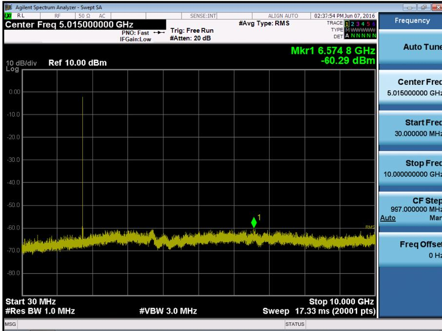
BAND 4. Conducted Spurious Plot\_2 (20325ch\_15MHz\_QPSK\_RB 1\_0)
