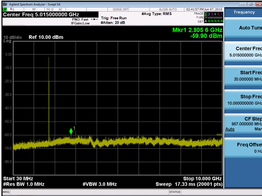
BAND 4. Conducted Spurious Plot\_2 (20300ch\_20MHz\_QPSK\_RB 1\_0)
