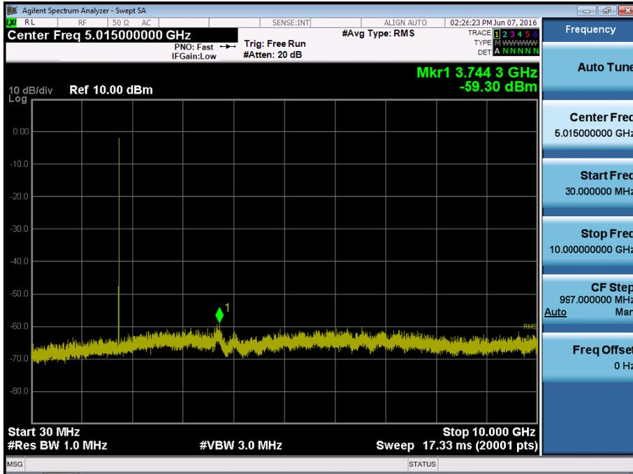
BAND 4. Conducted Spurious Plot\_2 (20385ch\_3MHz\_QPSK\_RB 1\_0)
