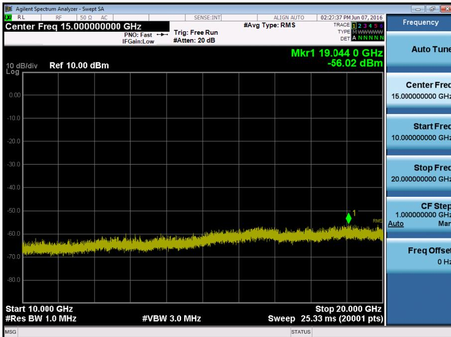
BAND 4. Conducted Spurious Plot\_1 (20175ch\_5MHz\_QPSK\_RB 1\_0)
