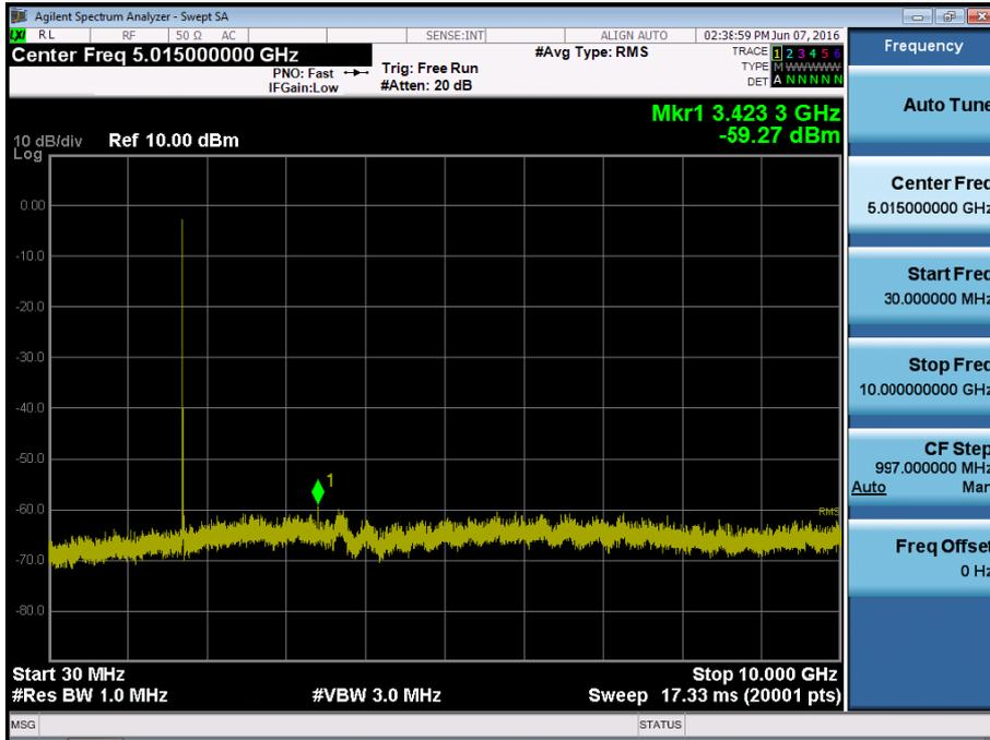
BAND 4. Conducted Spurious Plot\_2 (20050ch\_20MHz\_QPSK\_RB 1\_0)
