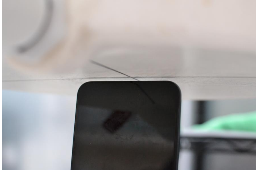
SAR Test Setup Photo 11 Bottom Edge 2 mm
