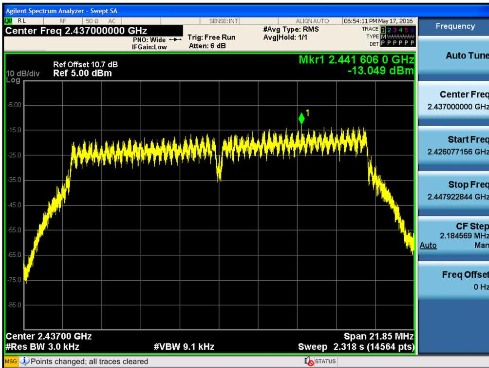
**Power Spectral Density (802.11n\_HT20 -CH 6)**
