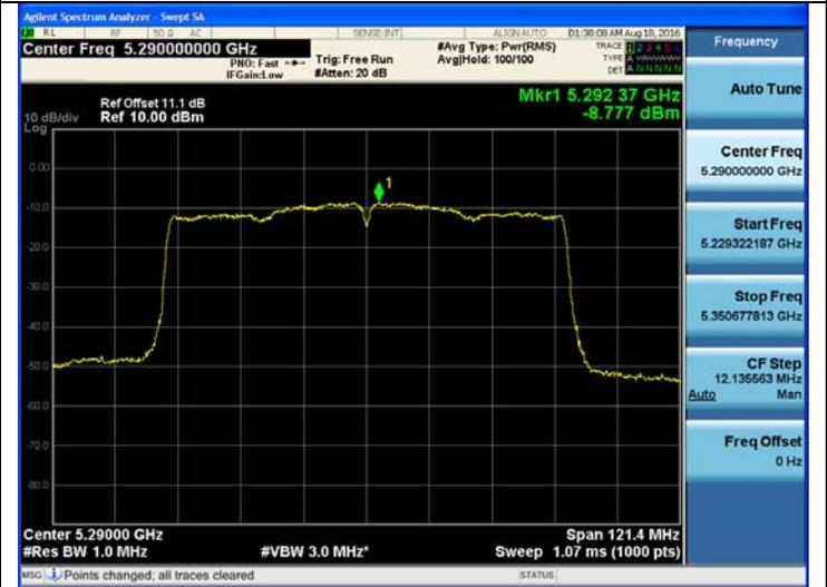
802.11ac\_VHT80 UNII 2C BAND PSD CH 106
