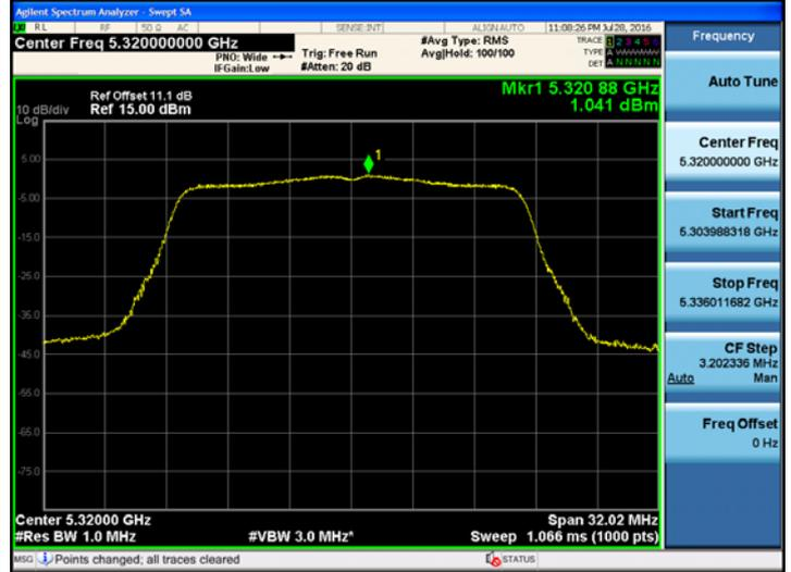
802.11ac\_VHT20 UNII 2C BAND PSD CH 100
