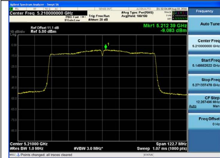
802.11ac\_VHT80 UNII 2A BAND PSD CH 58
