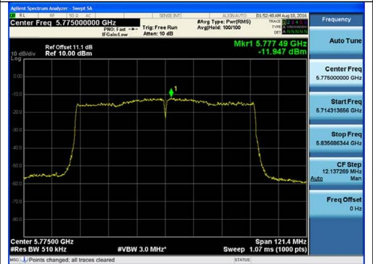
■ Straddle channels TEST RESULTS for 802.11a/n\_HT20/ac\_VHT20
