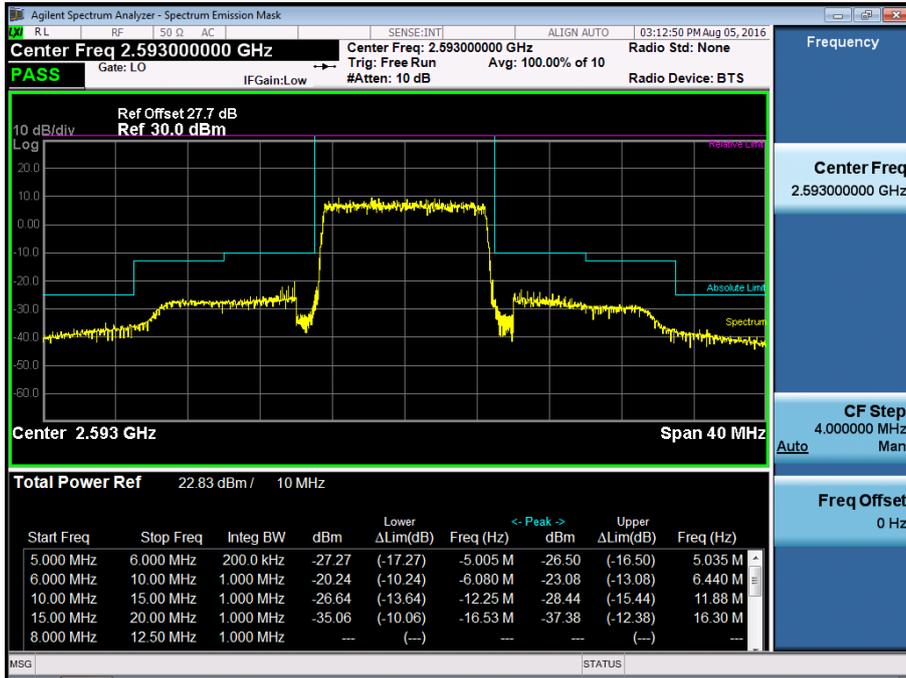
BAND 41. High Channel Edge Plot (10 MHz Ch.41540 QPSK RB 50)
