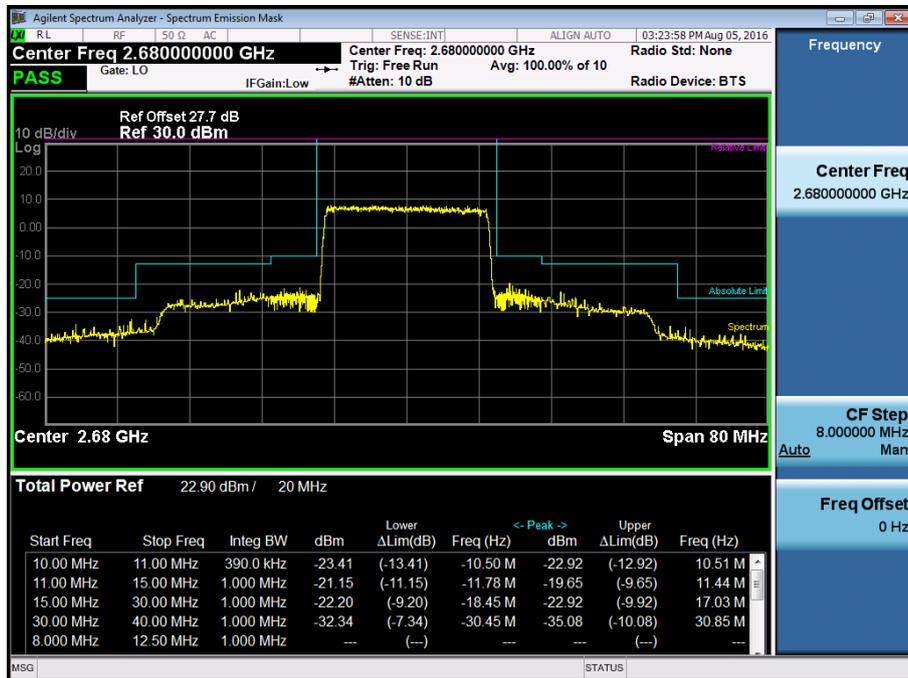
BAND 41. Conducted Spurious Plot 1 (5 MHz Ch.39675 QPSK RB 1, Offset 0)
