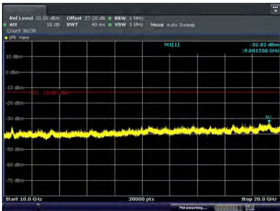
BAND 4. Conducted Spurious Plot_2 (20300ch_20MHz_QPSK_ RB 1_0)
