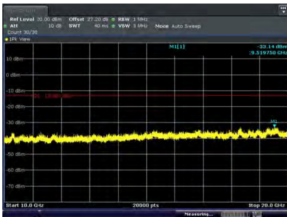
BAND 4. Conducted Spurious Plot_2 (20175ch_10MHz_QPSK_ RB 1_0)
