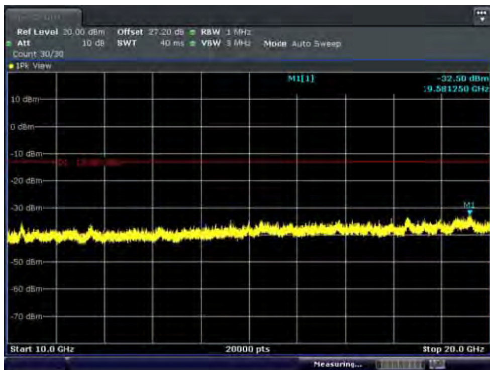
BAND 4. Conducted Spurious Plot_2 (20050ch_20MHz_QPSK_ RB 1_0)
