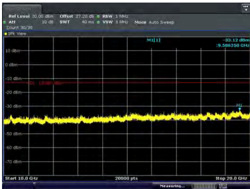
BAND 4. Conducted Spurious Plot_2 (20175ch_20MHz_QPSK_ RB 1_0)
