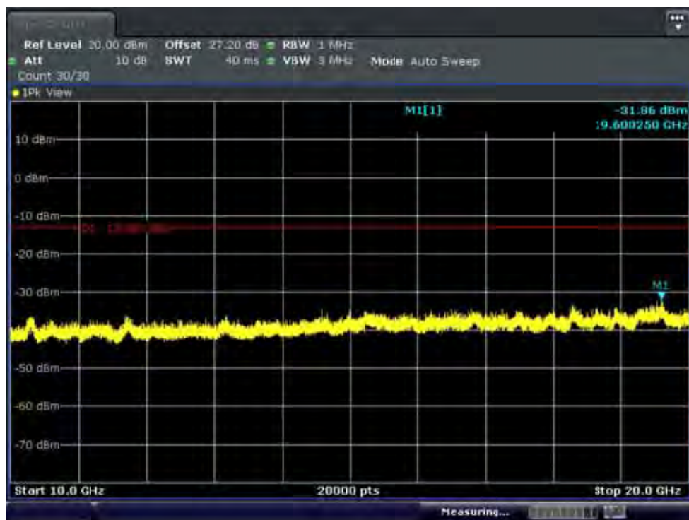
BAND 4. Conducted Spurious Plot_2 (20175ch_5MHz_QPSK_RB 1_0)
