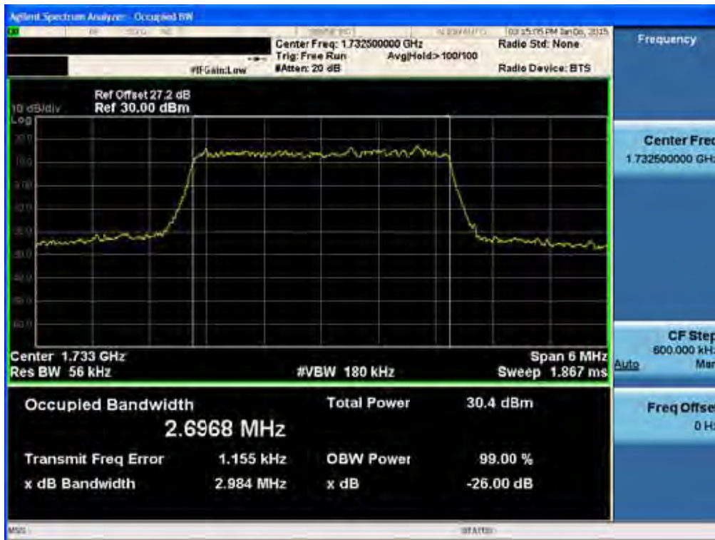
BAND 4. Occupied Bandwidth Plot (3M BW Ch.20175 QPSK RB 15)
