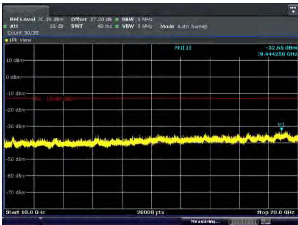
BAND 4 . Conducted Spurious Plot_2 (20325ch_15MHz_QPSK_ RB 1_0)
