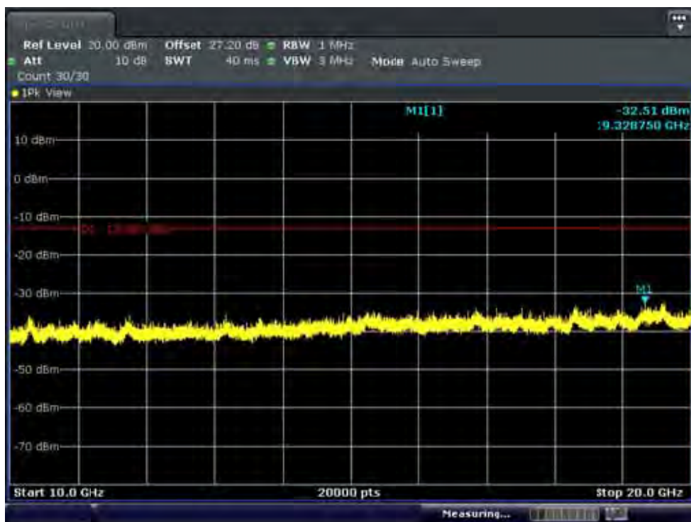
BAND 4 . Conducted Spurious Plot_2 (20375ch_5MHz_QPSK_RB 1_0)
