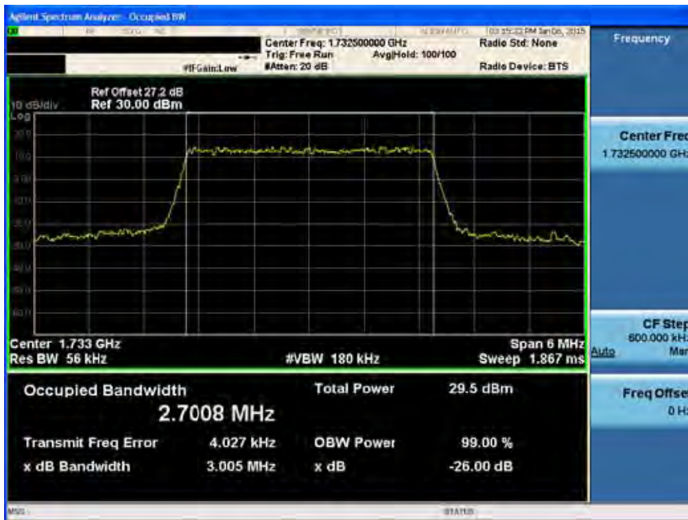
BAND 4. Occupied Bandwidth Plot (3M BW Ch.20175 16QAM RB 15)
