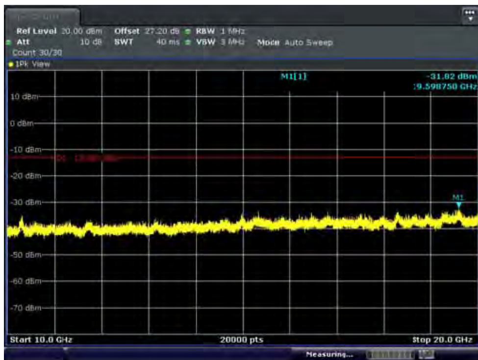
BAND 4. Conducted Spurious Plot_2 (19965ch_3MHz_QPSK_RB 1_0)
