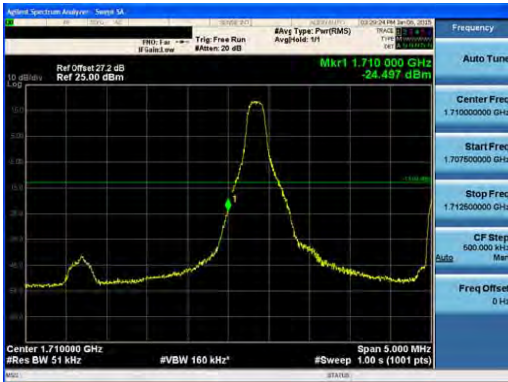
BAND 4. Lower Band Edge Plot (5M BW Ch.19975 QPSK RB 1, Offset 0) -1
