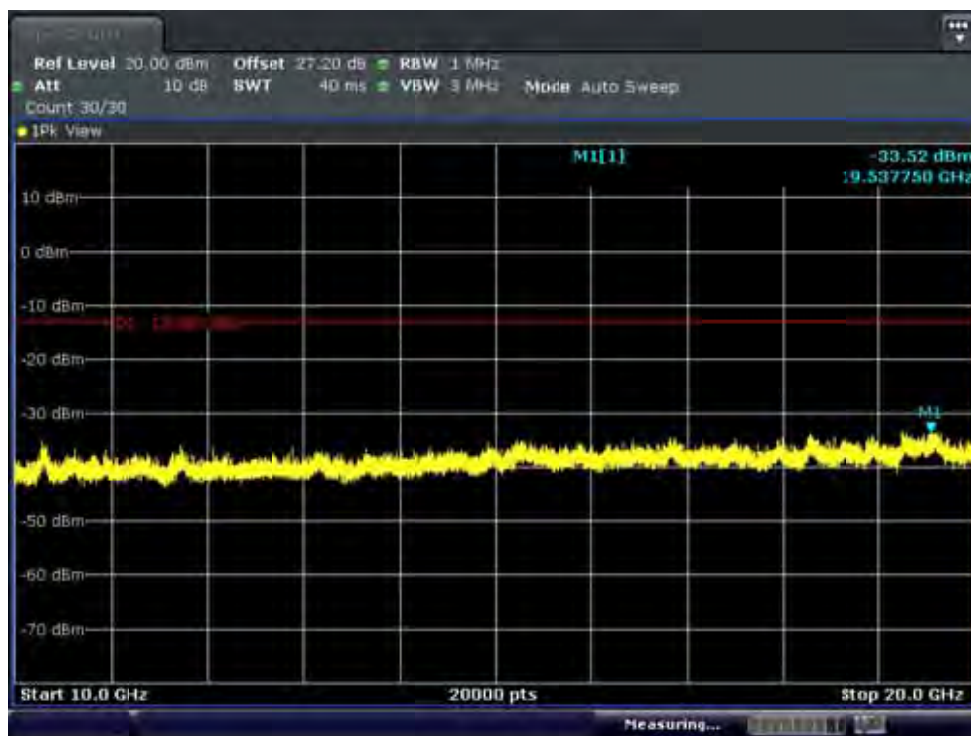
BAND 4. Conducted Spurious Plot_2 (19957ch_1.4MHz_QPSK_RB 1_0)
