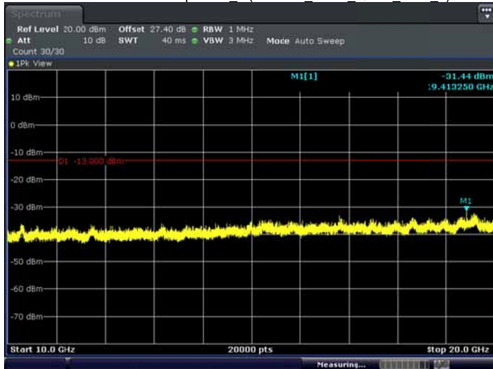
BAND 2. Conducted Spurious_2 (19175ch_5MHz_QPSK_RB 1_0)
