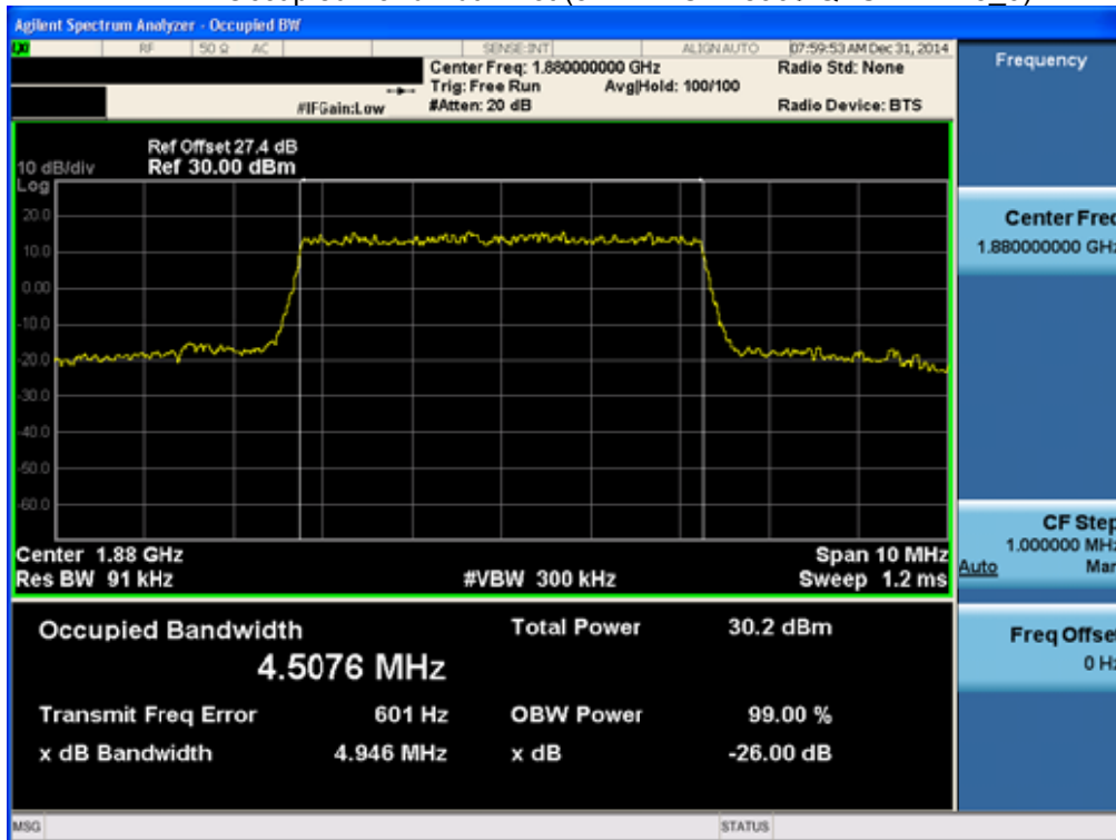
BAND 2. Occupied Bandwidth Plot (5M BW Ch.18900 QPSK RB 25_0)
