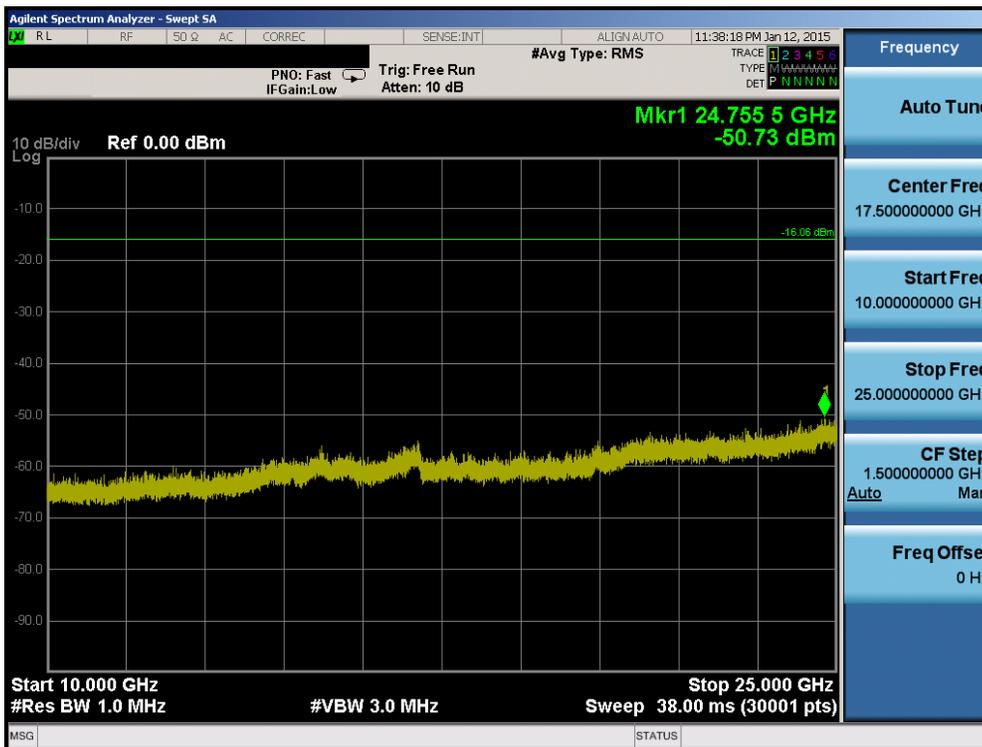
Plot 6-17. Conducted Spurious Plot (Bluetooth (LE) – Ch. 39)
