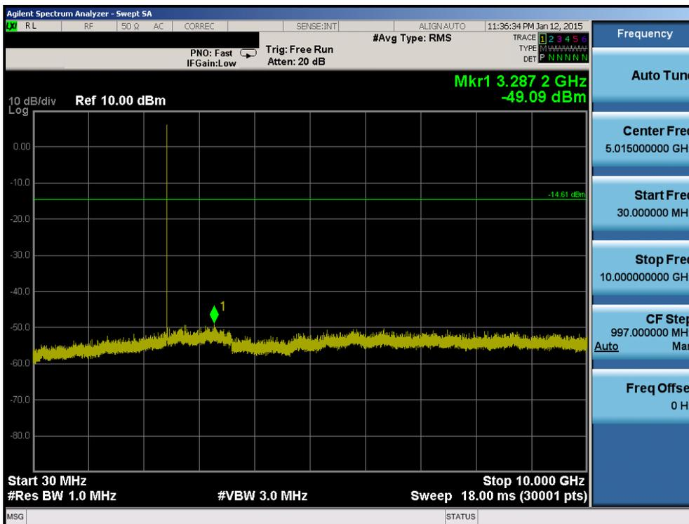
Plot 6-14. Conducted Spurious Plot (Bluetooth (LE) – Ch. 19)
