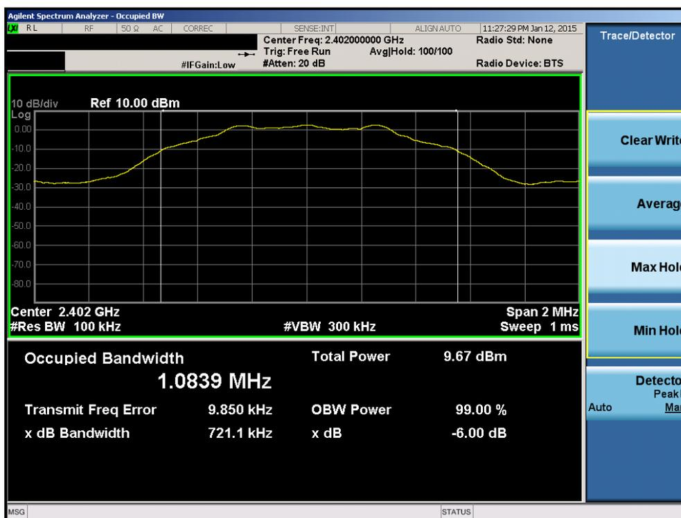
**Plot 6-1. 6dB Bandwidth Plot (Bluetooth (LE) – Ch. 0)**
