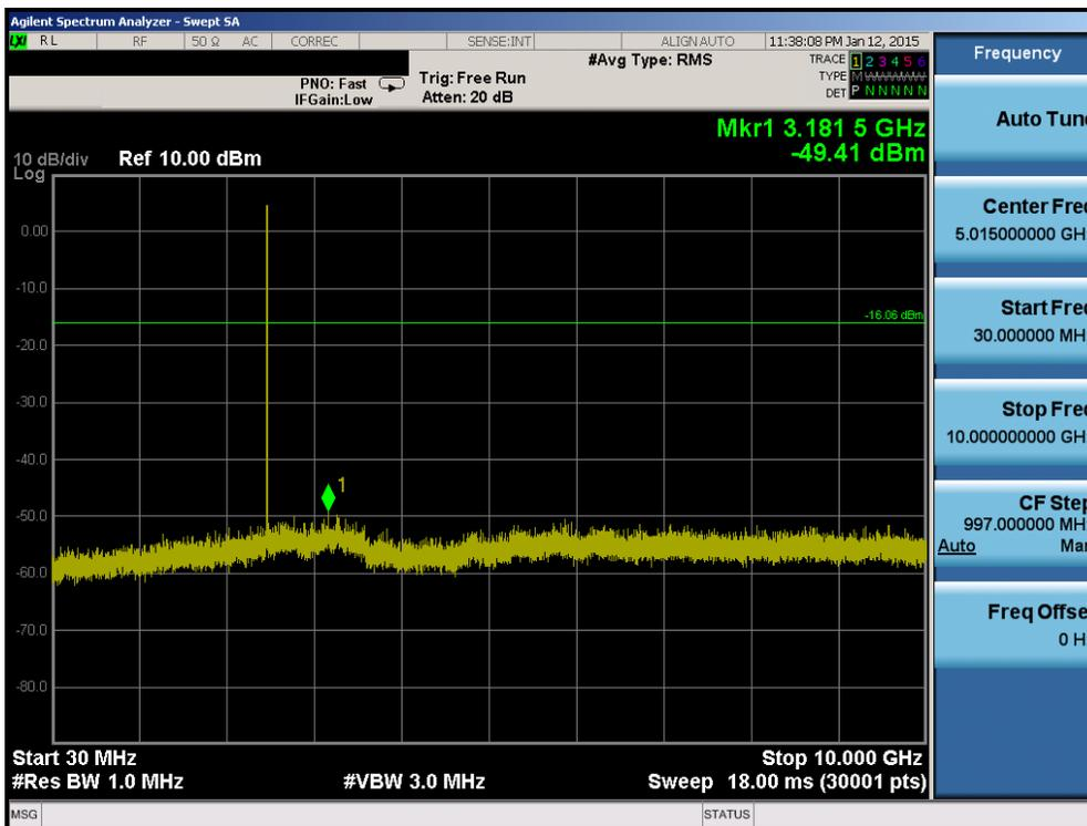
Plot 6-16. Conducted Spurious Plot (Bluetooth (LE) – Ch. 39)
