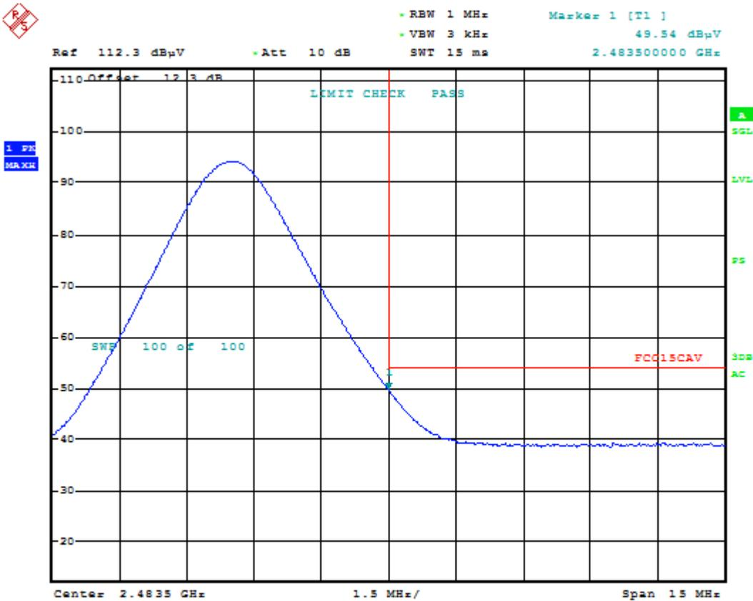
Plot 6-26. Radiated Restricted Upper Band Edge Measurement (Average)
