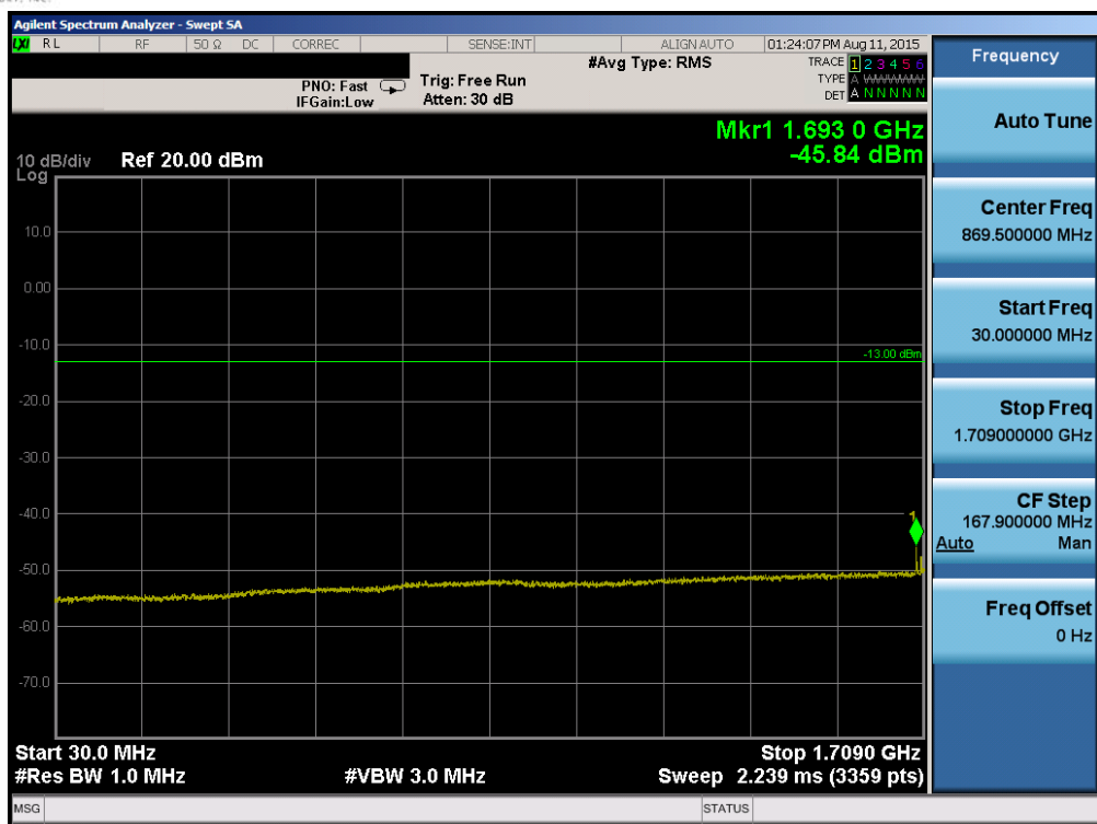
Plot 6-63. Conducted Spurious Plot (Band 4 – 20.0MHz QPSK – RB Size 1, RB Offset 0– Low Channel)
