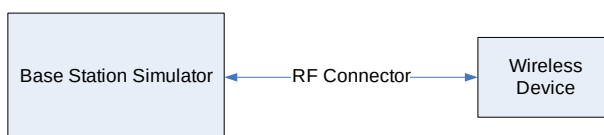
Figure 9-1 Power Measurement Setup
