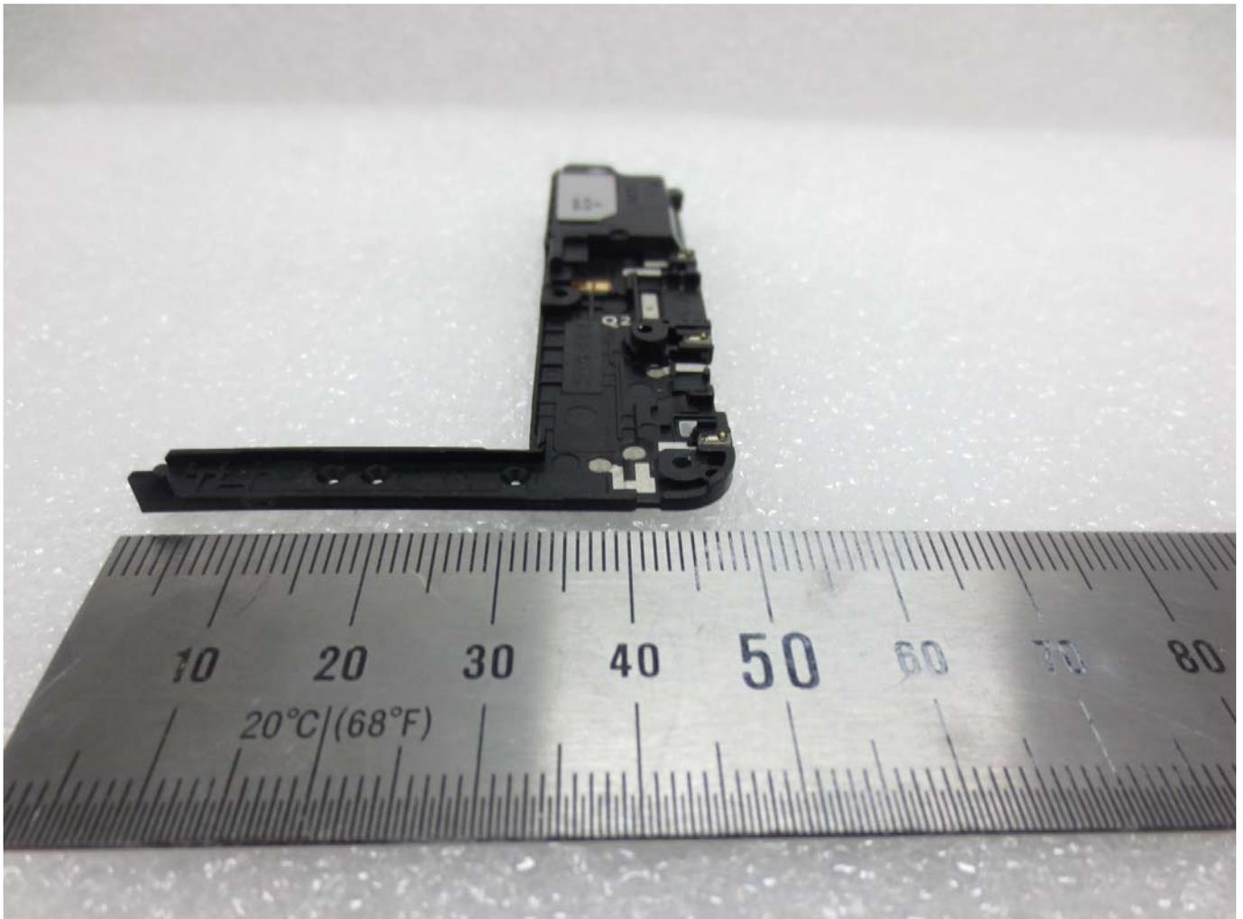
■ BT & WLAN Antenna INTERNAL PHOTO
