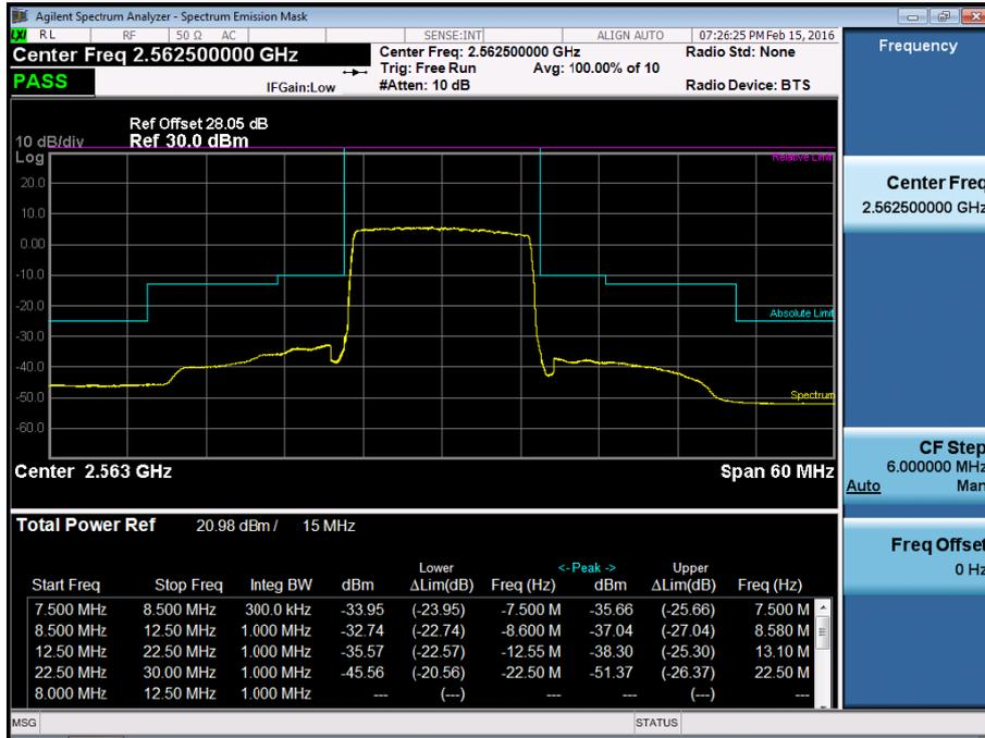
BAND7. Low Channel Edge Plot (20MHz Ch.20850 QPSK RB 100)
