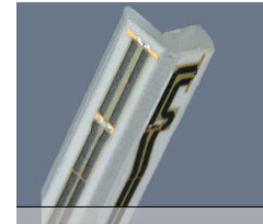
Figure 5-1 E-field Free-space Probe
