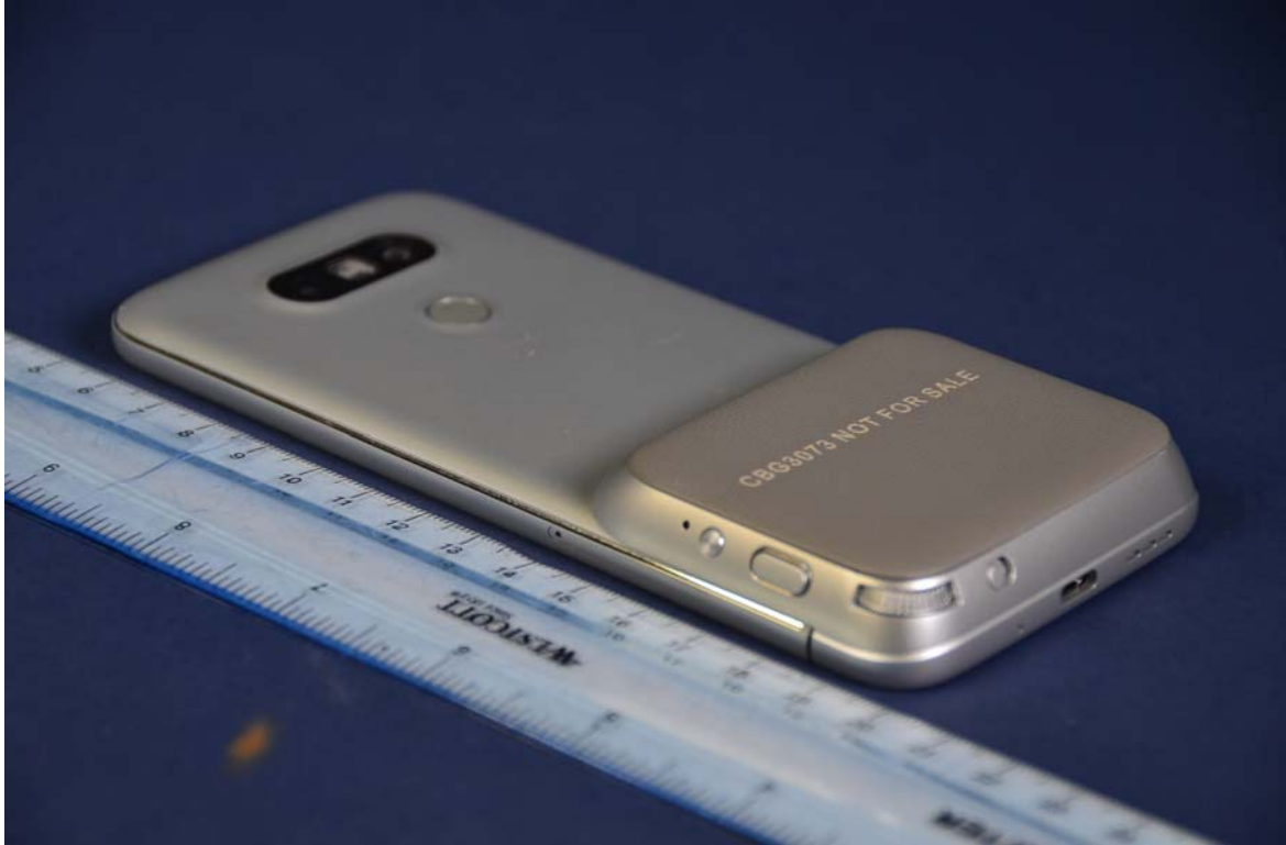
Camera Module Installed
