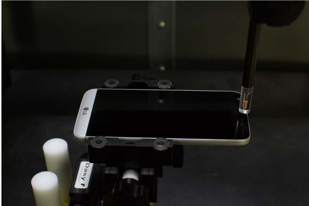
Figure 14-1 Test Setup for Wireless Device
