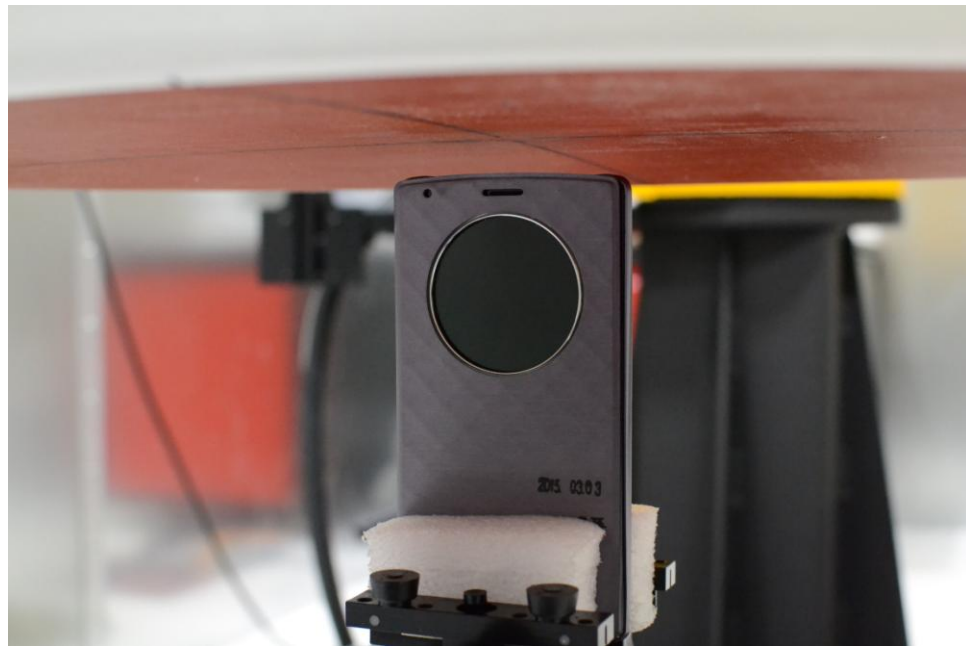
SAR Test Setup Photo 18: Top Edge, Quick Cover (Closed) at 10 mm
