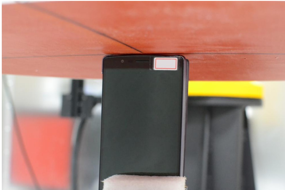
SAR Test Setup Photo 20: Top Edge, Quick Cover (Open) at 0 mm
