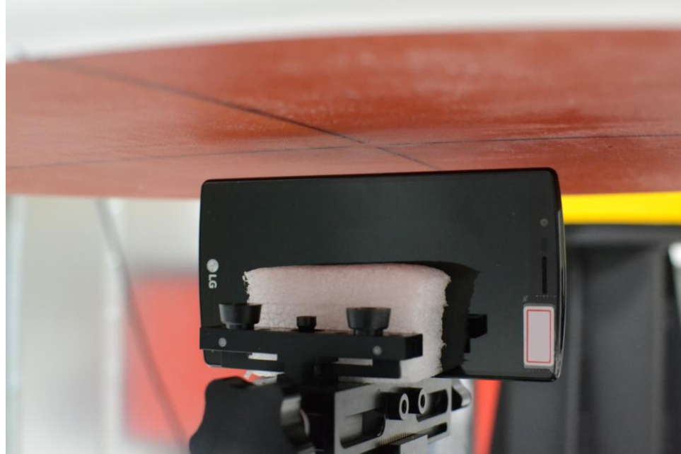
SAR Test Setup Photo 25: Left Edge, Standard Cover at 10 mm
