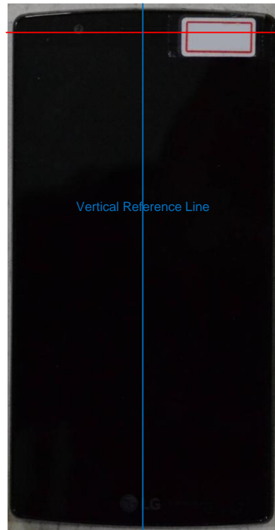
SAR Test Setup Photo 26: Horizontal and Vertical Reference Lines
