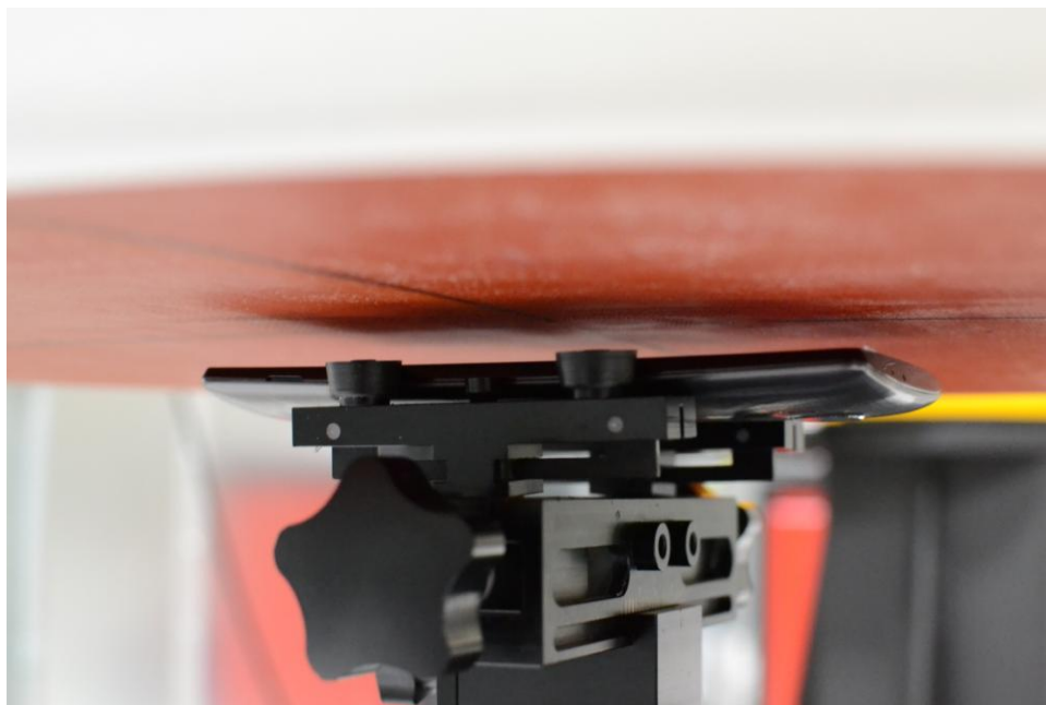
SAR Test Setup Photo 14: Front Side, Standard Cover at 10 mm
