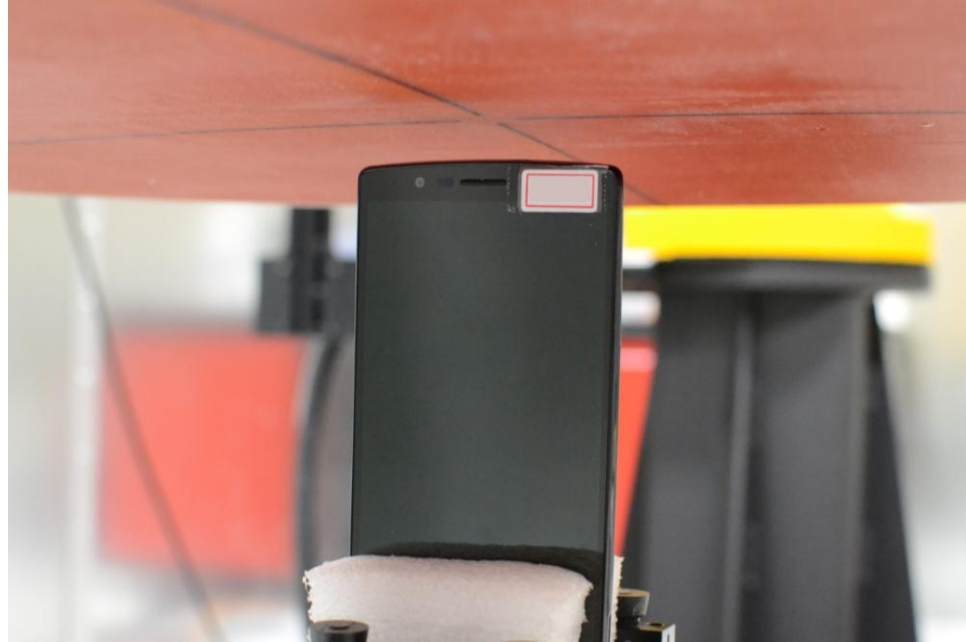
SAR Test Setup Photo 17: Top Edge, Standard Cover at 10 mm
