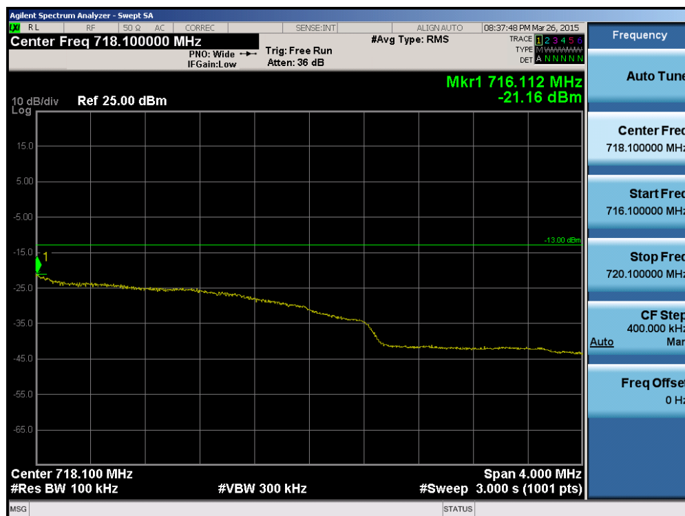
Plot 6-102. Upper Extended Band Edge Plot (Band 12 – 3.0MHz QPSK – RB Size 15)
