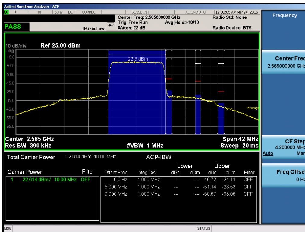
Plot 6-174. Upper ACP Plot (Band 7 – 10.0MHz QPSK – RB Size 50)
