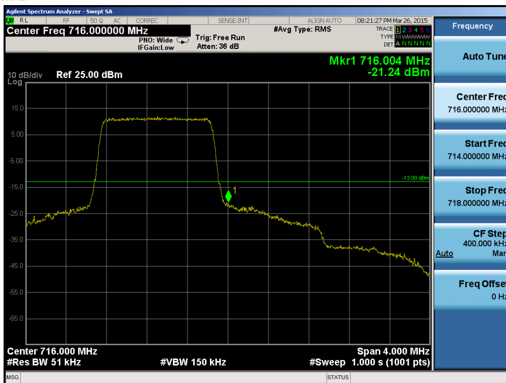
Plot 6-97. Upper Band Edge Plot (Band 12 – 1.4MHz QPSK – RB Size 6)
