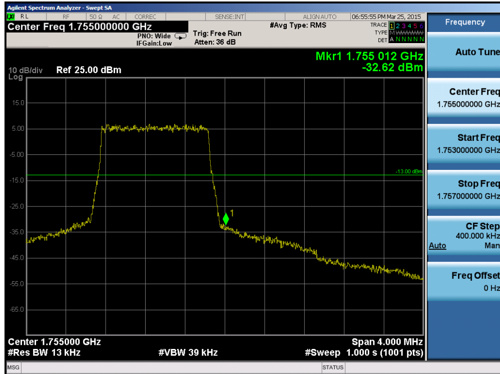
Plot 6-125. Upper Band Edge Plot (Band 4 – 1.4MHz QPSK – RB Size 6)
