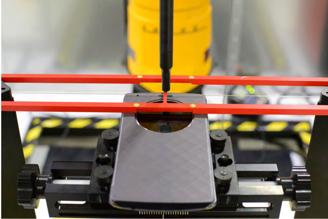
Figure 17-3 Ear Reference Point HAC Phantom Alignment (Wireless Charging Cover - Closed)
