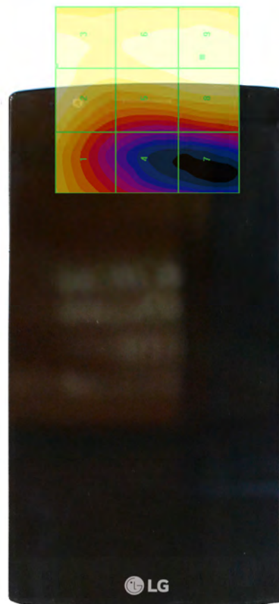
Figure 17-8 E-Field WD Scan overlay
