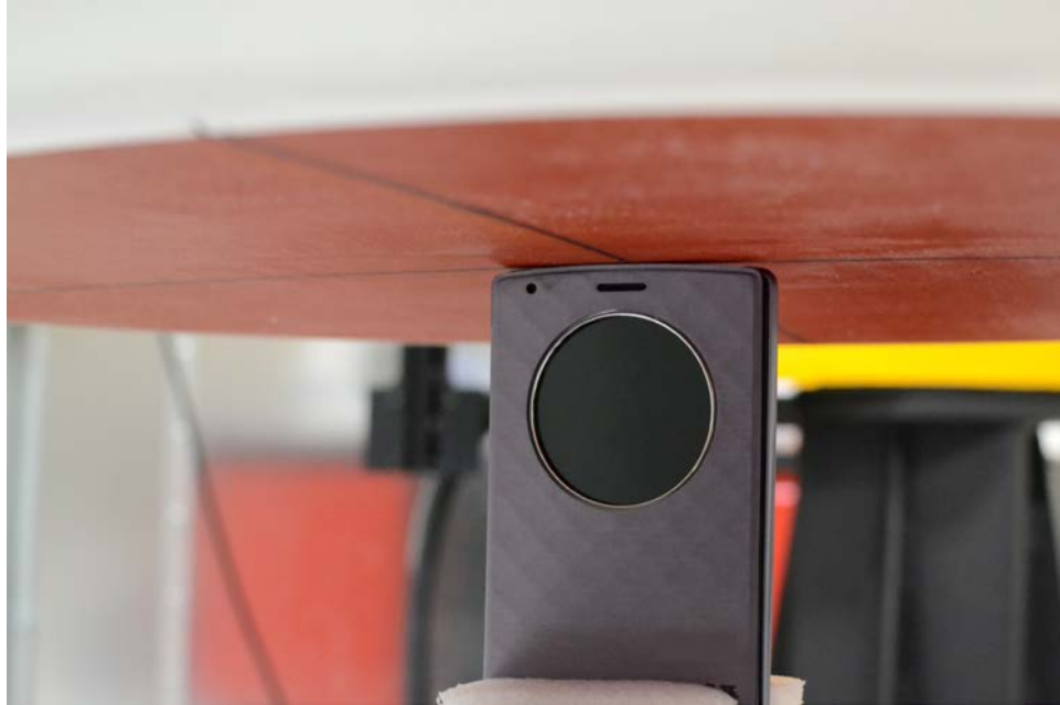
SAR Test Setup Photo 25: Top Edge, Quick Cover (Closed) at 0 mm
