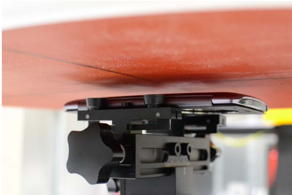
SAR Test Setup Photo 14: Back Side, Quick Cover (Closed) at 10 mm
