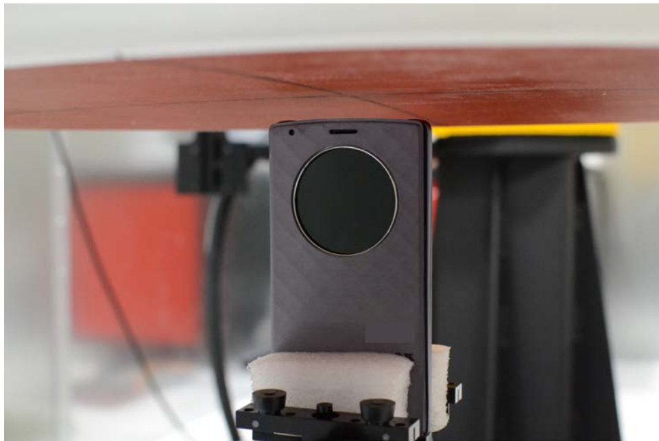
SAR Test Setup Photo 22: Top Edge, Quick Cover (Closed) at 10 mm
