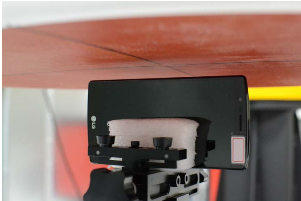
SAR Test Setup Photo 30: Left Edge, Standard Cover at 10 mm
