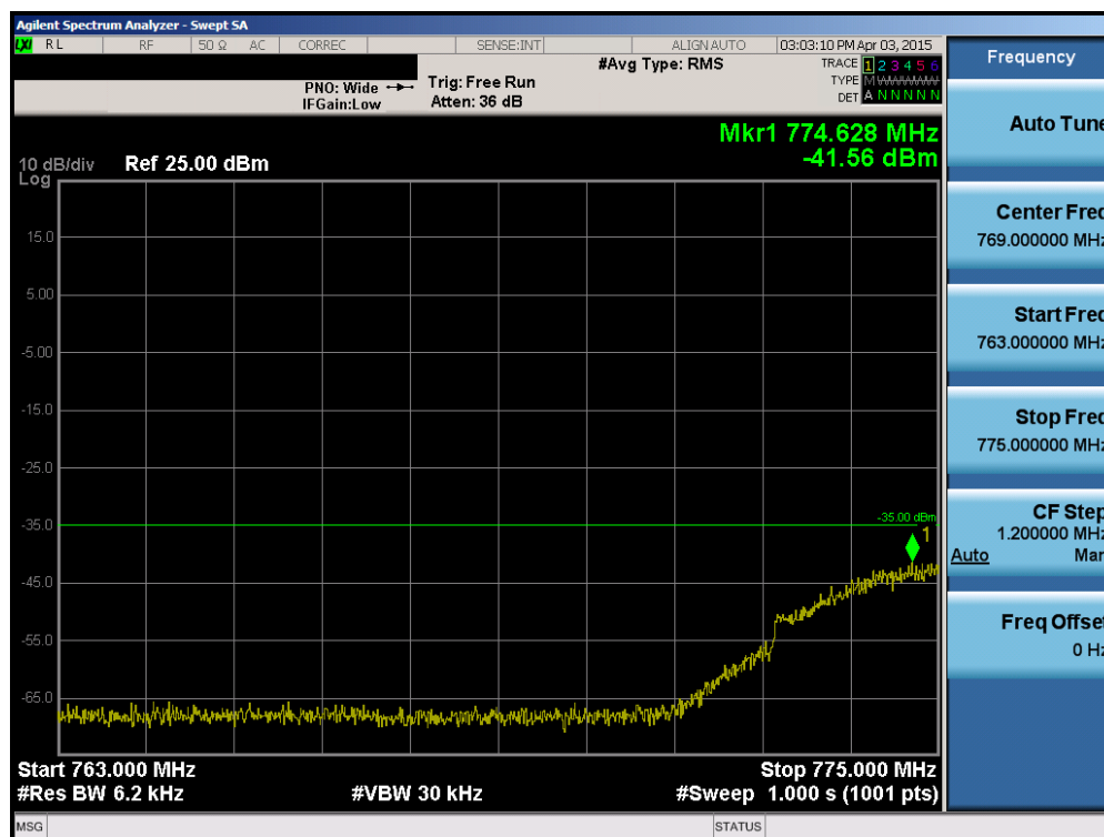
Plot 6-123. Lower Emission Mask Edge Plot (Band 13 – 5.0MHz QPSK – RB Size 25)
