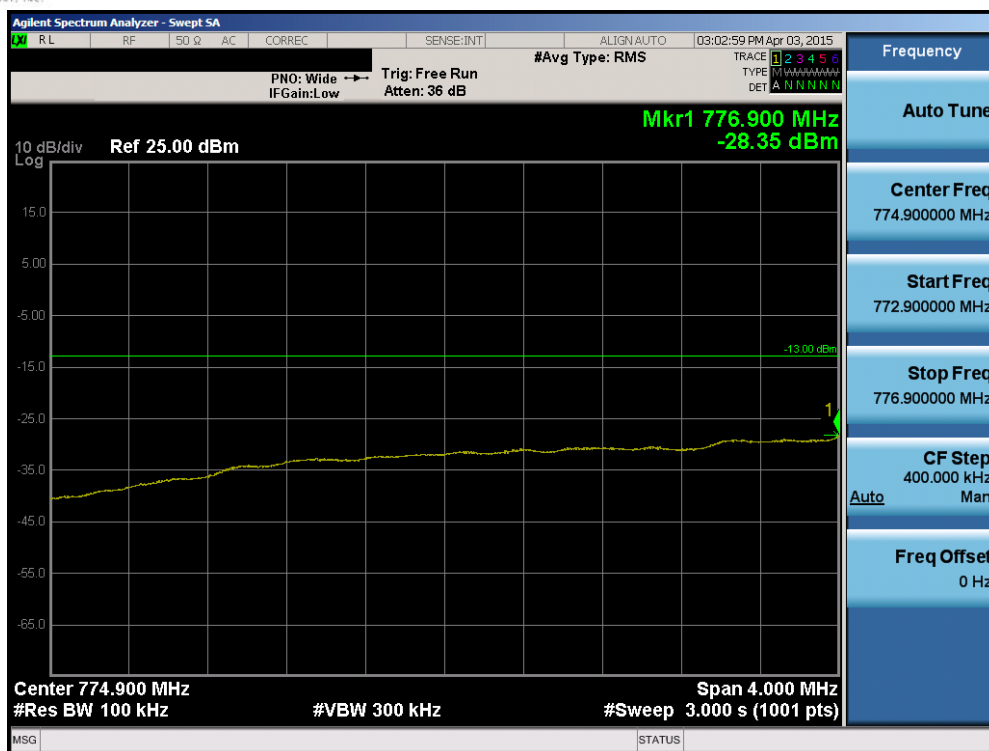
Plot 6-122. Lower Extended Band Edge Plot (Band 13 – 5.0MHz QPSK – RB Size 25)
