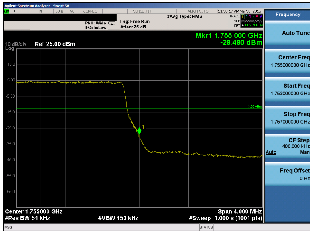
Plot 6-157. Upper Band Edge Plot (Band 4 – 5.0MHz QPSK – RB Size 25)
