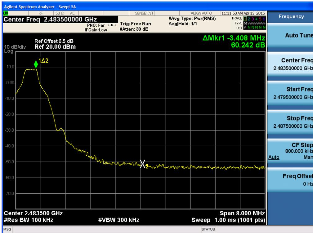
Test Plots with hopping (8DPSK)
