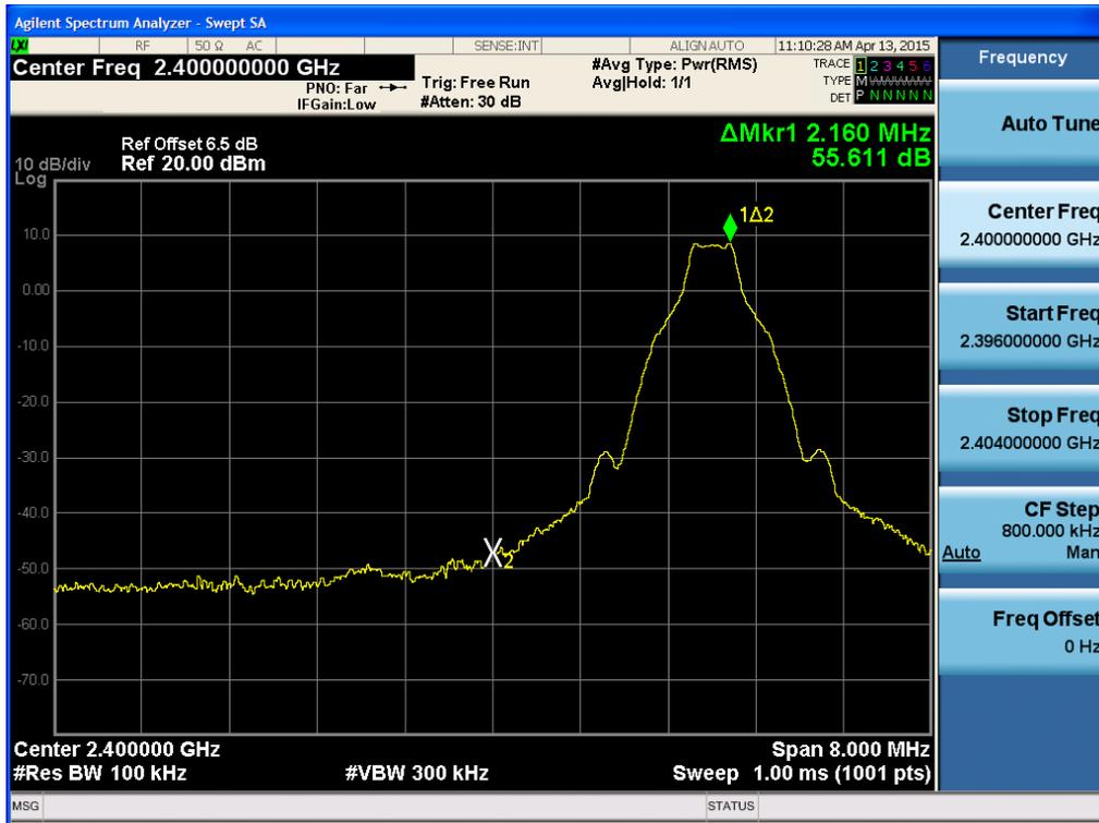
Test Plots with hopping (GFSK)
