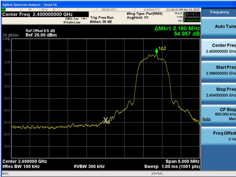
Test Plots with hopping (8DPSK)
