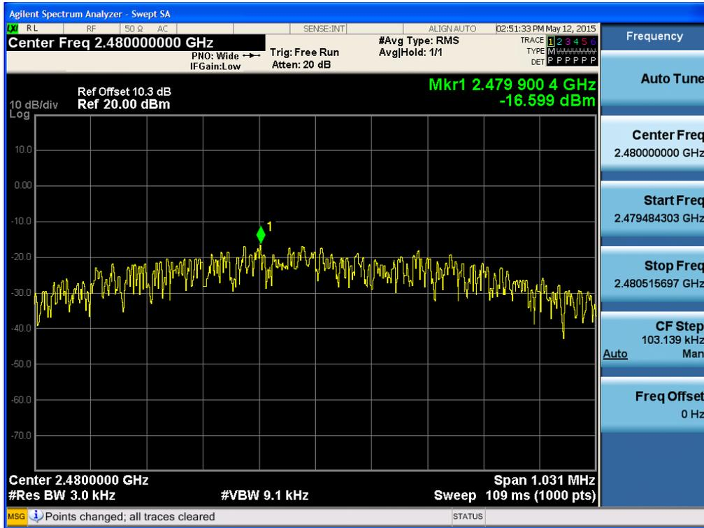
**8.5 OUT OF BAND EMISSIONS AT THE BAND EDGE/ CONDUCTED SPURIOUS EMISSIONS****Test Requirements and limit, §15.247(d)**
