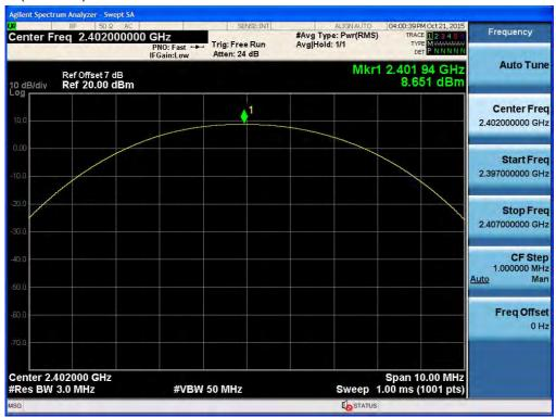
Test Plots (GFSK) Peak Power (Mid-CH)
