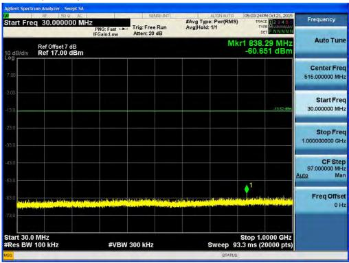
Test Plots (8DPSK)- 1 GHz - 3 GHz Spurious Emission (Mid-CH)
