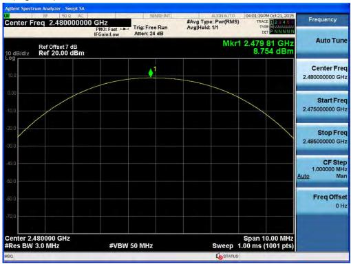
Test Plots (8DPSK) Peak Power (Low-CH)
