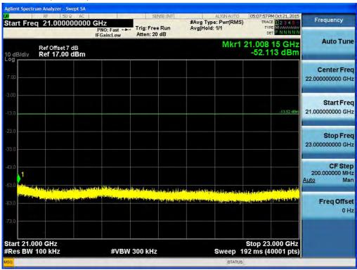
Test Plots (8DPSK)- 21 GHz - 23 GHz Spurious Emission (Mid-CH)
