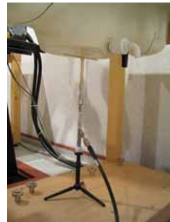
Photo of the dipole Antenna
