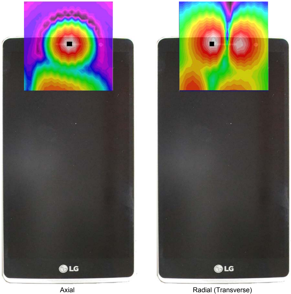
Axial Radial (Transverse) Figure 12-3 T-Coil Scan Overlay Magnetic Field Distributions
