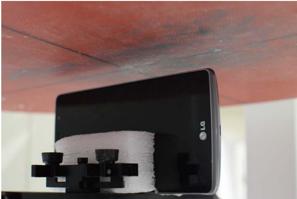
SAR Test Setup Photo 12 – Right Edge at 1.0 cm
