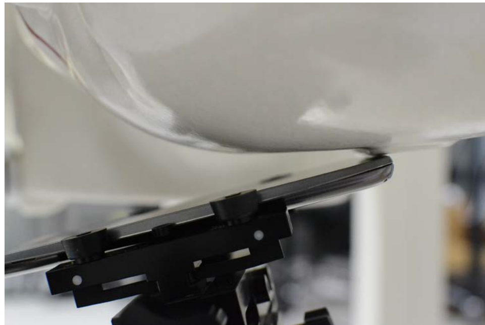
SAR Test Setup Photo 4 – Left Tilt
