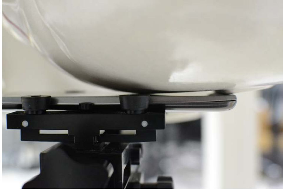
SAR Test Setup Photo 3 – Left Cheek
