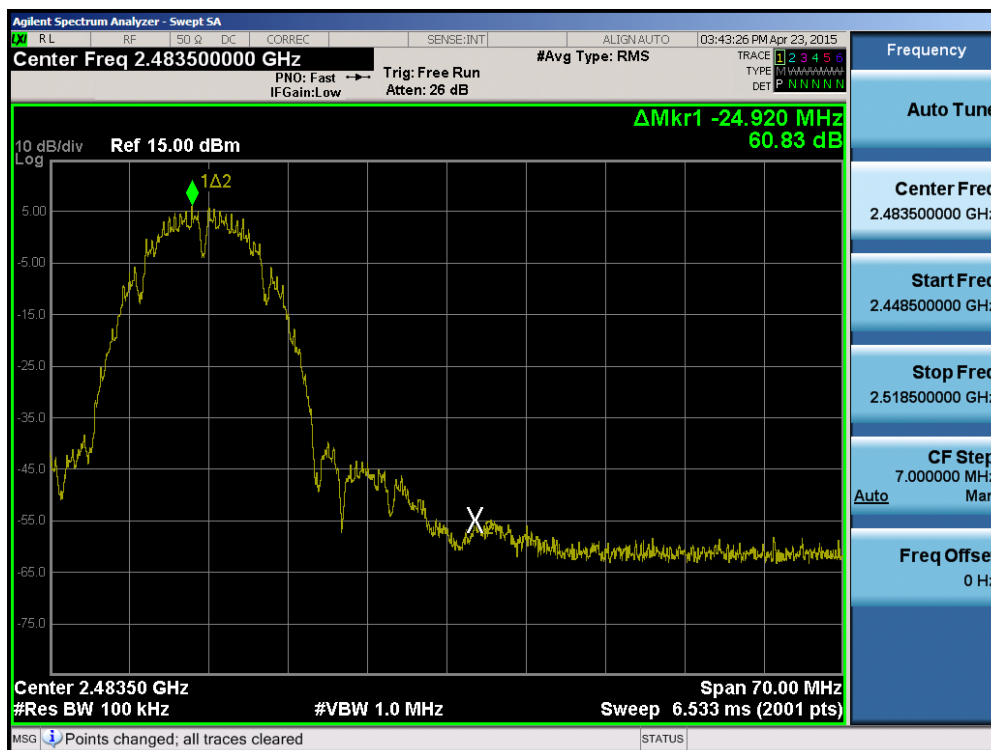
Plot 6-22. Band Edge Plot (802.11g - Ch. 11)
