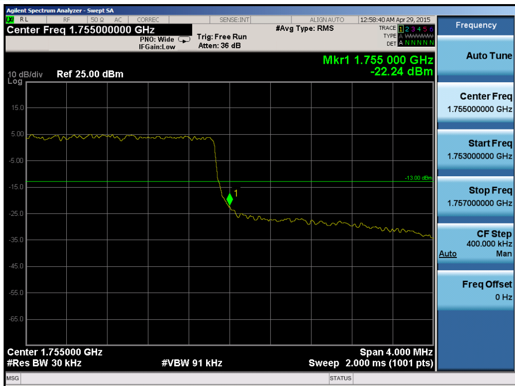
Plot 6-101. Upper Band Edge Plot (Band 4 – 3.0MHz QPSK – RB Size 15)
