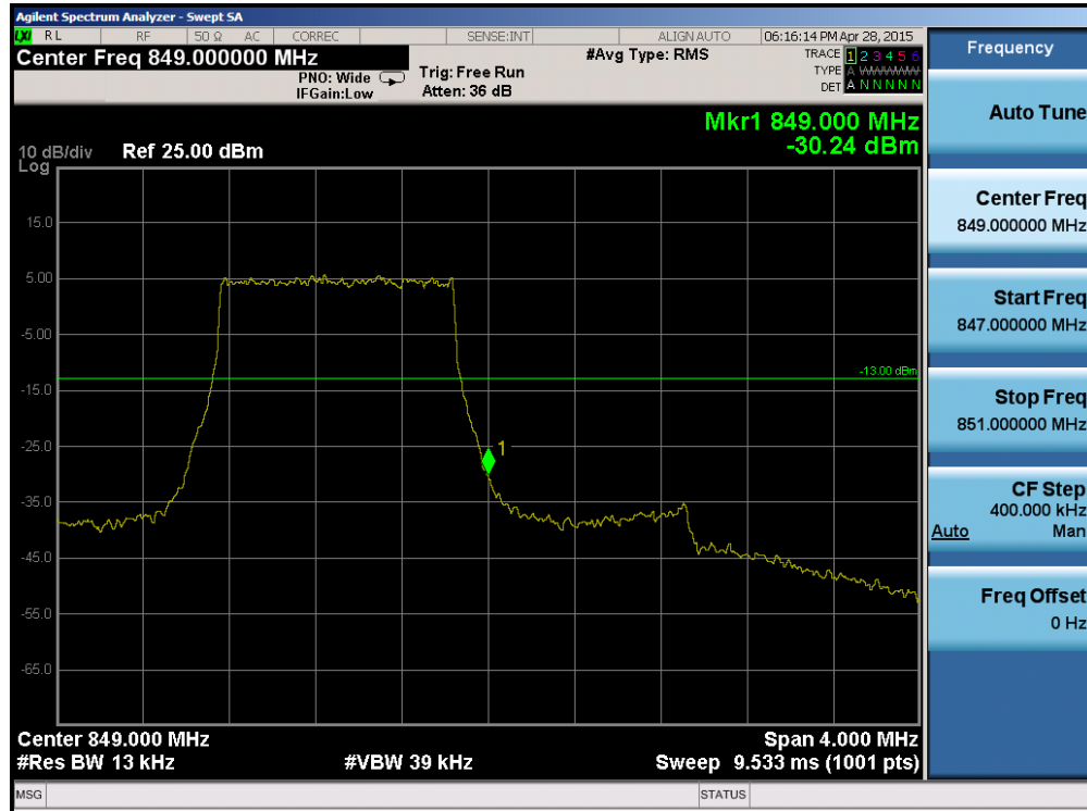
Plot 6-83. Upper Band Edge Plot (Band 5 – 1.4MHz QPSK – RB Size 6)
