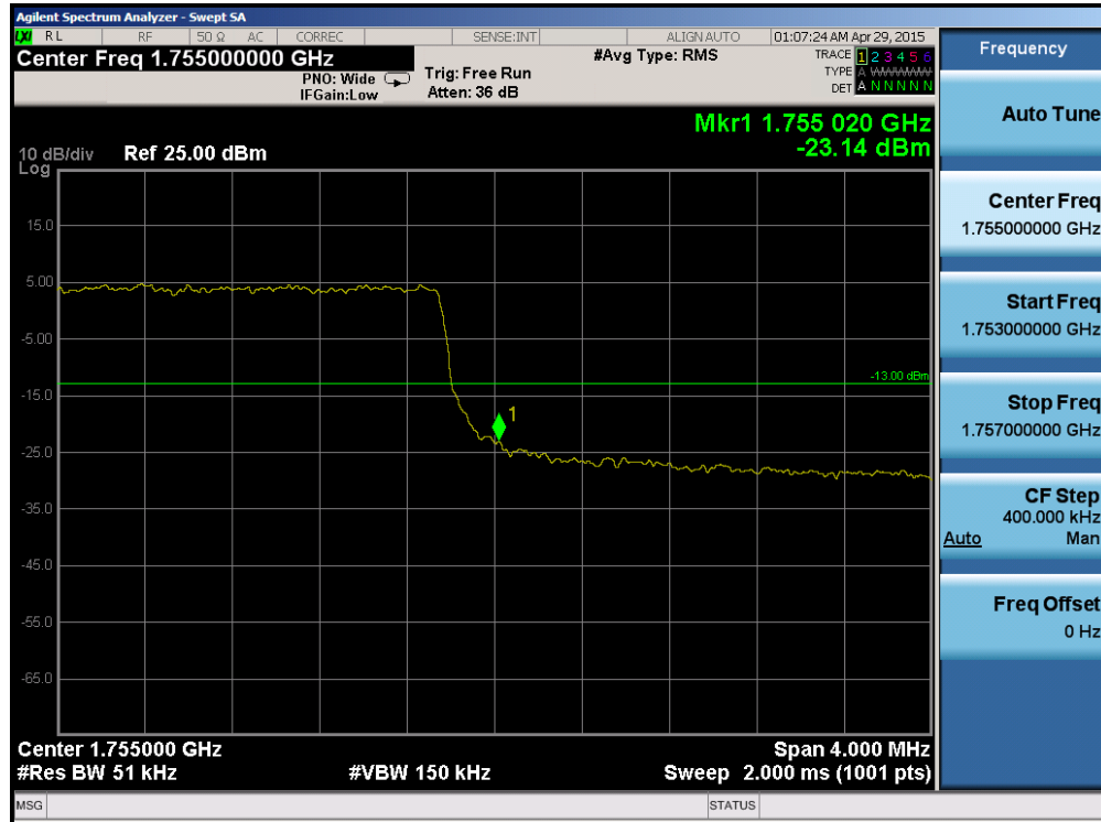
Plot 6-105. Upper Band Edge Plot (Band 4 – 5.0MHz QPSK – RB Size 25)
