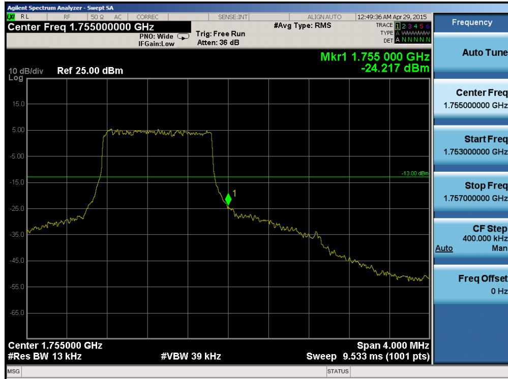
Plot 6-97. Upper Band Edge Plot (Band 4 – 1.4MHz QPSK – RB Size 6)
