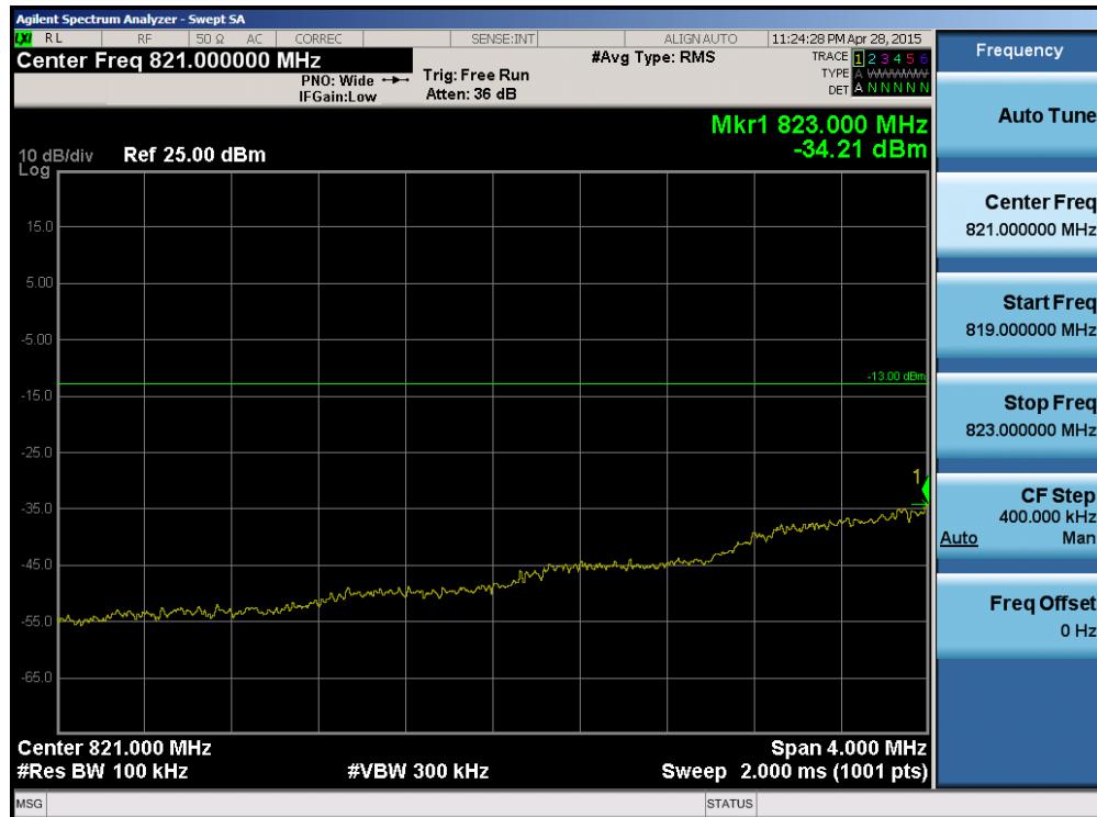
Plot 6-82. Lower Extended Band Edge Plot (Band 5 - 1.4MHz QPSK - RB Size 6)
