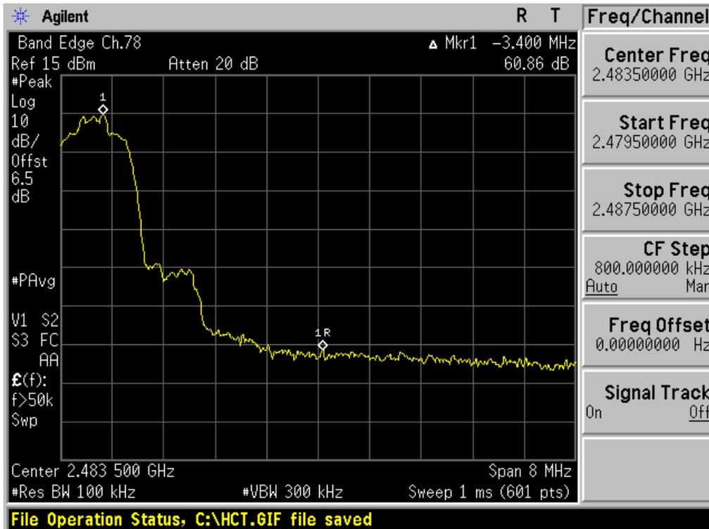
Test Plots with hopping (GFSK)
