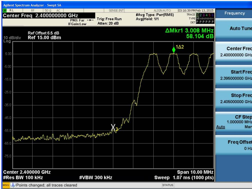
Test Plots with hopping (GFSK)
