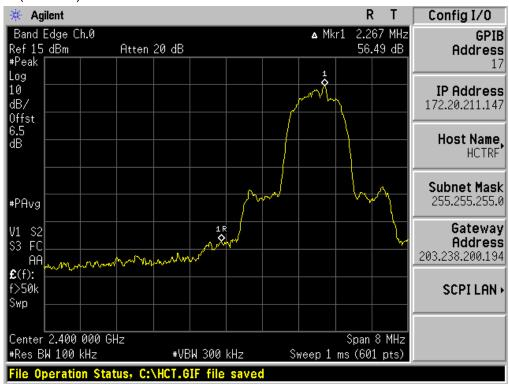
Test Plots without hopping (8DPSK) Band Edges (High-CH)
