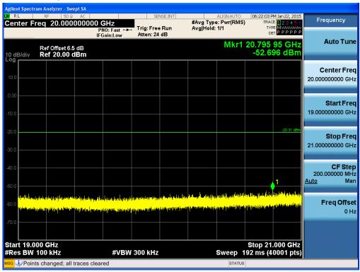
Test Plots (8DPSK)- 21 GHz - 23 GHz Spurious Emission (High-CH)
