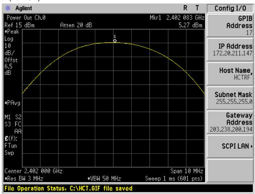
Test Plots (π/4DQPSK) Peak Power (Mid-CH)
