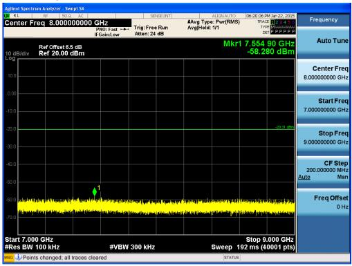
Test Plots (8DPSK)- 9 GHz - 11 GHz Spurious Emission(High-CH)
