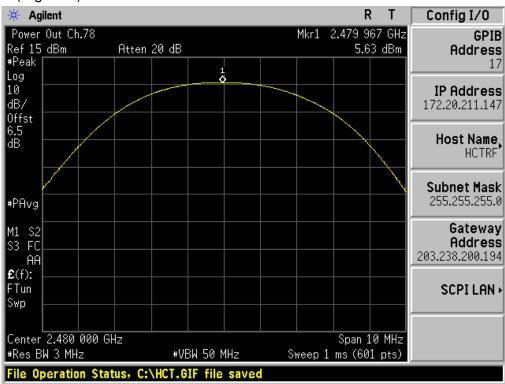
Test Plots (8DPSK) Peak Power (Low-CH)
