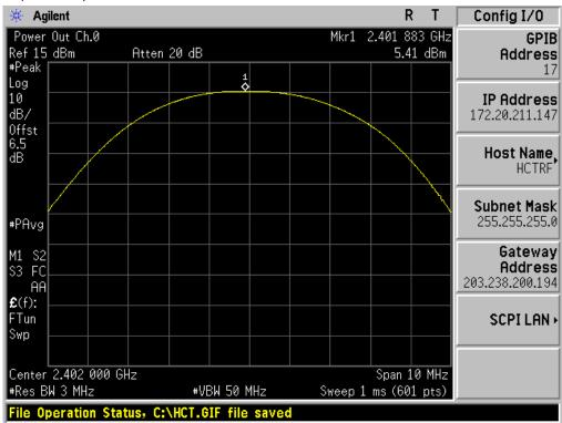
Test Plots (GFSK) Peak Power (Mid-CH)
