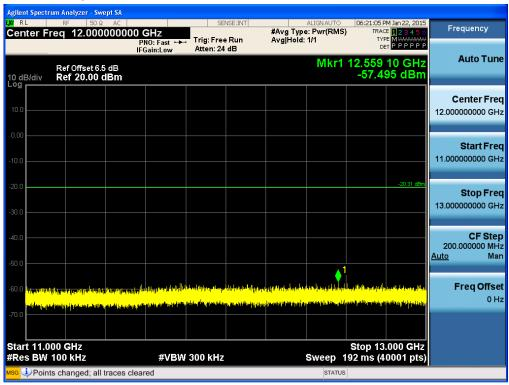
Test Plots (8DPSK)- 13 GHz - 15 GHz Spurious Emission (High-CH)
