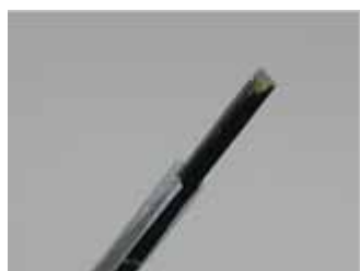
Figure 6. EX3DV4 E-field Probe
