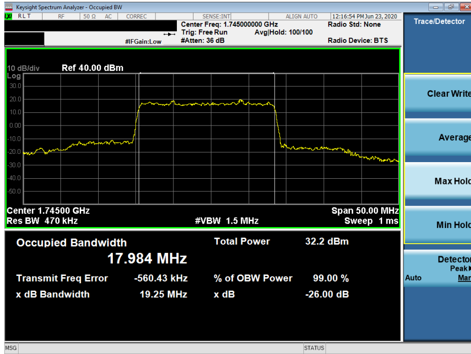
Plot 7-37. Occupied Bandwidth Plot (NR Band n66 - 20.0MHz DFT-s-OFDM BPSK - Full RB)
