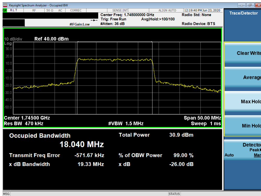
Plot 7-40. Occupied Bandwidth Plot (NR Band n66 - 20.0MHz CP-OFDM 64QAM - Full RB)
