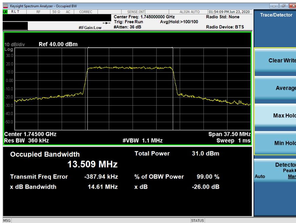
Plot 7-44. Occupied Bandwidth Plot (NR Band n66 - 15.0MHz CP-OFDM 16QAM - Full RB)
