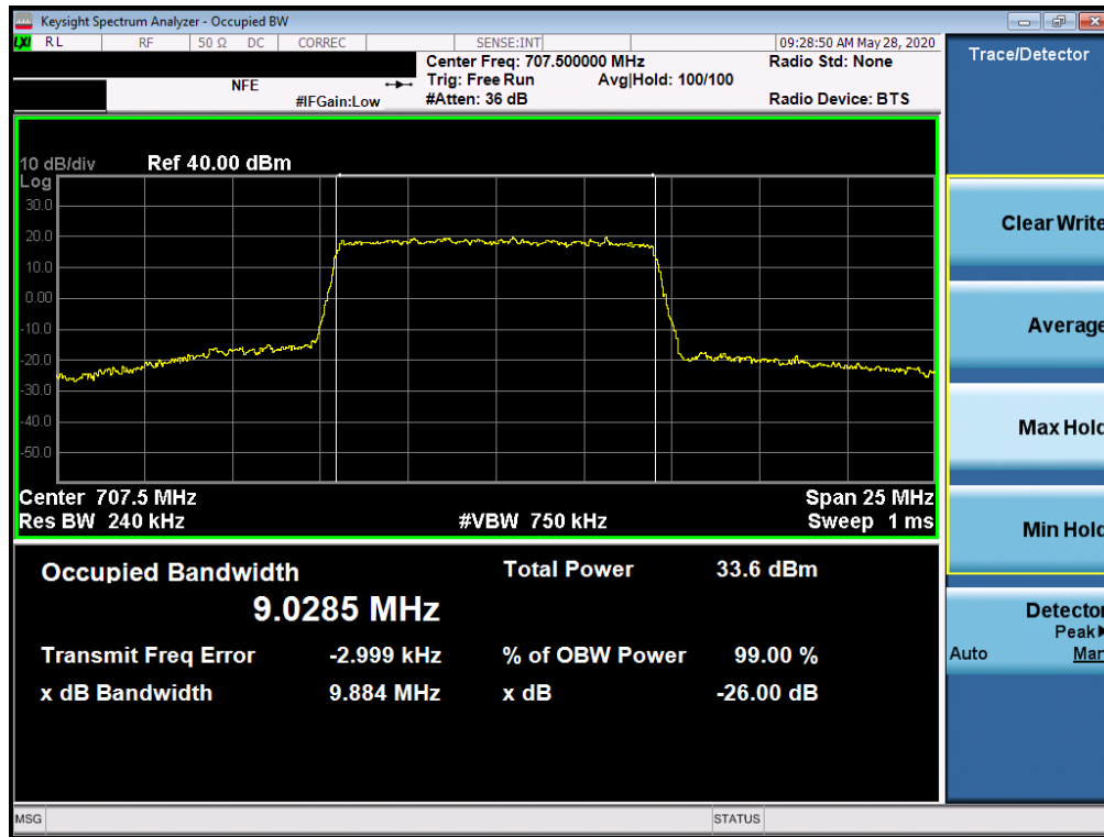
Plot 7-19. Occupied Bandwidth Plot (LTE Band 12 - 10MHz QPSK - Full RB Configuration)
