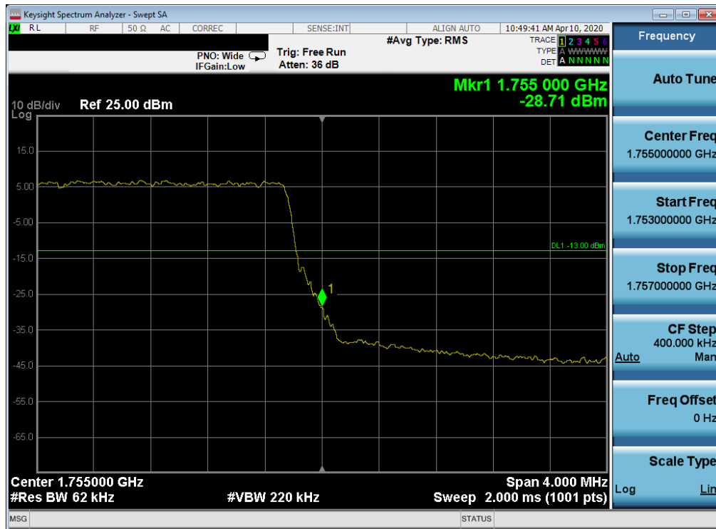
Plot 7-107. Upper Band Edge Plot (LTE Band 4 - 5MHz QPSK – Full RB Configuration)
