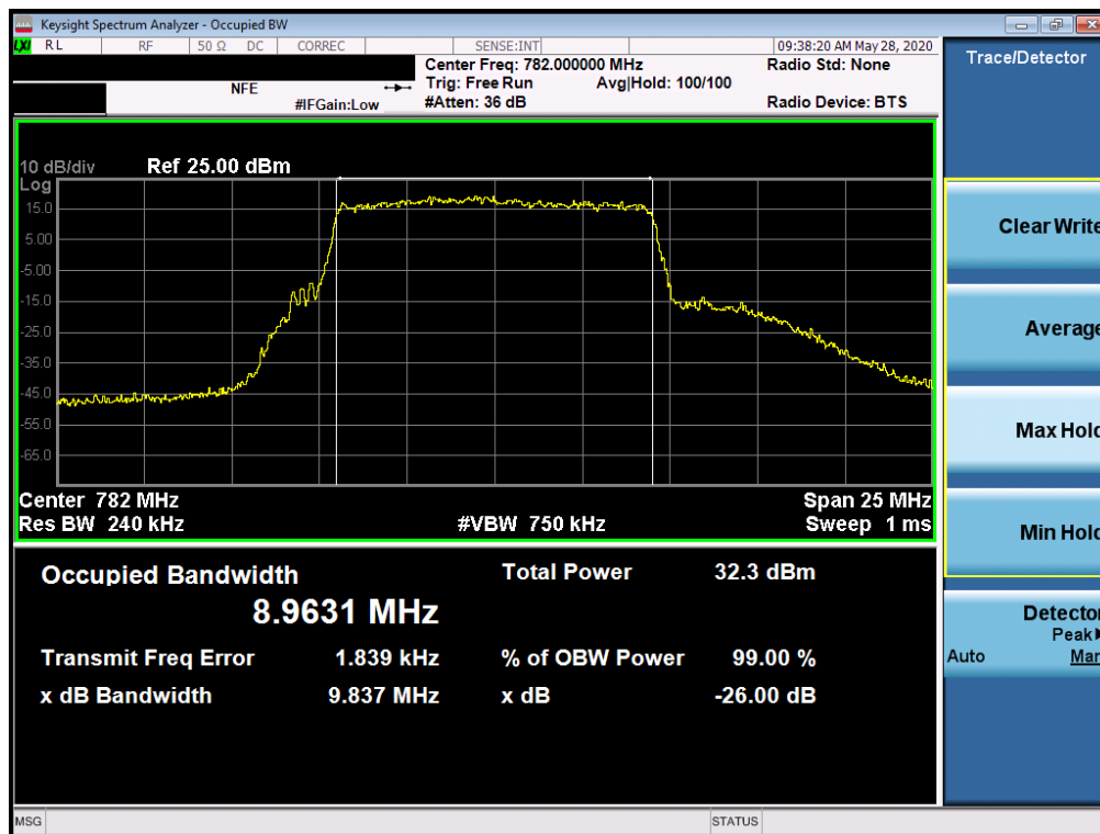
Plot 7-32. Occupied Bandwidth Plot (LTE Band 13 - 10MHz 16-QAM - Full RB Configuration)
