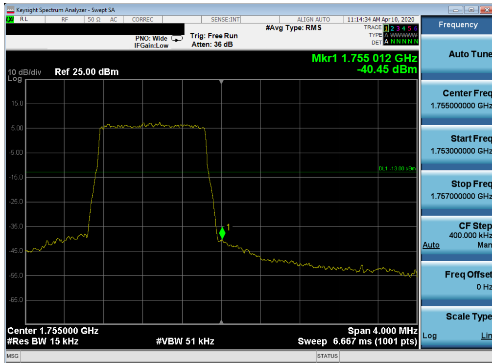
Plot 7-119. Upper Band Edge Plot (LTE Band 4 – 1.4MHz QPSK – Full RB Configuration)
