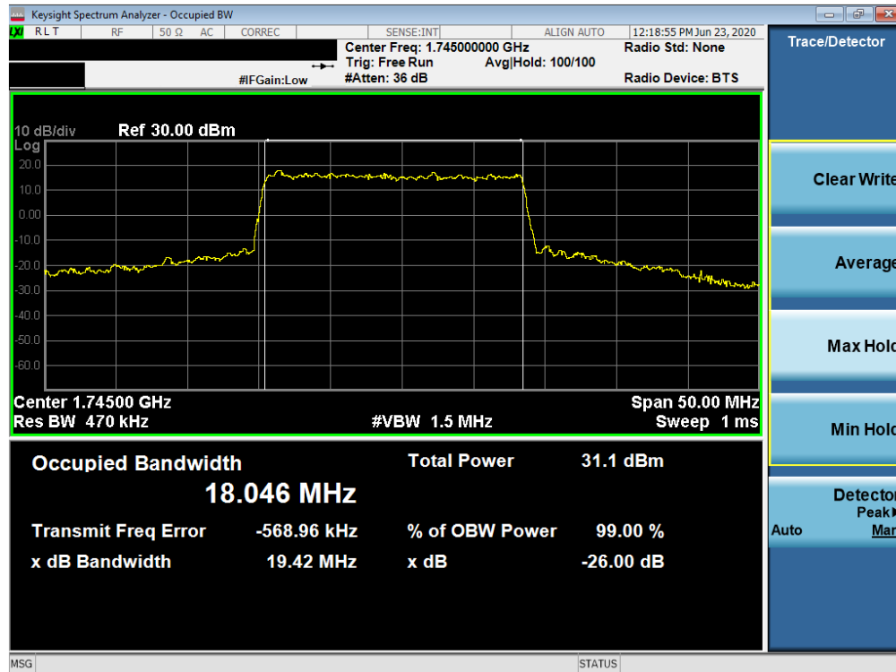
Plot 7-39. Occupied Bandwidth Plot (NR Band n66 - 20.0MHz CP-OFDM 16QAM - Full RB)
