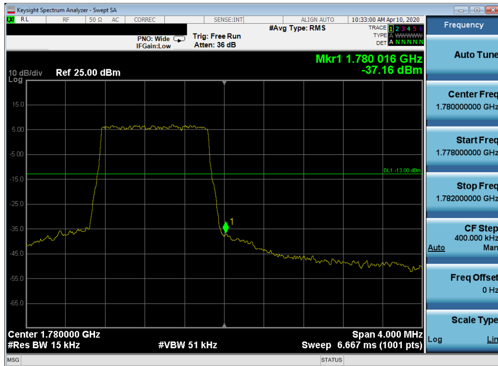
Plot 7-121. Upper Band Edge Plot (LTE Band 66 – 1.4MHz QPSK – Full RB Configuration)
