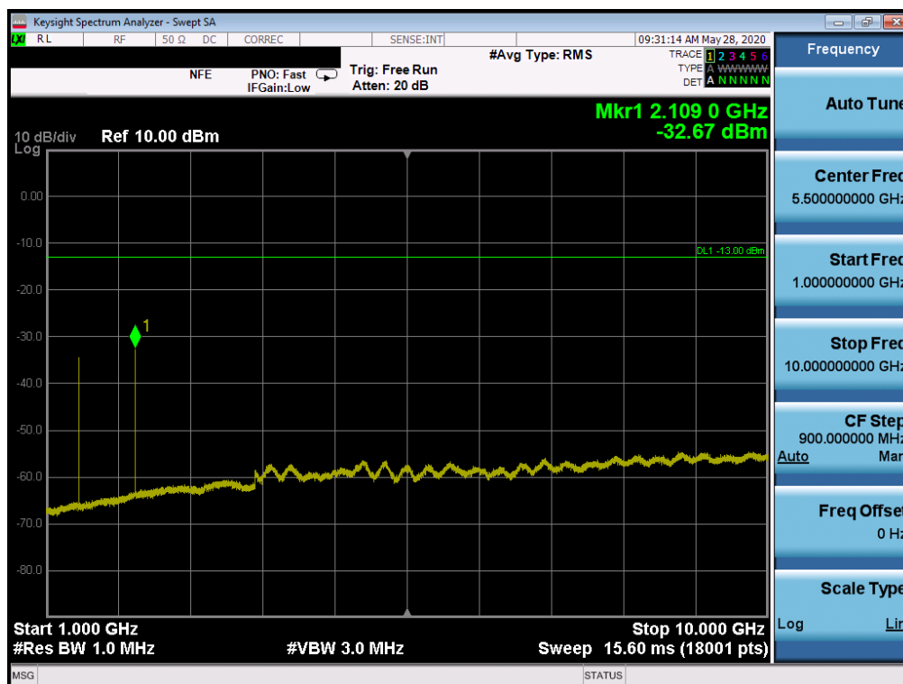
Plot 7-71. Conducted Spurious Plot (LTE Band 12 - 10MHz QPSK - RB Size 1, RB Offset 0 - Mid Channel)
