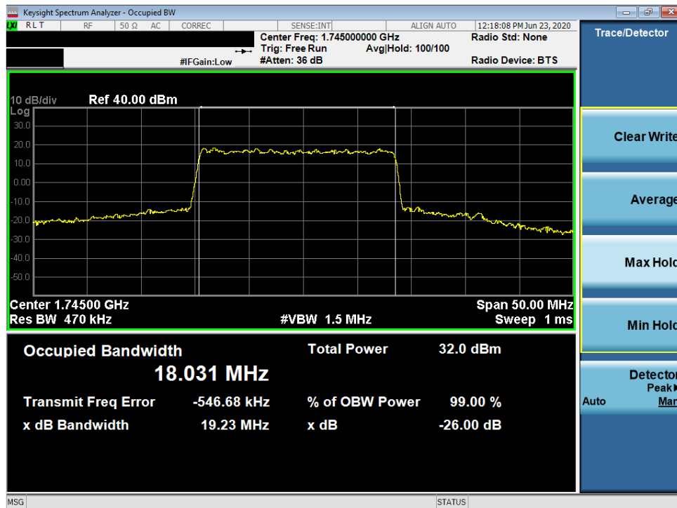
Plot 7-38. Occupied Bandwidth Plot (NR Band n66 - 20.0MHz CP-OFDM QPSK - Full RB)
